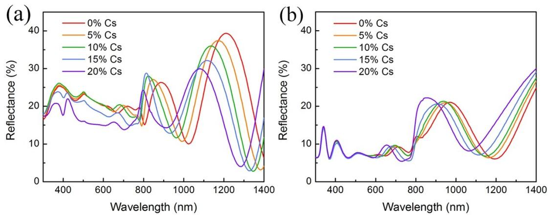
**Fig. S4.** The reflectance spectra from (a) film side and (b) glass side of perovskite films fabricated on FTO substrates with different amount of Cs.
