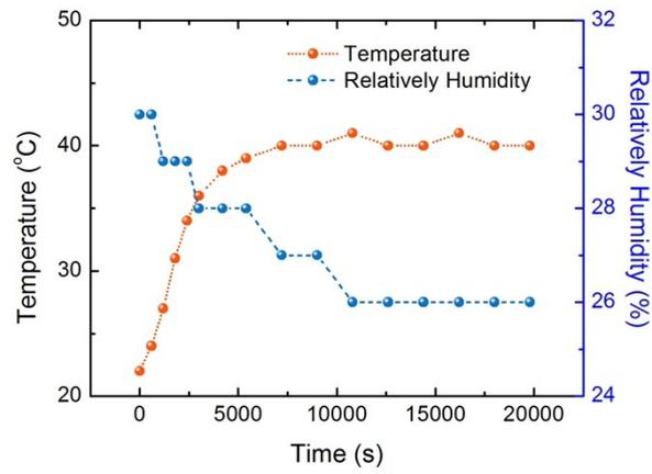
**Fig. S9.** The evolution of surface temperature of the device and relatively humidity of the atmosphere during the MPPT measurement of one PVSC.
