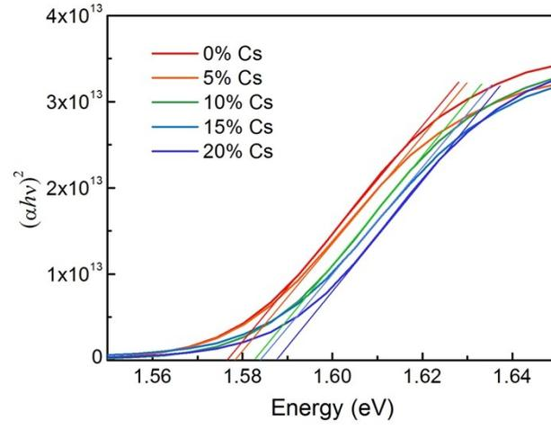
**Fig. S2.** Tacu plots derived from absorbance spectra of perovskite films with different Cs concentrations.
