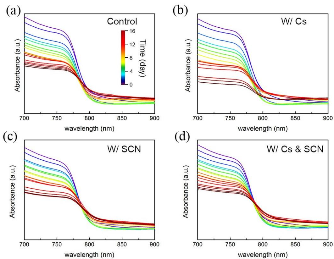
**Fig. S11.** Absorbance spectra of perovskite films exposed in ~60% relatively humidity air for different days.
