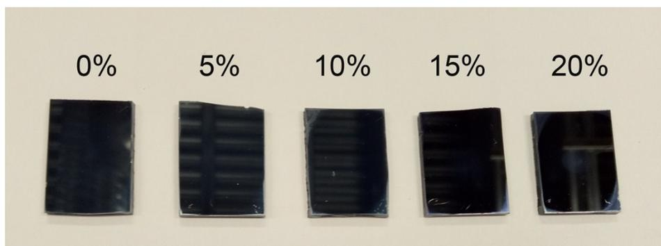
**Fig. S3.** Photos of perovskite films with different Cs concentrations.
