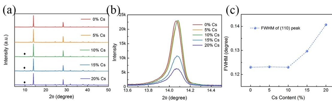
**Fig. S5.** (a) XRD patterns and (b) enlarged (110) peak of perovskite films fabricated on FTO substrates with different amount of Cs. (c) Full width half maximum (FWHM) of the (110) peak calculated from (b).
