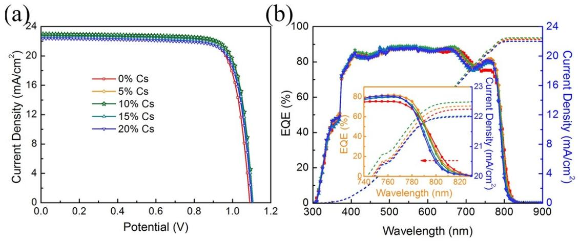
**Fig. S7.** (a)  $J-V$  curves measured under reverse voltage scans and (b) EQE plots of PVSCs with SCN and different contents of Cs. Inset shows that the onset of EQE gradually blue-shifted while increasing the ratio of Cs.
