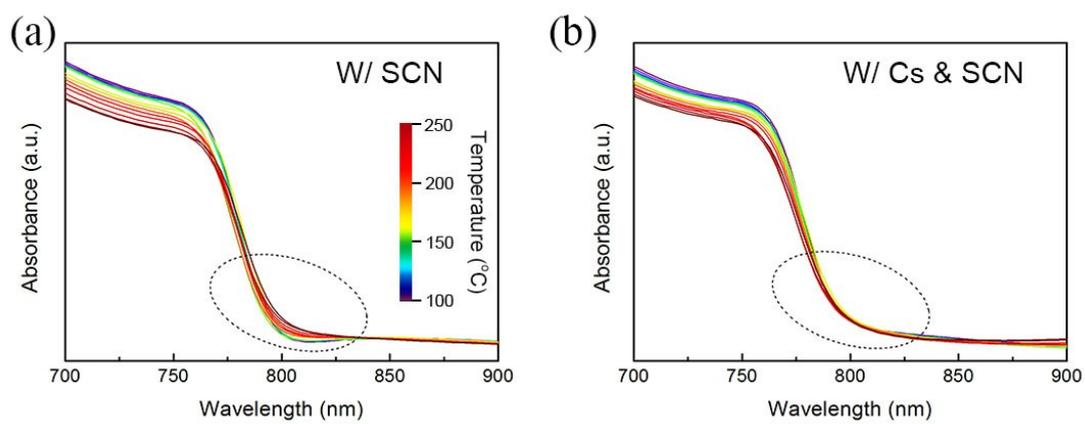
**Fig. S10.** Absorbance spectra of perovskite films W/ SCN and W/ Cs & SCN heated at different temperatures for 1 minute at each. The temperature changes from 100 to 250 °C.
