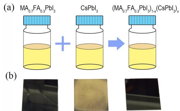
**Fig. S1.** (a) Scheme of the mixture of  $(\text{MA}_{0.7}\text{FA}_{0.3}\text{PbI}_3)_{1-x}(\text{CsPbI}_3)_x$  precursor. (b) Perovskite films fabricated at 100 °C in a glovebox and then been brought out for taken picture. From left to right,  $x=0$ ,  $x=1$  and  $x=0.1$ , respectively.
