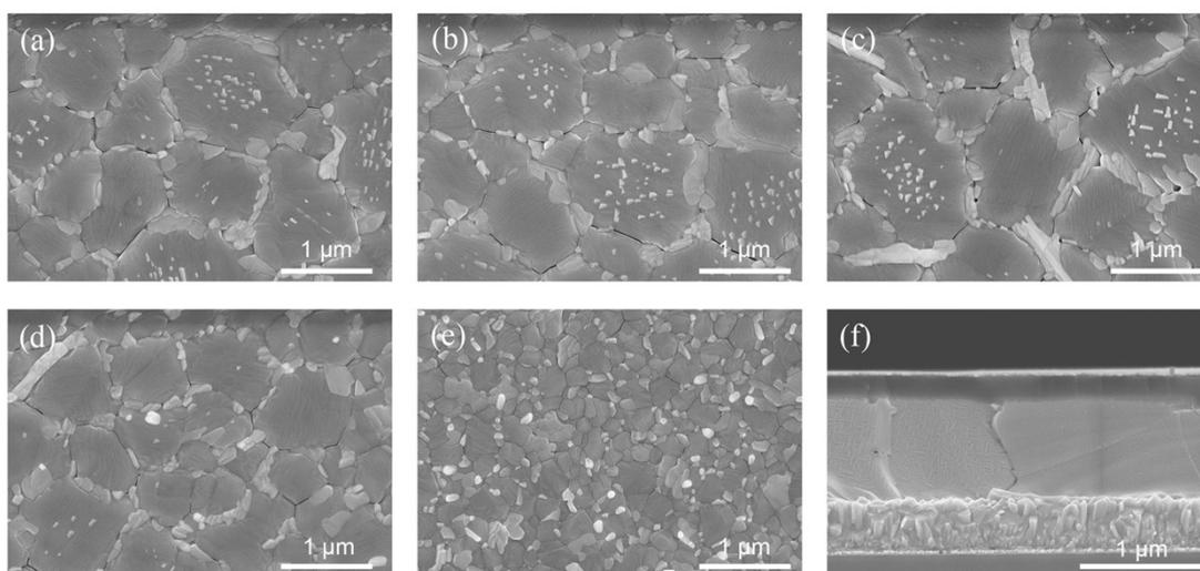
**Fig. S6.** Top-view of SEM images of SCN-incorporated  $(\text{MA}_{0.7}\text{FA}_{0.3})_{1-x}\text{Cs}_x\text{PbI}_3$  films with the concentration of Cs varying from 0 to 20%. (a) 0%, (b) 5%, (c) 10%, (d) 15%, (e) 20%. (f) Cross-sectional SEM of 10% Cs incorporated perovskite device.
