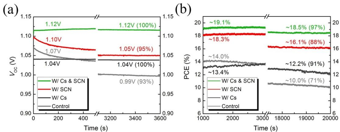
**Fig. S8.** The (a)  $V_{OC}$  tracking and (b) maximum power point tracking of PVSCs of pure  $MA_{0.7}FA_{0.3}PbI_3$  (control), incorporated with only Cs (W/ Cs), incorporated with only  $Pb(SCN)_2$  (W/ SCN) and with both (W/ Cs & SCN).
