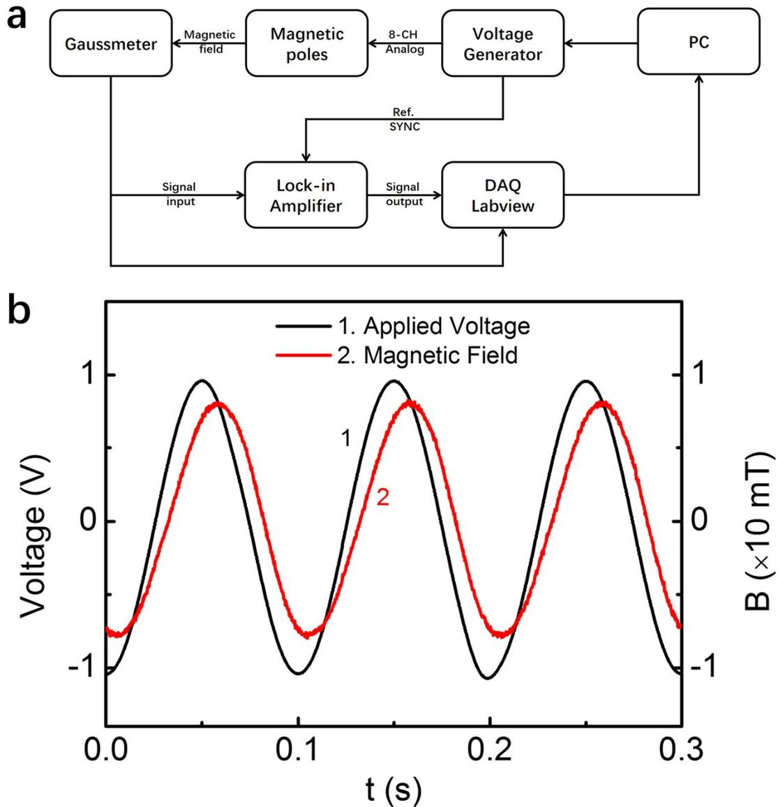
**Fig. S3. (a) Schematic to measure amplitude decay and phase delay of the magnetic field. (b) Time dependence of the applied voltage and the corresponding magnetic field (B). An AC voltage signal at frequency of 10 Hz is applied on the two sets of magnetic poles, where a Gaussmeter probe is placed in between with a distance of 0.5 mm from each set.**
