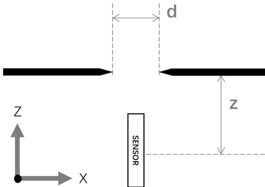
Fig. S4. Schematic of utilizing a Gaussmeter probe to access the distance dependence of the magnetic field from the magnetic poles ( $z$ ) and the size of the gap ( $d$ ) between them.
