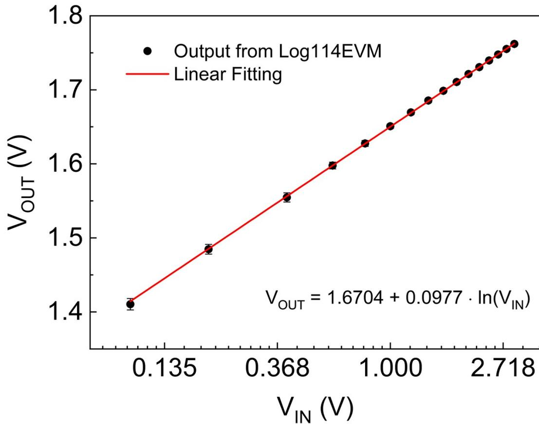
**Fig. S1. Linear relationship between output ( $V_{OUT}$ ) and input ( $V_{IN}$ ) for logarithmic amplifier. The impedance used in the LOG114 module is about  $0.5 M\Omega$ , the input voltage is generated by a function generator in a square-wave function.**
