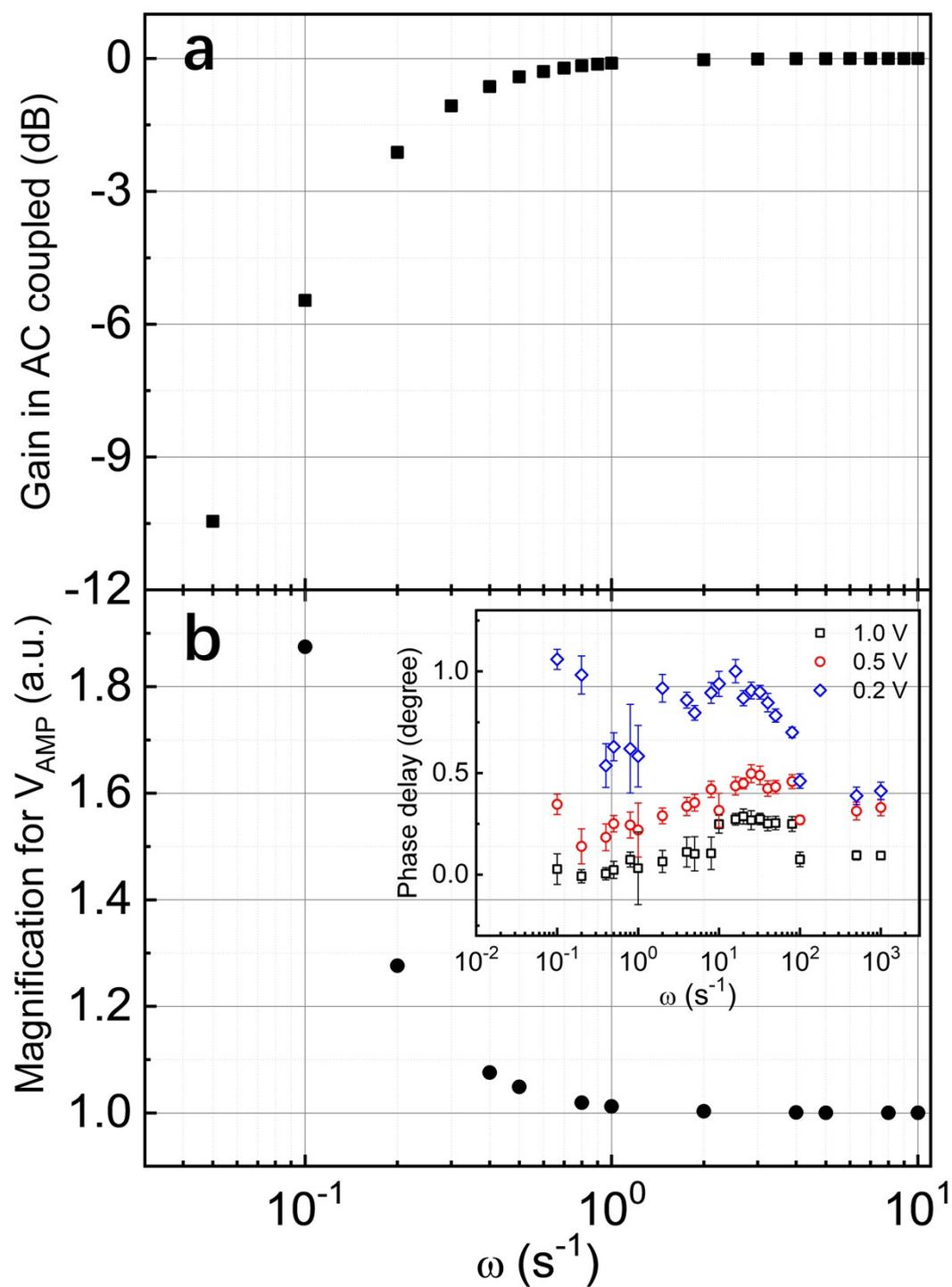
Fig. S2. Correction for amplitude and phase lag for the lock-in amplifier. (a)
