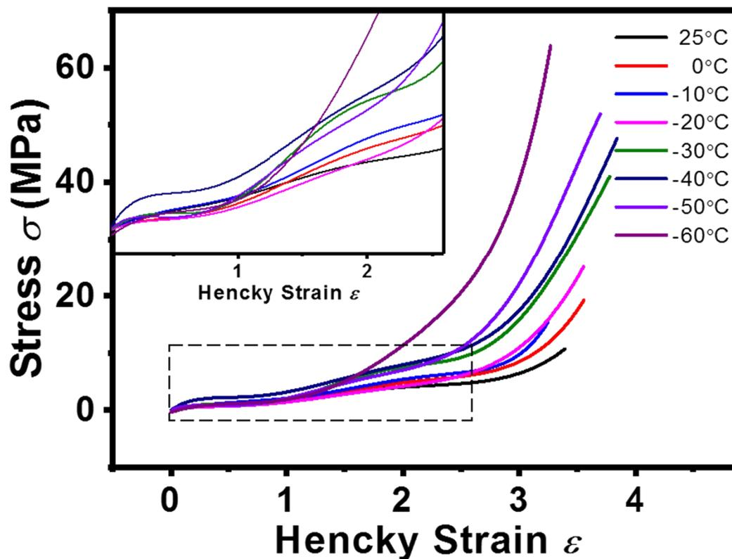
**Fig. S3** The stress-strain curves of NR at various temperatures (stress represents the engineering stress). Magnified **Fig. 4**.
