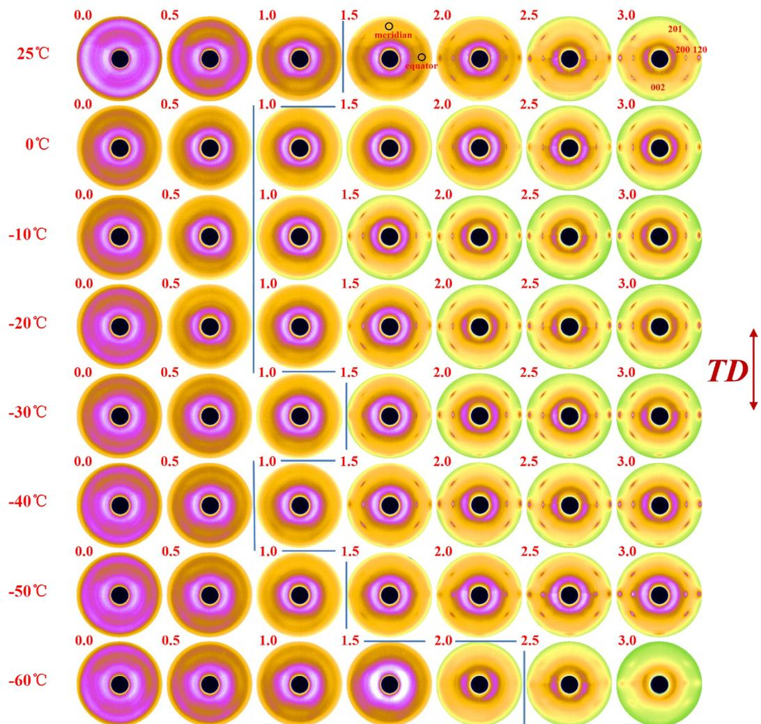
**Fig. S4** Sequential evolution of 2D SR-WAXD patterns during uniaxial stretching at different temperatures. The tensile direction is vertical as shown by the double arrow, and the corresponding Hencky strain values  $\epsilon$  are shown at the top left corner of each diffraction pattern. Magnified **Fig. 6**.
