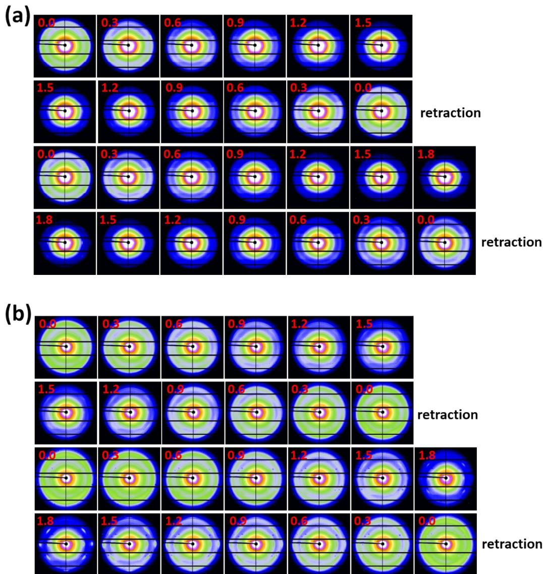
**Fig. S2** Sequential evolution of 2D SR-WAXD patterns during deformation-retraction at (a) 25 °C and (b) -40 °C. The tensile direction is vertical and the corresponding Hencky strain values  $\epsilon$  are shown at the top left corner of each diffraction pattern.
