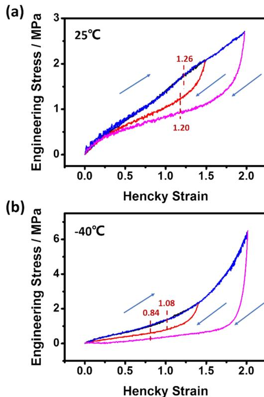
**Fig. S1** The stress-strain curves of NR at (a) 25 °C and (b) -40 °C.
