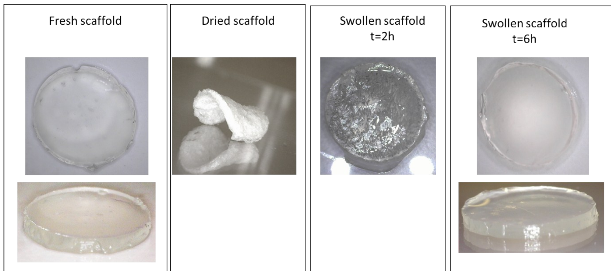
Figure 4 Macroscopic images showing the swelling process of the HM-10 scaffold from the dried sample and over 2h and 6h. The samples reached swelling equilibrium after 6h.
