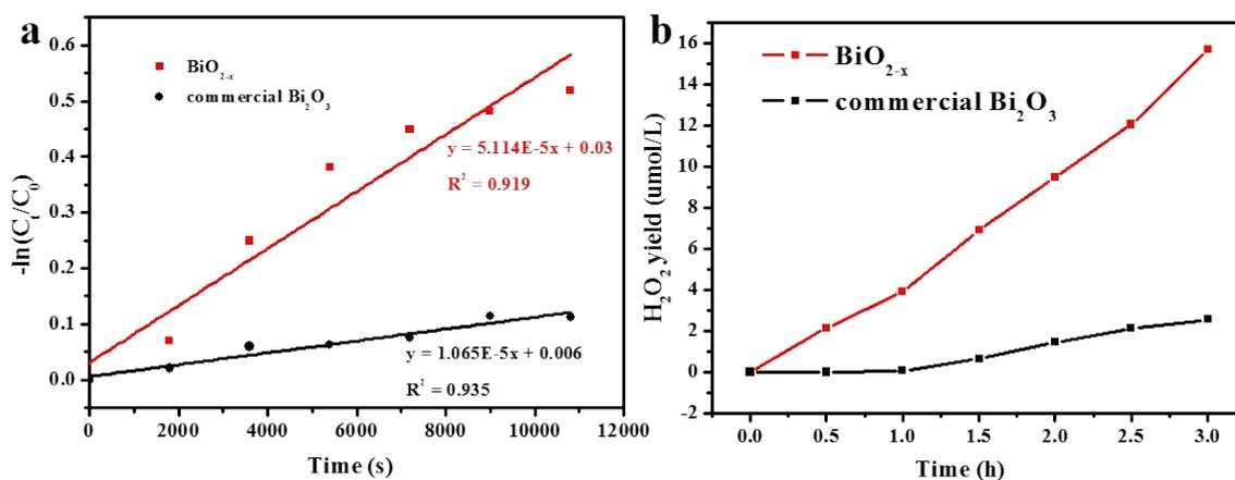
**Figure S8.** a) Pseudo-first-order reaction fitting curve of NBT concentration, and b) H<sub>2</sub>O<sub>2</sub> concentration in the presence of BiO<sub>2-x</sub> or Bi<sub>2</sub>O<sub>3</sub> under visible light irradiation.
