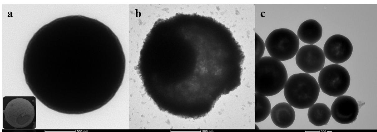
**Figure S5.** TEM images of  $\text{BiO}_{2-x}$  with (a) core-shell structure, b) yolk-shell structure, and c) complex hollow structures.
