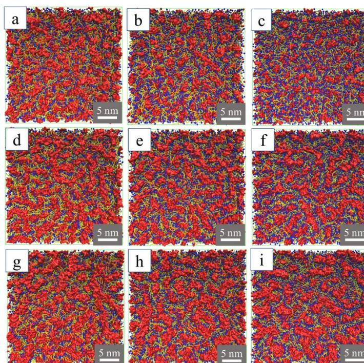
**Figure S4.** The collected snapshots of the computed results of (a) C6C6-X20Y30; (b) C6C6-X30Y20; (c) C6C6-X40Y10; (d) C10C6-X20Y30; (e) C10C6-X30Y20; (f) C10C6-X40Y10; (g) C16C6-X20Y30; (h) C16C6-X30Y20; (i) C16C6-X40Y10. Yellow represents PPO domains; Blue represents QA and OH domains; Red represents GC domains.
