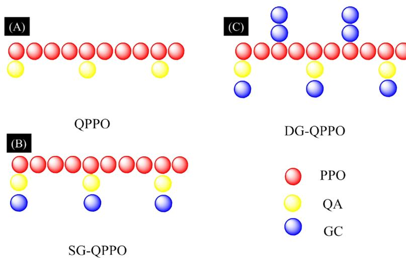
**Figure S2.** The models used for the calculated system (A) QPPO; (B) SG-QPPO; (C) DG-QPPO. Note that one PPO bead corresponds to one PPO monomer unit
