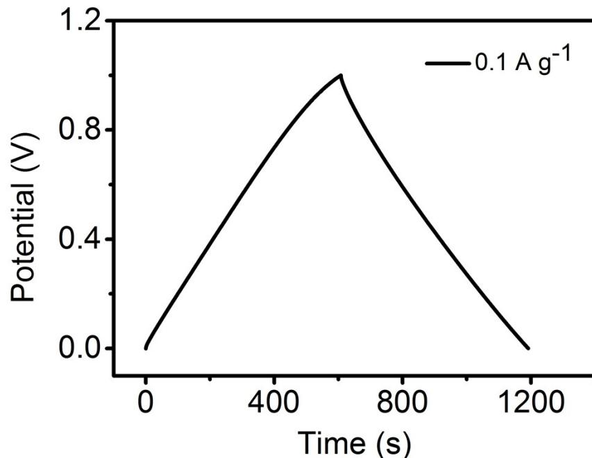
**Fig. S7** Galvanostatic charge-discharge curves of the solid-state supercapacitor at a current density of  $0.1 \text{ A g}^{-1}$
