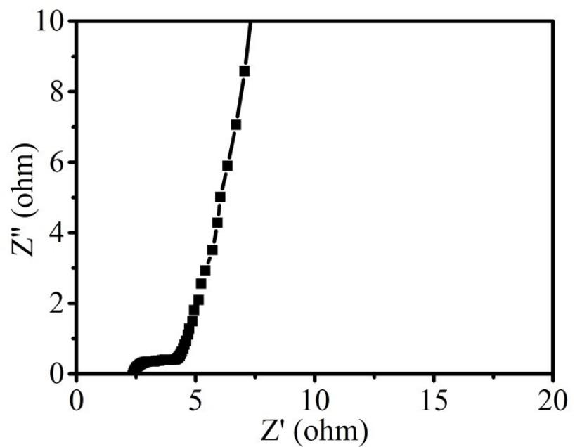
**Fig. S6** Nyquist plot of the solid-state supercapacitor with a-CNS/EG-10 electrode measured in PVA/KOH gel electrolyte.
