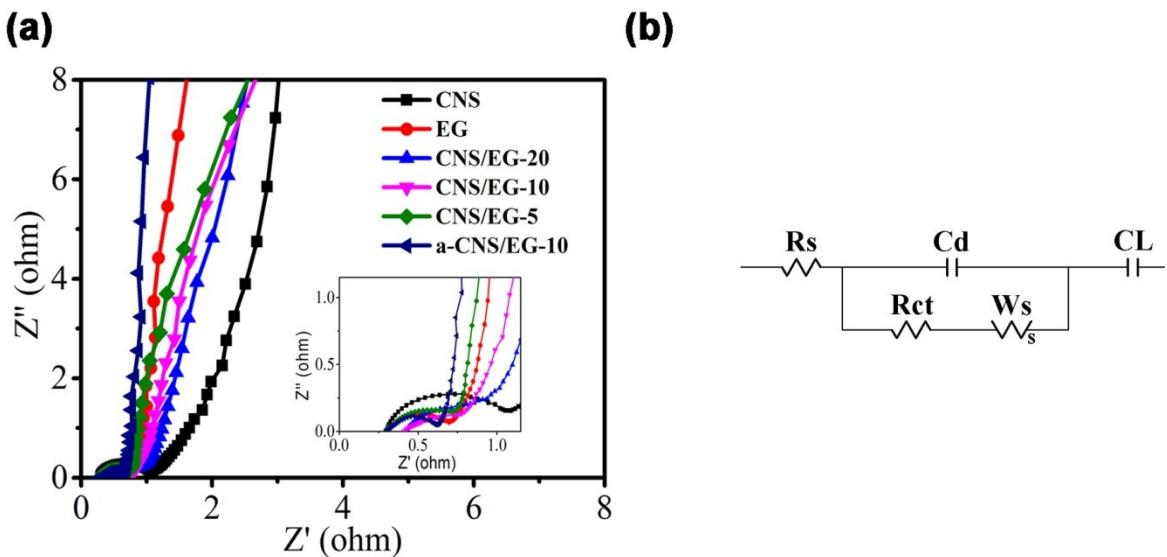
Fig. S5 (a) Nyquist plots of the CNS, EG, CNS/EG, and a-CNS/EG-10 samples measured in  $6 \text{ mol L}^{-1}$  KOH electrolyte using three-electrode systems (the inset shows the magnified high frequency range). (b) The equivalent circuit of EIS.
