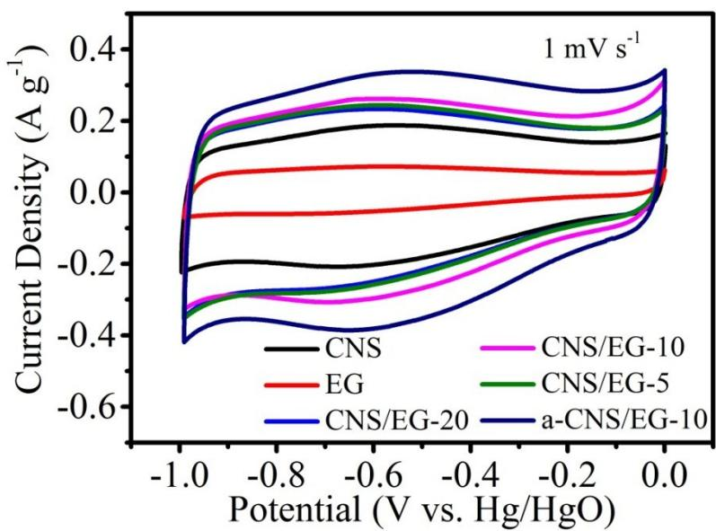
**Fig. S4** CV curves of the CNS, EG, CNS/EG, and a-CNS/EG-10 electrodes at a scan rate of  $1 \text{ mV s}^{-1}$ .
