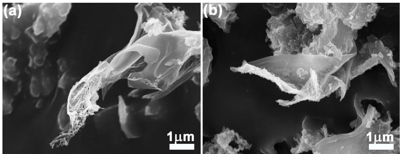
**Fig. S2** SEM images of the (a) CNS/EG-5 and (b) CNS/EG-20 hybrids.
