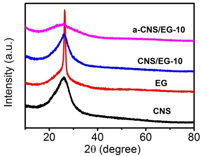
**Fig. S3** XRD patterns of CNS, EG, CNS/EG-10, and a-CNS/EG-10.
