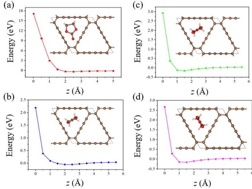
**Figure S2.** (a-d) Potential energy profiles of the other four trail orientations of EC molecule approaching the pore in graphdiyne.  $z$  denotes the distance between the geometric center of EC and the graphdiyne plane. The inset images show the configurations of EC approaching graphdiyne.
