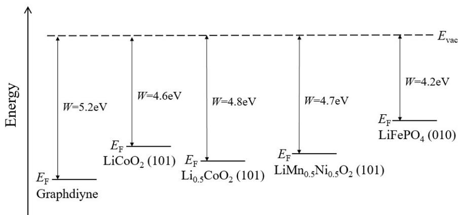
**Figure S3.** Schematic plot of the electron work functions of graphdiyne,  $LiCoO_2$  (101),  $Li_{0.5}CoO_2$  (101),  $LiMn_{0.5}Ni_{0.5}O_2$  (101), and  $LiFePO_4$  (010) surfaces.  $E_{vac}$  and  $E_F$  denote the energies of the vacuum and Fermi energy, respectively.  $W$  represents the electron work function.
