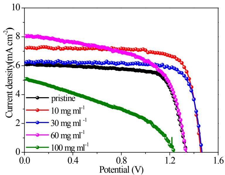
**Figure S8** J-V curves of inorganic PSCs with various concentration of the  $\text{CuInS}_2/\text{ZnS}$  QDs under air mass 1.5 global (AM1.5G,  $100 \text{ mW cm}^{-2}$ ) illumination.
