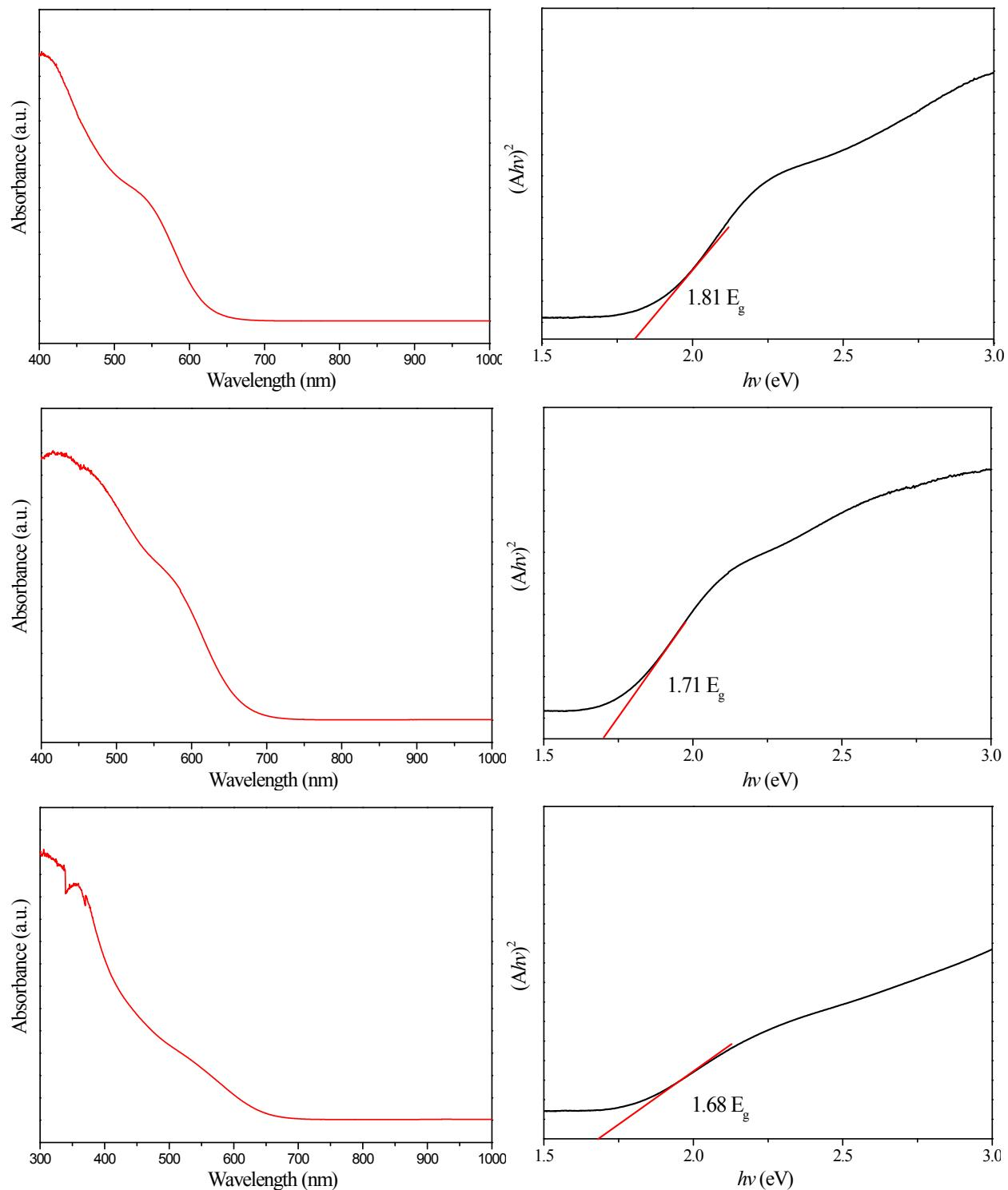
**Figure S2** Absorption spectra and corresponding  $(Ahv)^2$  vs energy ( $h\nu$ ) curves of CuInS<sub>2</sub>/ZnS QDs.
