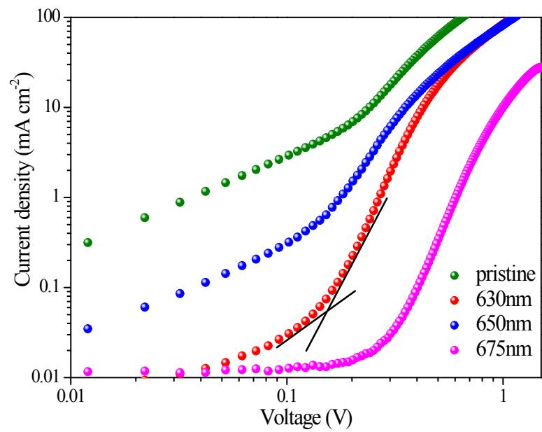
**Figure S7**  $J$ - $V$  curves of inorganic PSC devices under dark conditions.
