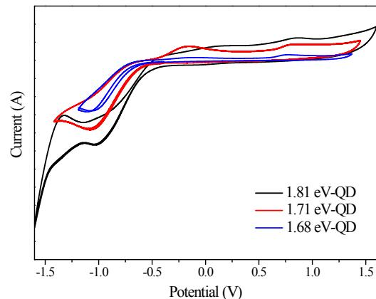
**Figure S1** Cyclic voltammetry curves of CuInS<sub>2</sub>/ZnS QDs the corresponding parameters are shown in Table S1.
