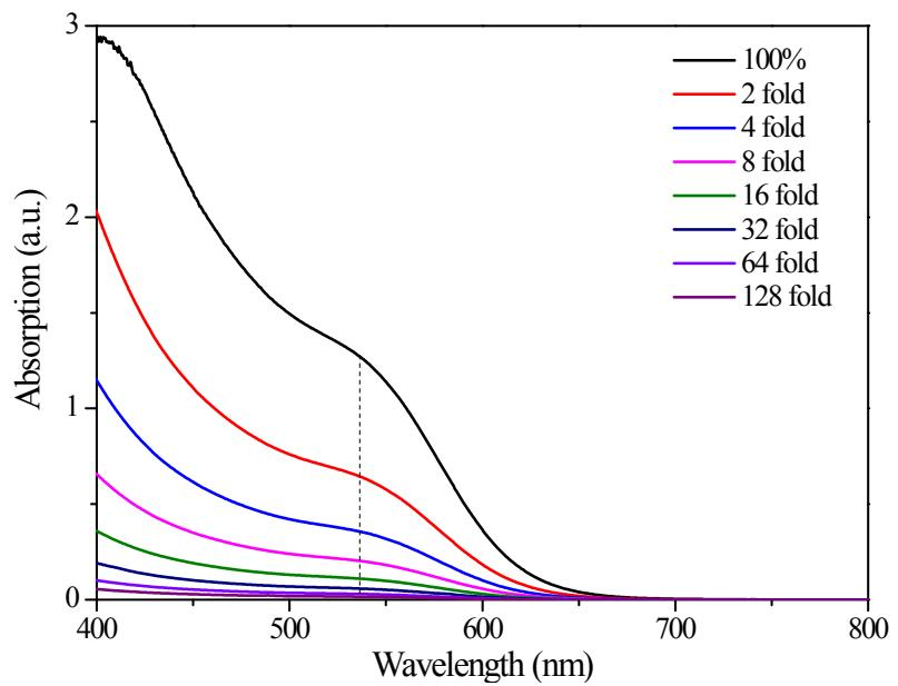
**Figure S3** UV-vis absorption spectra of CuInS<sub>2</sub>/ZnS QDs in diluted solutions.
