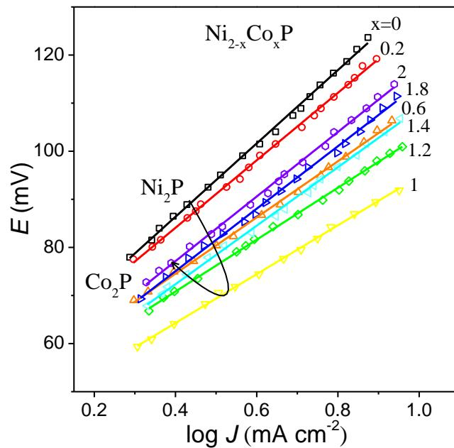
**Figure S13.** Tafel plots for the  $\text{Ni}_{2-x}\text{Co}_x\text{P}$  NCs. Tafel slopes for  $\text{Ni}_{2-x}\text{Co}_x\text{P}$  ( $x$  from 0 to 0.2, 0.6, 1, 1.2, 1.4, 1.6, 1.8, 2) are: 76, 70, 58, 51, 54, 61, 65, 67  $\text{mV dec}^{-1}$ .
