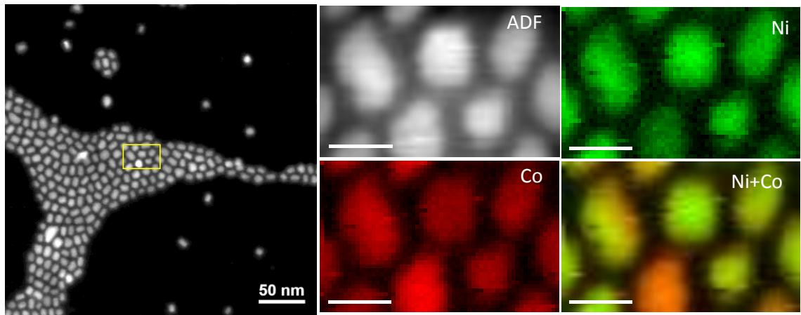
**Figure S8.** STEM – EELS elemental composition maps of a selected area of  $\text{Ni}_{0.4}\text{Co}_{1.6}\text{P}$  nanocrystals on the left image: Ni (green), Co (red) and combination Ni+Co.
