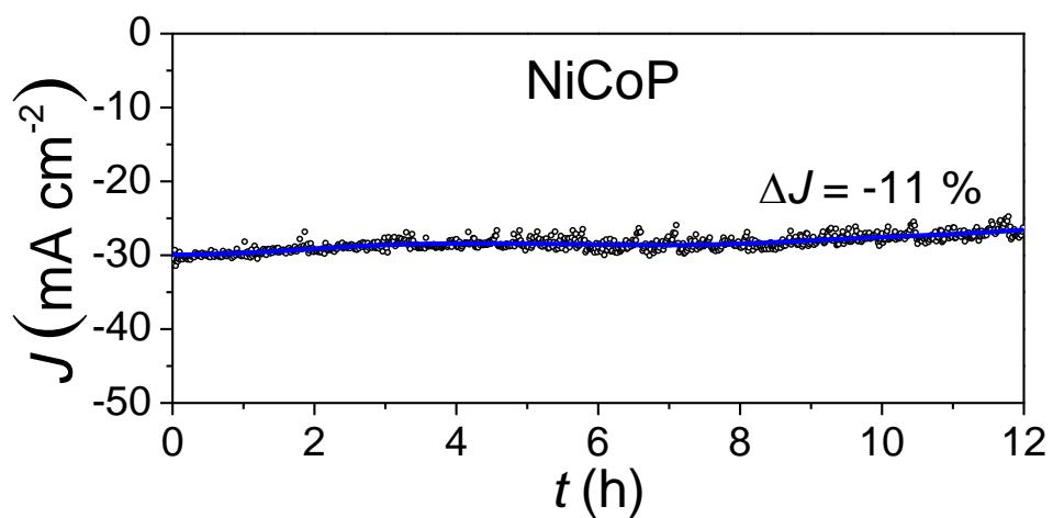
**Figure S14.** Time-dependent current density curve of  $\text{NiCoP}$  at an overpotential of 150 mV for 12 h.
