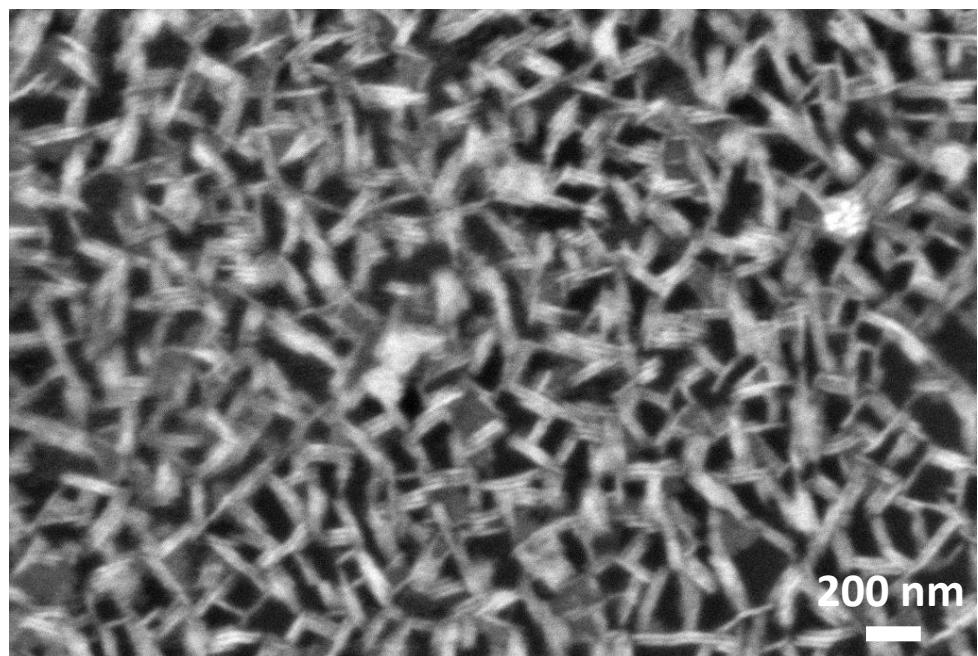
**Figure S12.** SEM micrograph of Co<sub>2</sub>P nanorods obtained using Co(NO<sub>3</sub>)<sub>2</sub> · 6H<sub>2</sub>O instead of CoCl<sub>2</sub> as cobalt precursor (Co(NO<sub>3</sub>)<sub>2</sub>·6H<sub>2</sub>O : HDA : TPP = 1 : 10 : 10)
