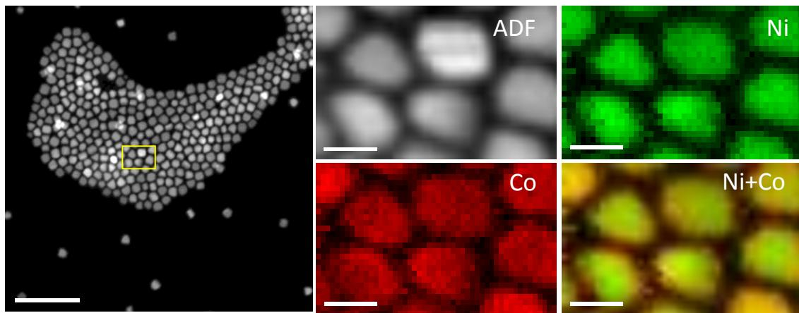
**Figure S6.** STEM – EELS elemental composition maps of a selected area of NiCoP nanocrystals on the left image: Ni (green), Co (red) and combination Ni+Co.
