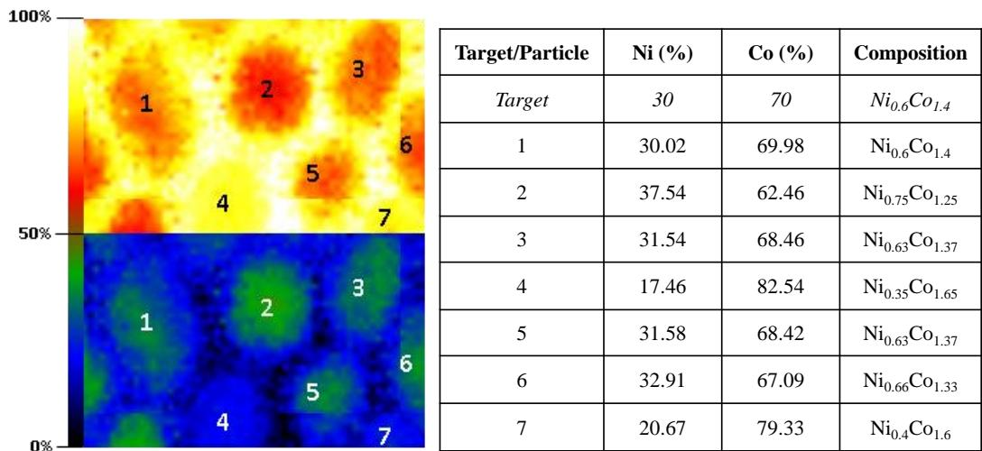
**Figure S9.** Ni and Co quantification maps obtained in the squared areas of the STEM images in Figure S8, together with a table representing the quantification of the numbered particles.
