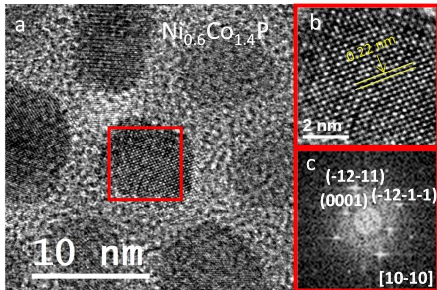
**Figure S4.** HRTEM micrograph of  $\text{Ni}_{0.6}\text{Co}_{1.4}\text{P}$  NCs (a), detail of the NC in red (b) and its corresponding power spectrum (c).
