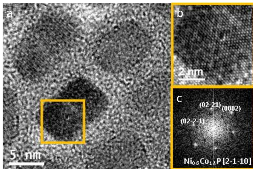
**Figure S5.** HRTEM micrograph of  $\text{Ni}_{0.6}\text{Co}_{1.4}\text{P}$  NCs (a), detail of the NC in yellow (b) and its corresponding power spectrum (c).
