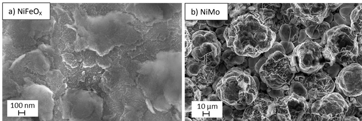
Figure S6: Scanning electron microscopy images of NiFeO<sub>x</sub> (a) and NiMo (b) after the measurement under simulated day-night-cycle conditions (6h of operation under 10 mA/cm<sup>2</sup>, no bias over night). For NiFeO<sub>x</sub> (a) it can be seen that catalyst layers remain on the surface, although the size of the NiFeO<sub>x</sub> structures decreased compared to figure S1. In the case of NiMo (b), the surface morphology is similar compared to figure S2 (a, e).
