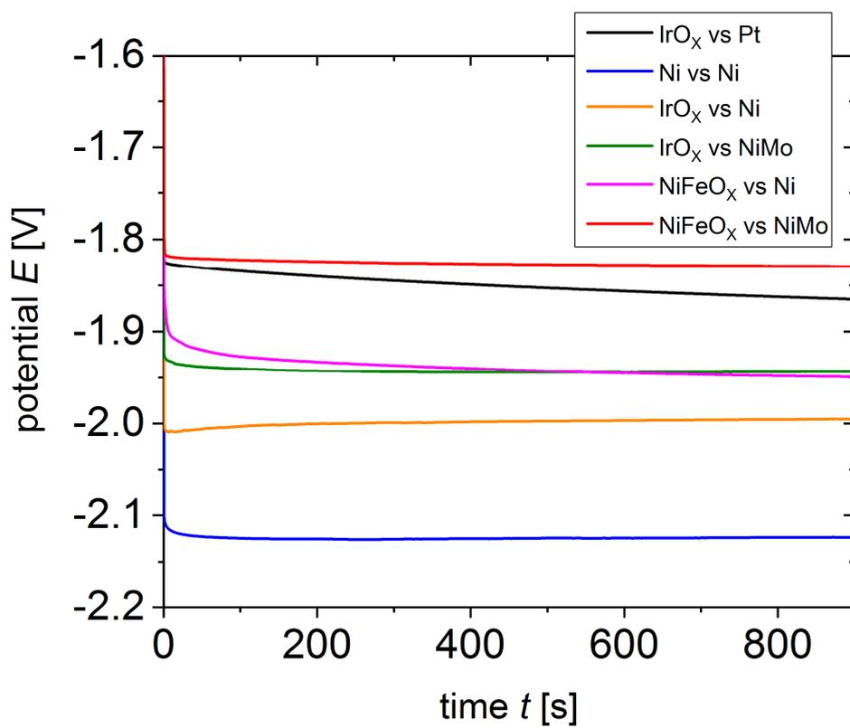
Figure S4: Chronopotentiometry scans for different catalyst systems on 50.3 cm<sup>2</sup> geometrical electrode area.
