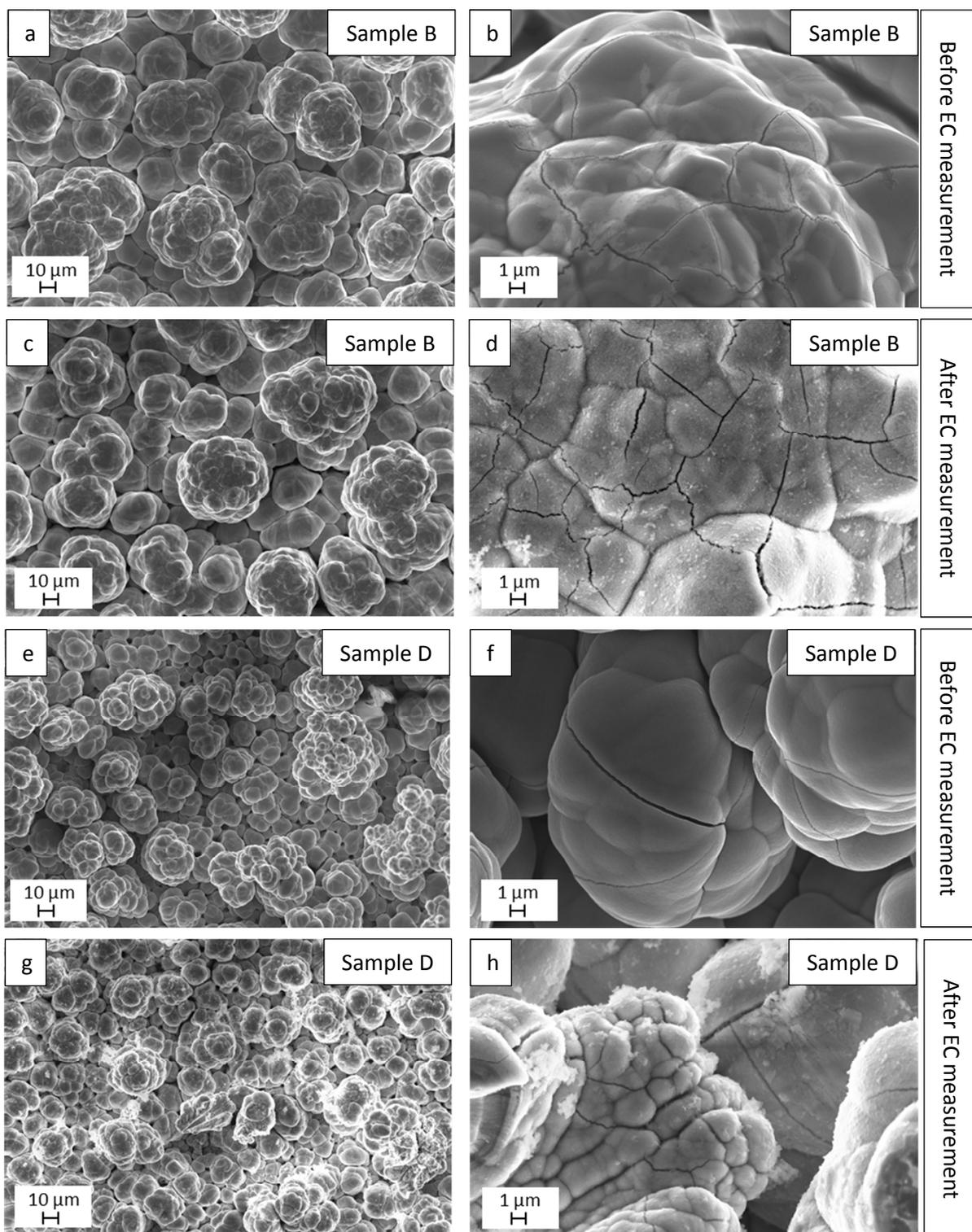
Figure S2: Scanning electron microscopy (SEM) images of NiMo samples B (a, b, c, d) and D (e, f, g, h) before (a+b, e+f) and after (c+d, g+h) the electrochemical measurements. Both samples were deposited under constant charge density conditions ( $Q_{\text{dep}} = -192 \text{ C/cm}^2$ ) which results in the same surface morphology (compare a+b to e+f). The obtained surface morphology is well preserved after
