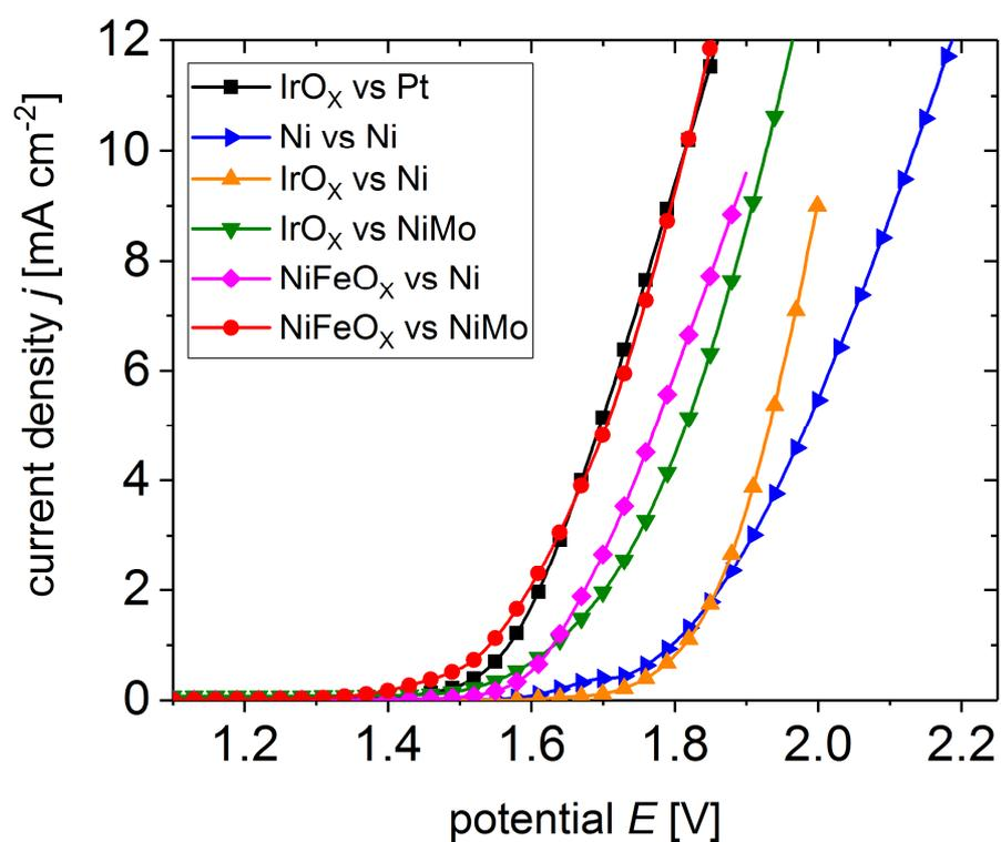
Figure S3: Linear sweep voltammetry curves of different catalyst systems on  $50.3 \text{ cm}^2$  geometrical electrode area.
