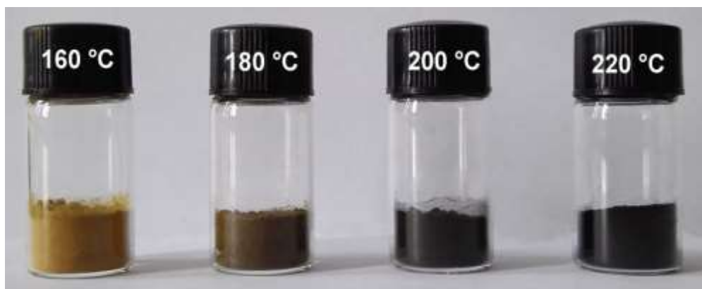
Figure S1. The photo of S160, S180, S200 and S220 of ca. 2 g each produced at 160, 180, 200 and 220 °C, respectively. The color of the materials changes from yellow to black as elevating reaction temperature.
