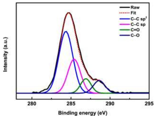
Fig. S7 XPS spectra of the narrow scan for elemental C of TiO<sub>2</sub>/GY-5 after photocatalytic reaction.
