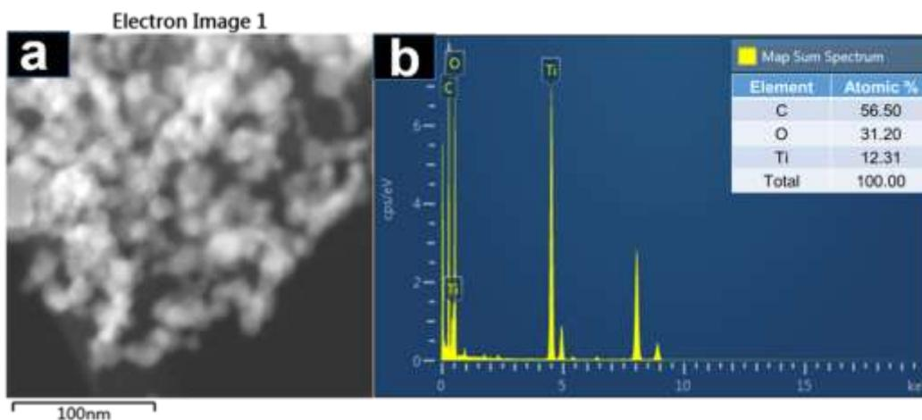
Fig. S3 (a) TEM and (b) EDS spectrum of TiO<sub>2</sub>/GY-5 sample
