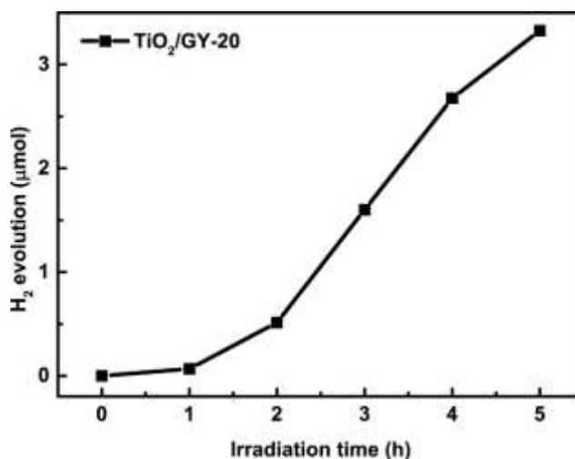
Fig. S6 Hydrogen evolution of TiO<sub>2</sub>/GY-20 nanocomposite
