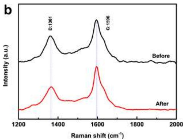
Fig. S8 (a) Raman spectra and (b) the corresponding magnified Raman spectra at 1200-2000 nm of TiO<sub>2</sub>/GY-5 before and after photocatalytic reaction.
