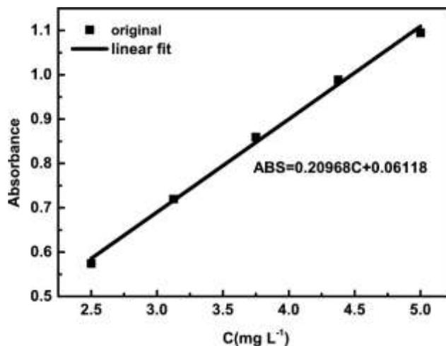
Fig. S1 A linear fit using five different concentrations of MB
