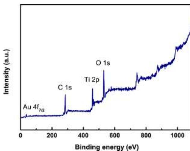
Fig. S5 XPS spectrum of TiO<sub>2</sub>/ $\gamma$ -GY-5 nanocomposite
