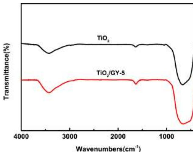
Fig. S2 Fourier transform infrared (FT-IR) spectra of TiO<sub>2</sub> and TiO<sub>2</sub>/GY-5
