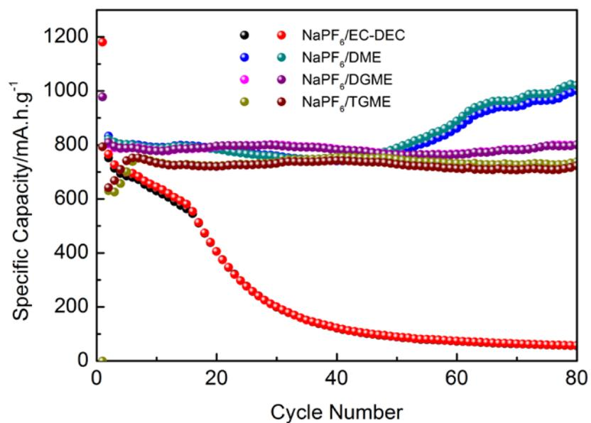
Fig. S6. Cycling performances of the FeS<sub>2</sub>@C at 0.5 A g<sup>-1</sup> in the electrolytes with different solvents: NaPF<sub>6</sub>/EC-DEC, NaPF<sub>6</sub>/DME, NaPF<sub>6</sub>/DGME, NaPF<sub>6</sub>/TGME. Voltage range: 0.005 ~ 3V
