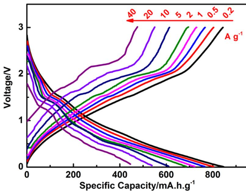
Fig. S12 Charge-discharge profiles of the FeS<sub>2</sub>@C in NaPF<sub>6</sub>/DME at different current densities from 0.2 to 40 A g<sup>-1</sup>. Voltage range: 0.005 ~ 3 V.
