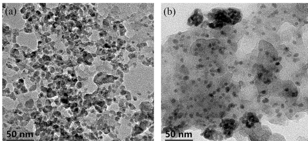
Fig. S16. TEM images of FeS<sub>2</sub>@C electrode at the fully charged state: (a) pristine electrode, (b) electrode cycled after 1000 cycles
