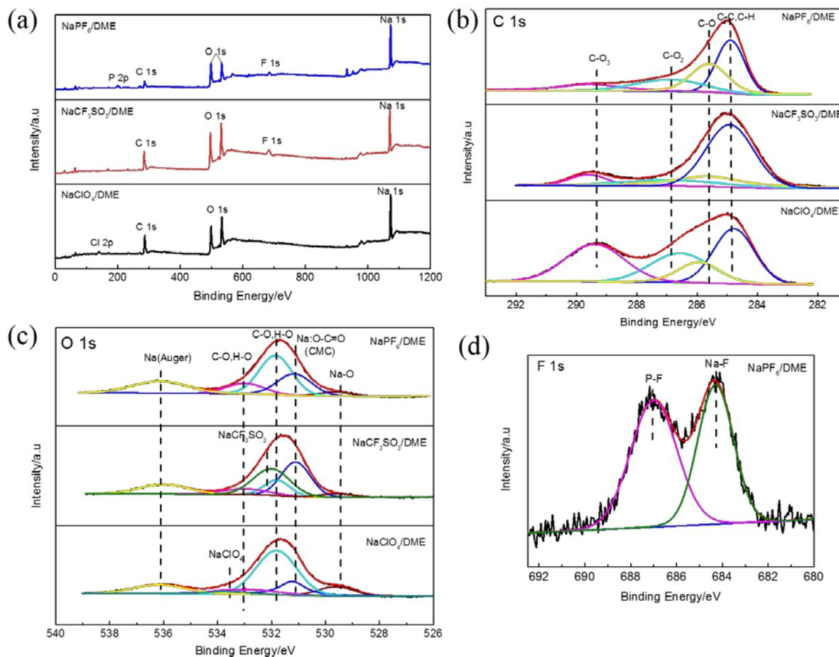
Fig. S9. Typical XPS spectra of the electrode cycled in NaPF<sub>6</sub>/DME, NaCF<sub>3</sub>SO<sub>3</sub>/DME and NaClO<sub>4</sub>/DME after the initial discharge process: (a) survey spectra, (b) high-resolution image of C 1s band, (c) high-resolution image of O 1s band, (d) high-resolution image of F 1s band.
