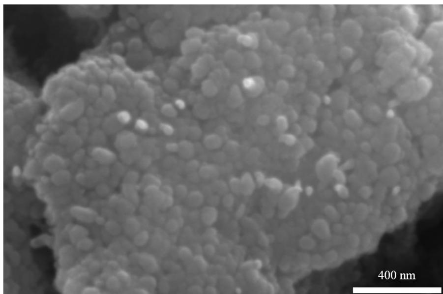
Fig. S15. SEM images of FeS<sub>2</sub>@C electrode at the fully charged state after 1000 cycles
