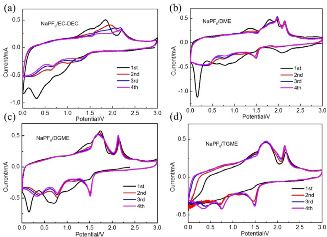
Fig. S5. CV curves of the as-prepared FeS<sub>2</sub>@C electrode in (a) NaPF<sub>6</sub>/EC-DEC; (b) NaPF<sub>6</sub>/DME; (c) NaPF<sub>6</sub>/DGME; (d) NaPF<sub>6</sub>/TGME. Scanning rates: 0.2 mV s<sup>-1</sup>; voltage range: 0.005 - 3 V
