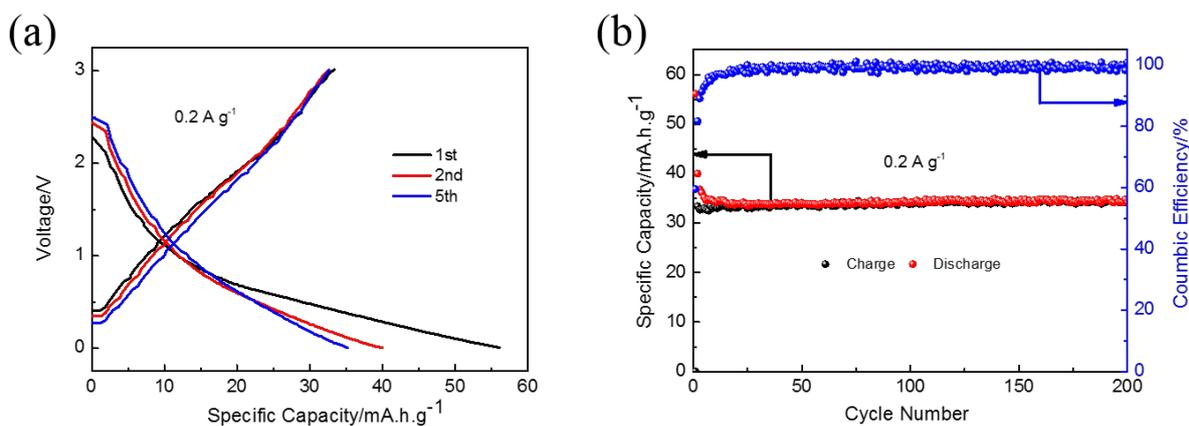
Fig. S7. (a) The charge-discharge profiles and (b) cycling performances of carbon derived from citric acid at 0.2 A g<sup>-1</sup>;
