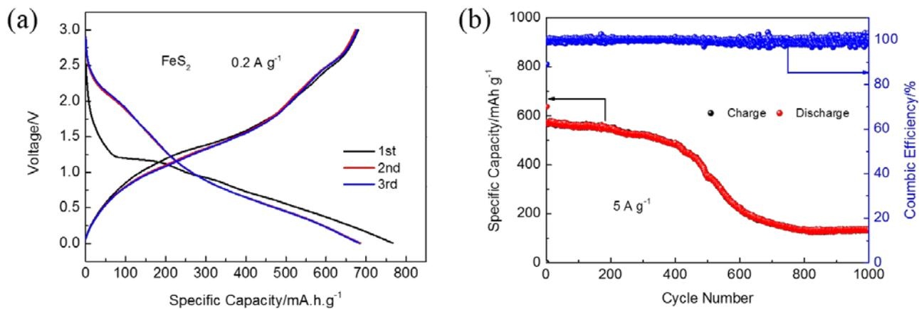
Fig. S14 (a) Charge-discharge profiles of the FeS<sub>2</sub> in NaPF<sub>6</sub>/DME at 0.2 A g<sup>-1</sup>; (b) cycling performances of FeS<sub>2</sub> at 5 A g<sup>-1</sup>; voltage range: 0.005 ~ 3 V.
