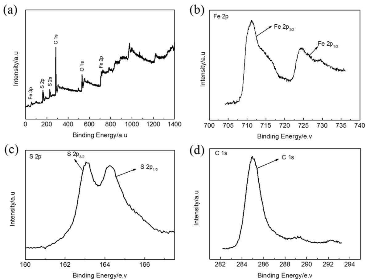
Fig. S1. Typical XPS spectra of the FeS<sub>2</sub>@C composite: (a) survey spectra, (b) high-resolution image of Fe 2p band, (c) high-resolution image of S 2p band, (d) high-resolution image of C 1s band
