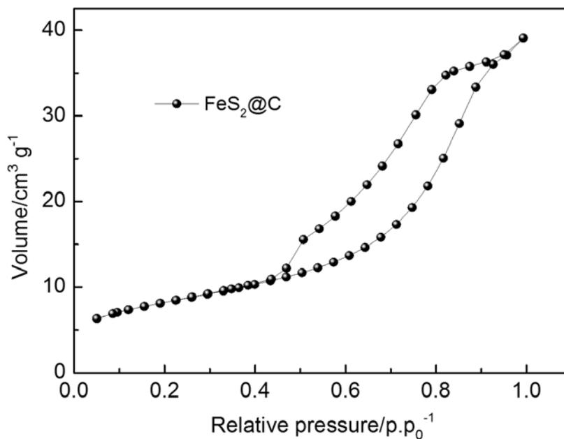
Fig. S4. N<sub>2</sub> adsorption–desorption isotherm of the as prepared FeS<sub>2</sub>@C
