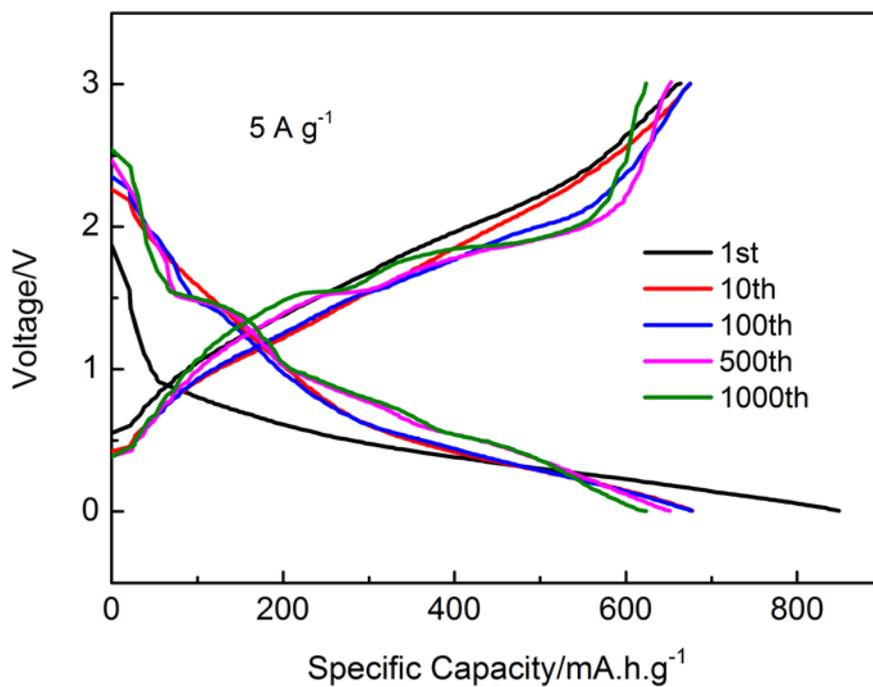
Fig. S13 Charge-discharge profiles of the FeS<sub>2</sub>@C in NaPF<sub>6</sub>/DME at 5 A g<sup>-1</sup> of different cycles. Voltage range: 0.005 ~ 3 V.
