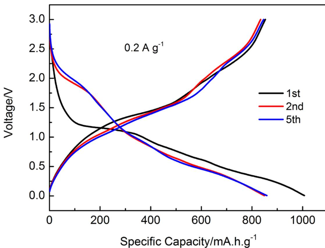
Fig. S11 Charge-discharge profiles of the FeS<sub>2</sub>@C in NaPF<sub>6</sub>/DME at 0.2 A g<sup>-1</sup>. Voltage range: 0.005 ~ 3 V.
