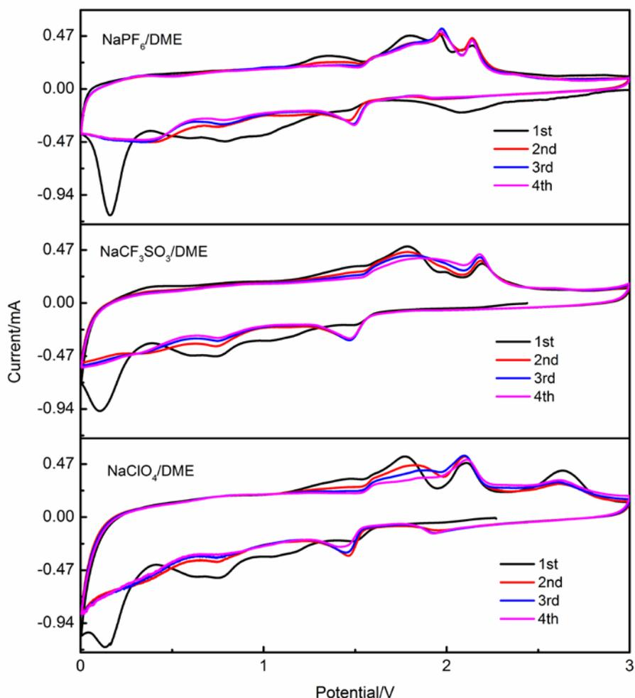
Fig. S8. CV curves of the as-prepared FeS<sub>2</sub>@C electrode in DME-based electrolyte with different Na salts: NaPF<sub>6</sub>/DME, NaCF<sub>3</sub>SO<sub>3</sub>/DME, NaClO<sub>4</sub>/DME. Scanning rates: 0.2 mV s<sup>-1</sup>; voltage range: 0.005 - 3 V.
