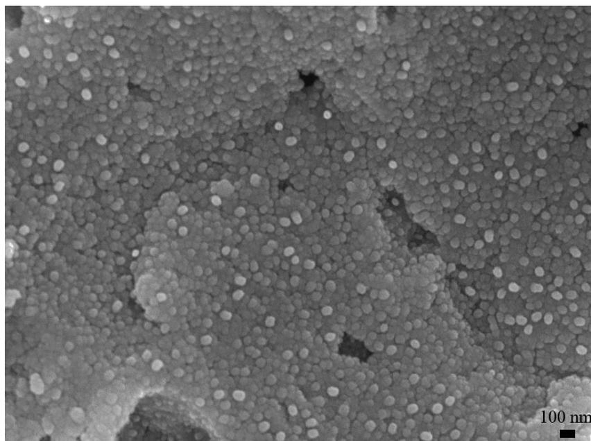
Fig. S3. SEM image of the as prepared FeS<sub>2</sub>@C
