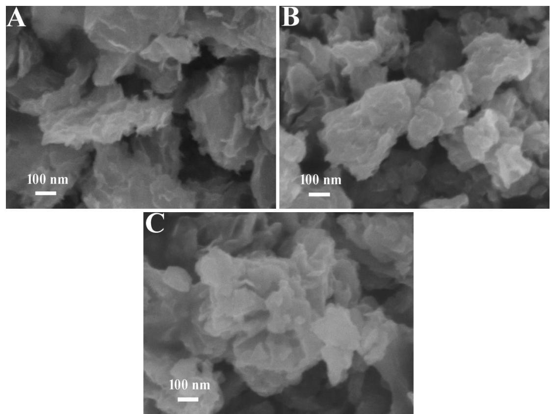
Figure S9. The SEM images of the CoAl-LDH nanosheets treatment conditions with different concentrations of NaOH (A) 2 M, (B) 8M, and (C) 10 M.
