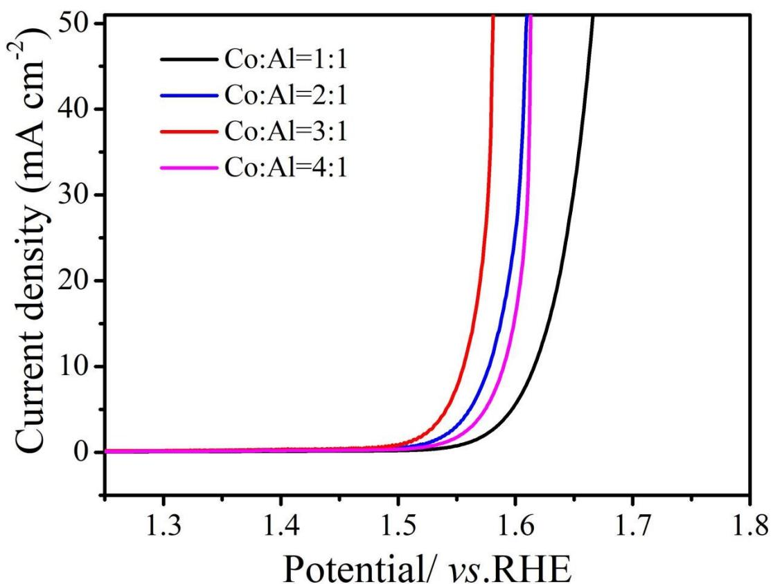
Figure S8. The OER performances of those samples with different Co:Al ratios were treated in mixed solution of 5 M NaOH and 3 M  $\text{Na}_2\text{S}$ .
