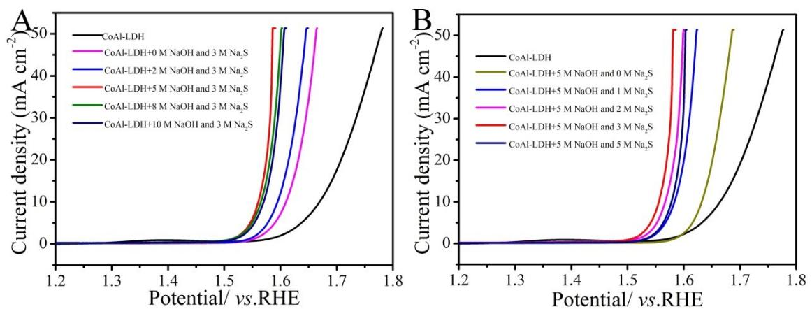
Figure S11. (A) The OER performances of the nanosheets treatment conditions with different concentrations of NaOH. (B) The OER performances of the nanosheets treatment conditions with different concentrations of  $\text{Na}_2\text{S}$ .
