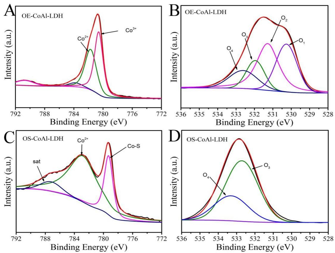
Figure S5. The XPS spectrums. (A) Co  $2\text{P}_{3/2}$  of OE-CoAl-LDH, (B) O 1s of OE-CoAl-LDH (C) Co  $2\text{P}_{3/2}$  of OS-CoAl-LDH (D) O 1s of OS-CoAl-LDH
