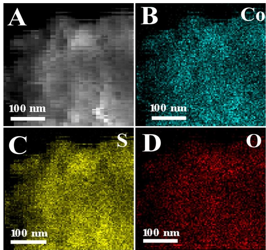
Figure S3. (A) The low-resolution TEM image of the PA- $\text{CoS}_x(\text{OH})_y$  and corresponding elemental mapping images of (B) Co, (C) S, and (D) O in the PA- $\text{CoS}_x(\text{OH})_y$ .
