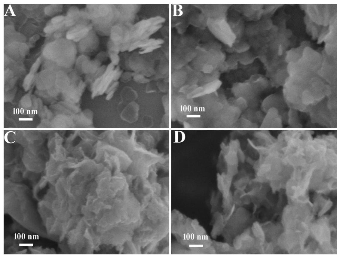
Figure S1. The SEM images of (A) CoAl-LDH, (B) OE-CoAl-LDH, (C) OS-CoAl-LDH (D) PA-CoS<sub>x</sub>(OH)<sub>y</sub>
