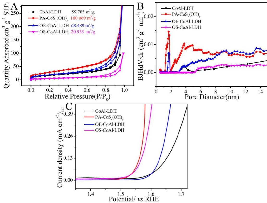
Figure S4. (A)  $\text{N}_2$  adsorption-desorption isotherms of CoAl-LDH, PA-CoS<sub>x</sub>(OH)<sub>y</sub>, OE-CoAl-LDH and OS-CoAl-LDH. (B) Corresponding BJH pore size distribution of CoAl-LDH, PA-CoS<sub>x</sub>(OH)<sub>y</sub>, OE-CoAl-LDH and OS-CoAl-LDH. (C) The OER performance of the CoAl-LDH, PA-CoS<sub>x</sub>(OH)<sub>y</sub>, OE-CoAl-LDH and OS-CoAl-LDH after BET normalization in 1.0M KOH.
