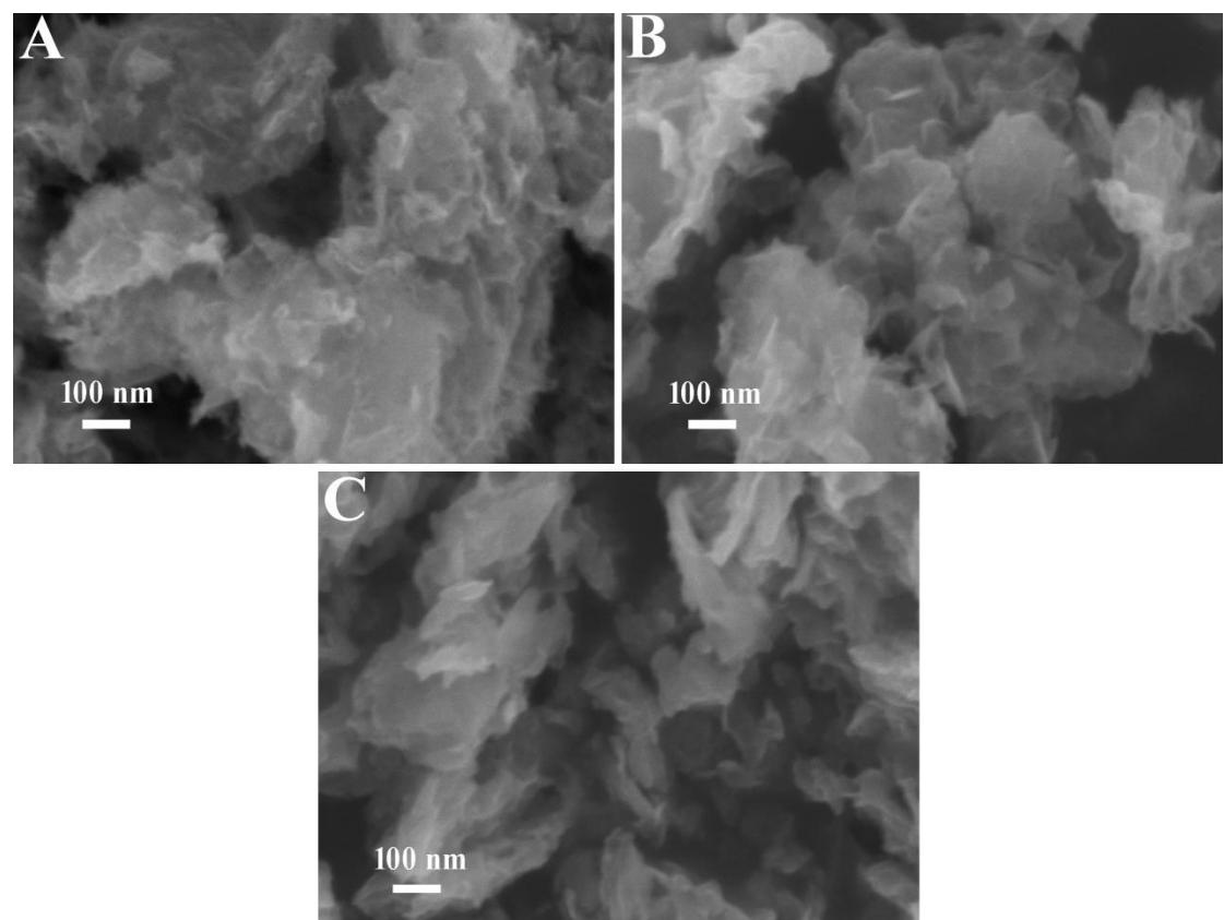
Figure S10. The SEM images of the CoAl-LDH nanosheets treatment conditions with different concentrations of  $\text{Na}_2\text{S}$  (A) 1 M, (B) 2M, and (C) 5 M.
