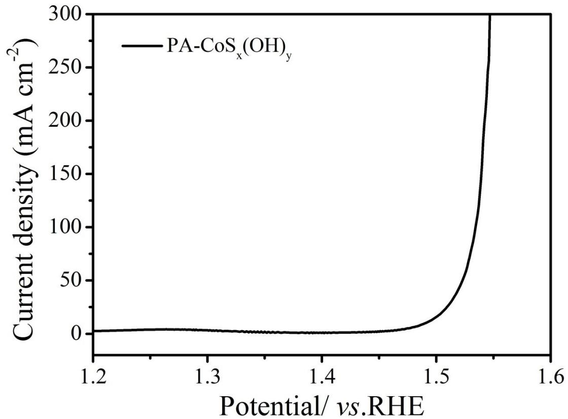
Figure S6.LSV polarization curves of PA-CoS<sub>x</sub>(OH)<sub>y</sub>/NF
