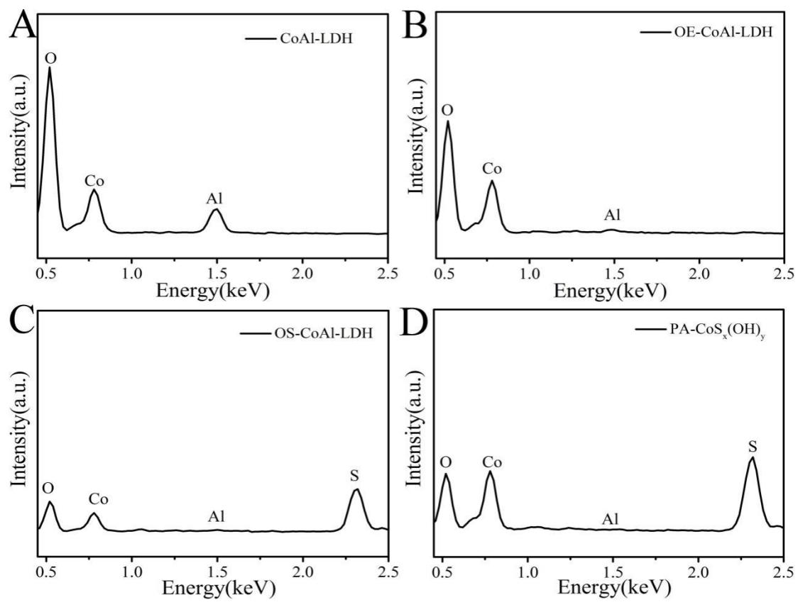
Figure S2. The EDX spectrums of (A) CoAl-LDH, (B) OE-CoAl-LDH, (C) OS-CoAl-LDH (D) PA-CoS<sub>x</sub>(OH)<sub>y</sub>
