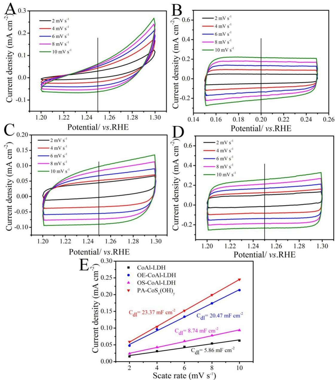
Figure S7. Tested the electrochemical surface area (ECSA) of CoAl-LDH, OE-CoAl-LDH, OS-CoAl-LDH and PA-CoS<sub>x</sub>(OH)<sub>y</sub> in 1.0 M KOH solution. (A) Cyclic voltammetry curves of (A) CoAl-LDH, (B) OE-CoAl-LDH, (C) OS-CoAl-LDH and (D) PA-CoS<sub>x</sub>(OH)<sub>y</sub> with different scanning rates. The capacitive current measured at 1.25 V vs RHE was plotting as a function of scan rate (E) CoAl-LDH, OE-CoAl-LDH, OS-CoAl-LDH and PA-CoS<sub>x</sub>(OH)<sub>y</sub>.
