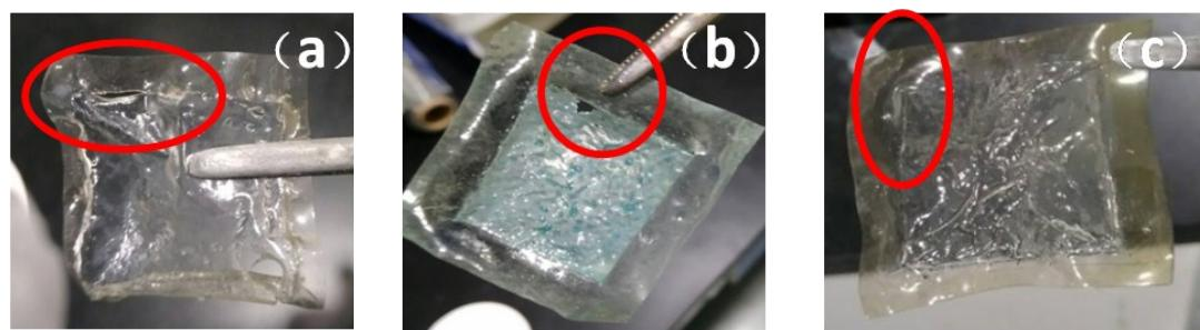
**Figure S7.** Images of AEMs after long-term charge-discharge cycles testing: (a) PSf-PTA-1.4, (b) PSf-c-PTA-1.4 and (c) PSf-c-QA-1.2.
