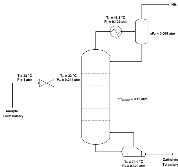
**Figure S10.** Schematic of the distillation model for ammonia separation from the anolyte based on Aspen HYSYS.
