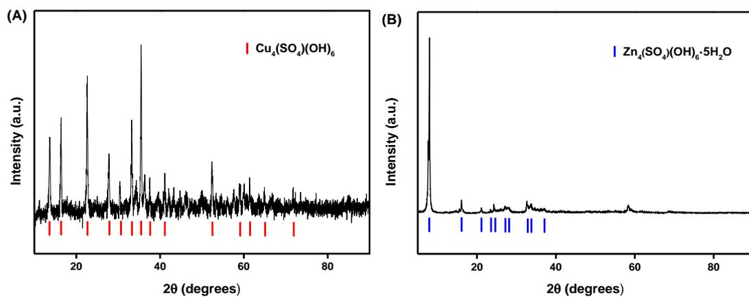
**Figure S7.** XRD patterns of the precipitates that produced during the thermal regeneration of anolyte effluent after (A) discharge and (B) charge processes.
