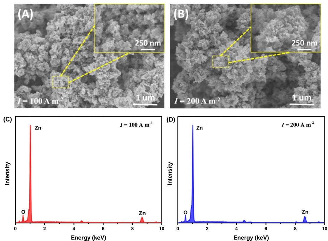
**Figure S6.** The SEM images of the zinc electrode and corresponding EDS spectrums after the constant-current discharge tests: (A) and (C)  $100 \text{ A m}^{-2}$ ; (B) and (D)  $200 \text{ A m}^{-2}$ .
