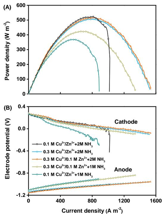
**Figure S3.** (A) Power density and (B) electrode potentials using different concentrations of Cu(II) and Zn(II) in the discharge process, with 1 M  $(\text{NH}_4)_2\text{SO}_4$  as the supporting electrolyte and 1 M or 2 M  $\text{NH}_3$  in the anolyte.
