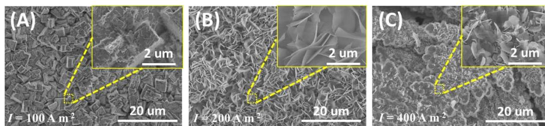
**Figure S2.** The SEM images of the zinc electrode after 30 minutes of the constant-current charge tests: (A)  $100 \text{ A m}^{-2}$  (B)  $200 \text{ A m}^{-2}$  (C)  $400 \text{ A m}^{-2}$ .
