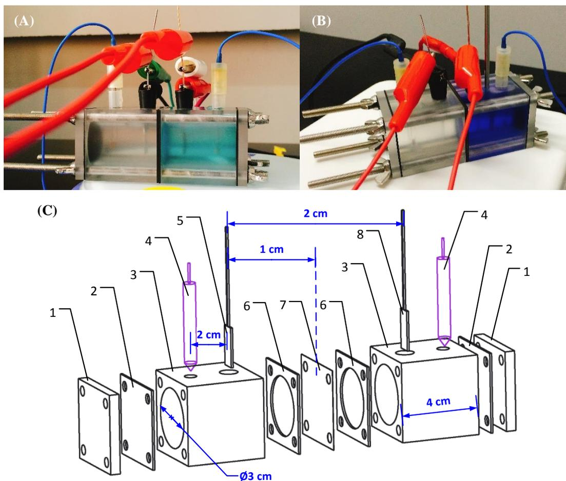
**Figure S1.** Test set-up for a Cu/Zn-TRAB. Photographs of a laboratory set-up during (A) discharge and (B) charge. (C) Exploded view drawing of the test Cu/Zn-TRAB (1-polycarbonate endplate, 2-fluoroelastomer gasket, 3-polycarbonate chamber, 4-Ag/AgCl reference electrode, 5-Zinc electrode, 6-another fluoroelastomer gasket, 7-anion exchange membrane, 8-copper electrode).
