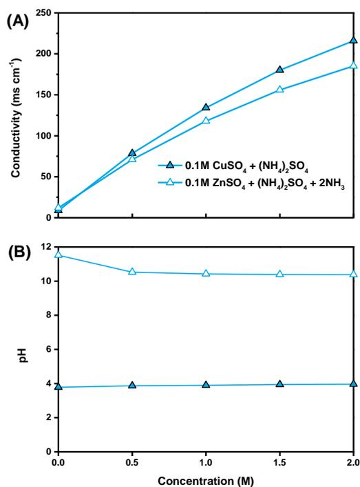
**Figure S4.** (A) Conductivity and (B) pH of 0.1 M  $\text{Cu}(\text{SO}_4)_2$  or 0.1 M  $\text{Zn}(\text{SO}_4)_2$  solutions with various concentrations of  $(\text{NH}_4)_2\text{SO}_4$ , with addition of 2 M  $\text{NH}_3$  in the Zn(II) solutions.
