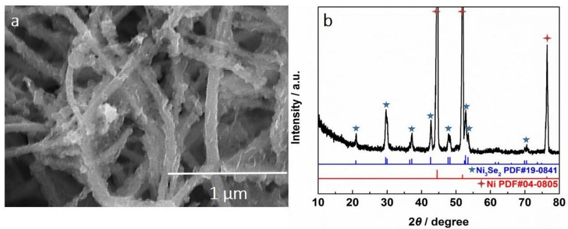
**Figure S8.** (a) SEM and (b) XRD of  $\text{Ni}_3\text{Se}_2/\text{NF}$ -0.4 after i-t curve analysis for OER.
