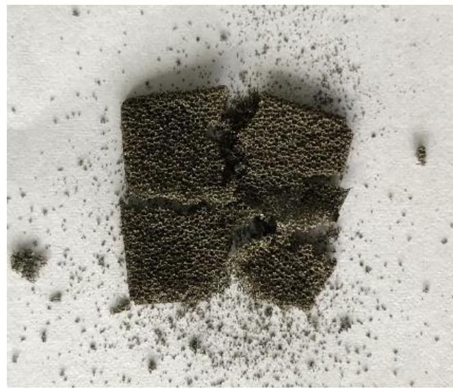
**Figure S2.** Picture showing the destruction of Ni foam while using 0.7 mmol Se powder for Ni<sub>3</sub>Se<sub>2</sub>/NF nanowire arrays.
