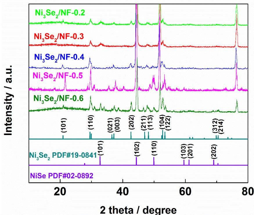
**Figure S4.** XRD patterns obtained for  $\text{Ni}_3\text{Se}_2/\text{NF}$  samples with Se powder concentration of 0.2 (fluorescent line), 0.3 (red line), 0.4 (blue line), 0.5 (pink line), and 0.6 mmol (green line).
