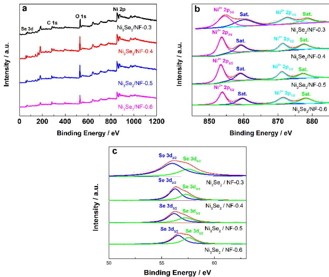
**Figure S5.** XPS of  $\text{Ni}_3\text{Se}_2/\text{NF}$  samples: (a) survey, (b) Ni 2p and (c) Se 3d
