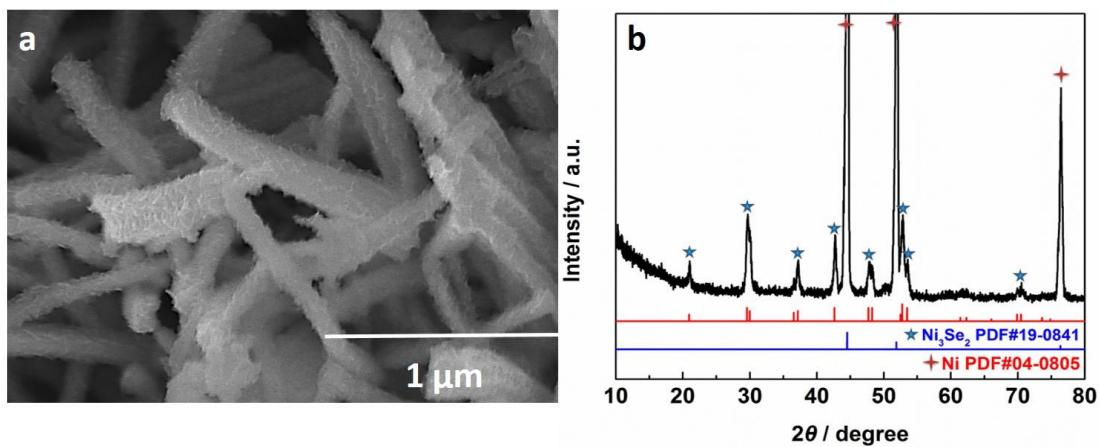
**Figure S7.** (a) SEM and (b) XRD of  $\text{Ni}_3\text{Se}_2/\text{NF}-0.4$  after i-t curve analysis for HER.
