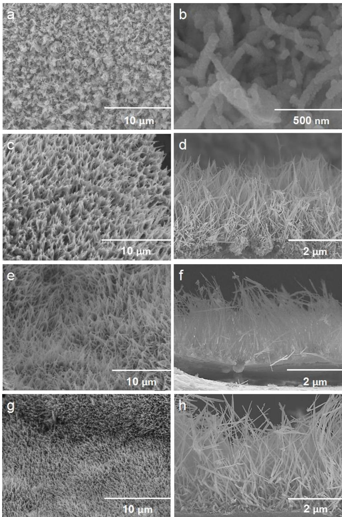
**Figure S1.** SEM images of Ni<sub>3</sub>Se<sub>2</sub>/NF-0.2 (a, b), Ni<sub>3</sub>Se<sub>2</sub>/NF-0.3 (c, d), Ni<sub>3</sub>Se<sub>2</sub>/NF-0.5 (e, f) and Ni<sub>3</sub>Se<sub>2</sub>/NF-0.6 (g, h).
