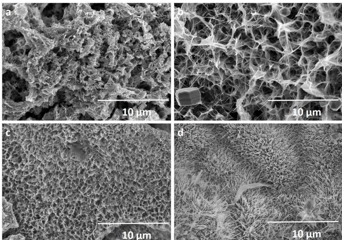
**Figure S3.** SEM images of nickel selenide prepared with different reaction time, (a) 6 h, (b) 12 h, (c) 18 h and (d) 24 h.
