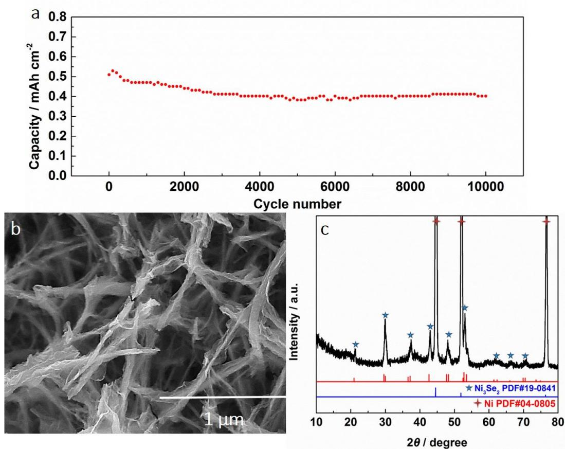
**Figure S6.** (a) Cycling stability of  $\text{Ni}_3\text{Se}_2/\text{NF}-0.4$ , (b) SEM and (c) XRD of  $\text{Ni}_3\text{Se}_2/\text{NF}-0.4$  after stability cycling analysis.
