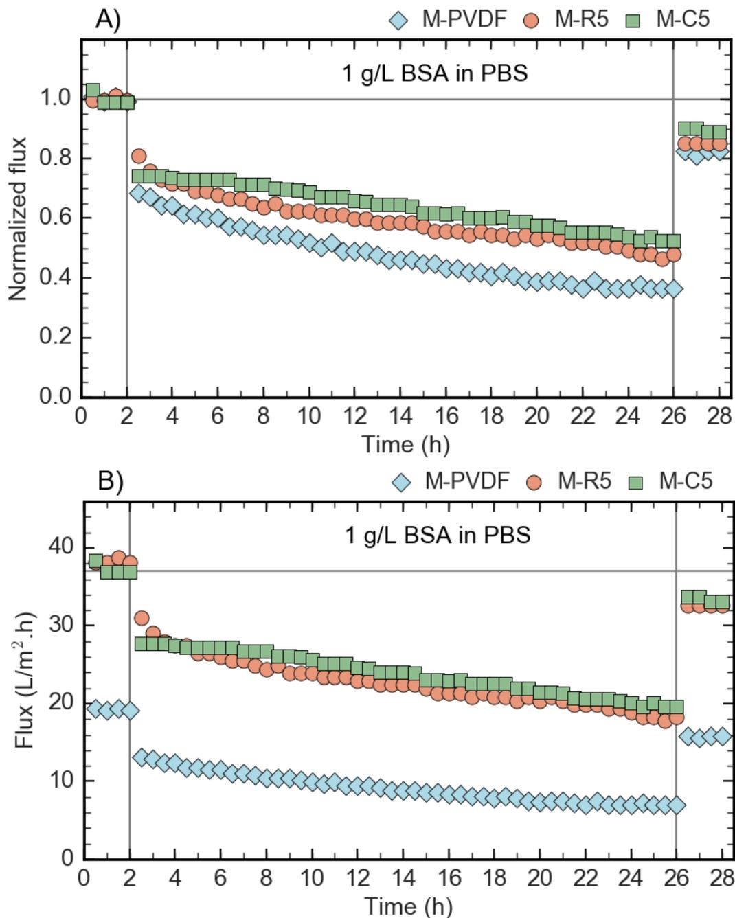
**Fig. S7** Long-term protein fouling resistance by 24 h filtration of M-PVDF (10 psi), M-R5 (5 psi), and M-C5 (10 psi) membranes. The fluxes are plotted (A) after normalizing by the average initial flux of each membrane; 19 L/m<sup>2</sup>.h for M-PVDF, 38 L/m<sup>2</sup>.h for M-R5, and 37 L/m<sup>2</sup>.h for M-C5, (B) without normalizing.
