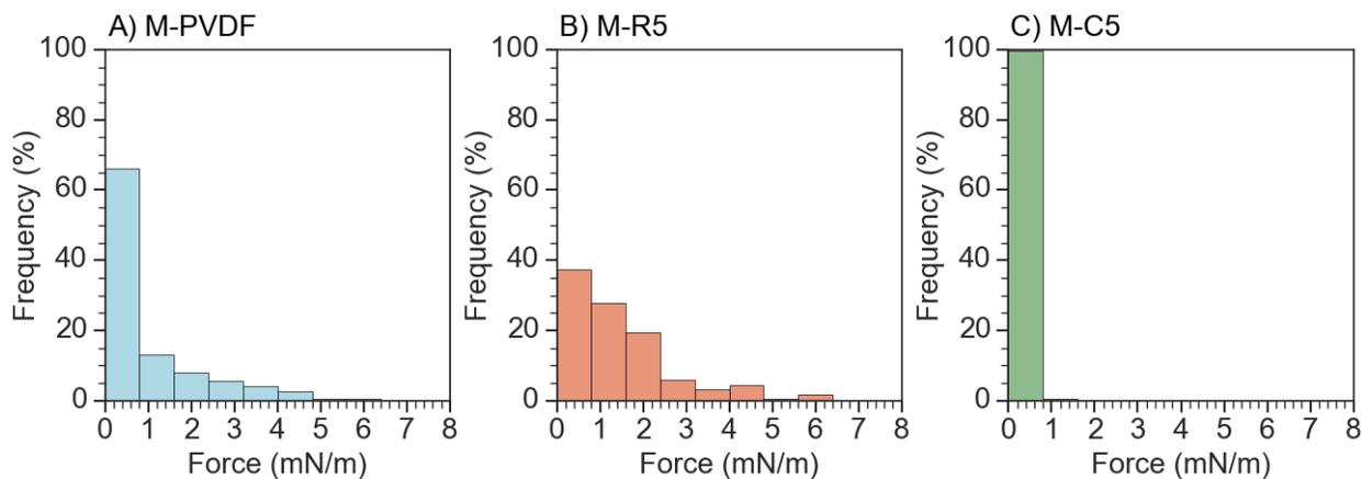
**Fig. S6** Distributions of normalized detachment force measurements between the AFM particle (foulant) probe and membranes (A) M-PVDF, (B) M-R5, and (C) M-C5.
