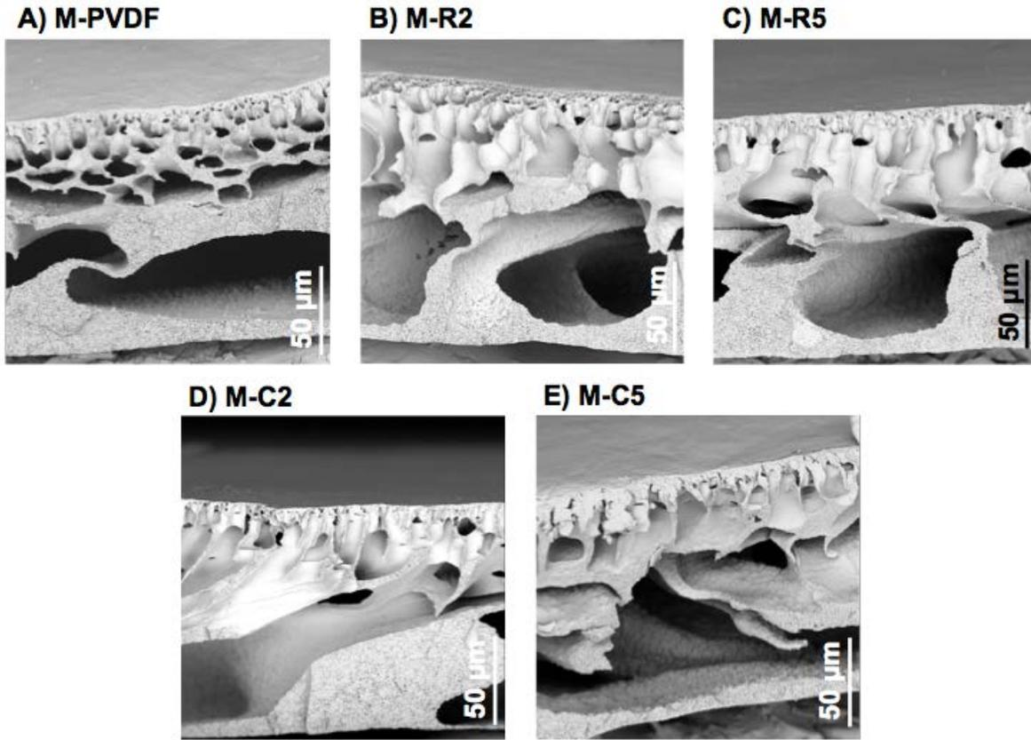
**Fig. S4** Tilted cross-sectional SEM images showing the surface and cross-sectional morphologies of membranes
