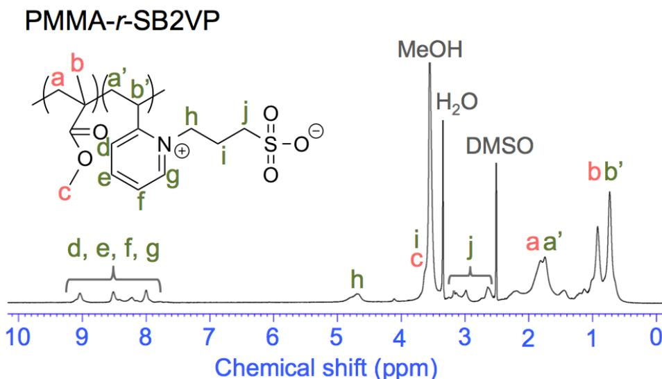
**Fig. S1**  $^1\text{H}$ -NMR spectrum of zwitterionic random copolymer PMMA-*r*-SB2VP
