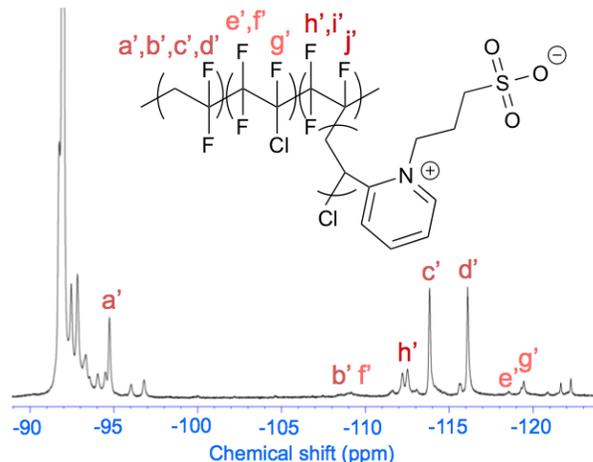
**Fig. S2**  $^{19}\text{F}$ -NMR spectra of (A) backbone copolymer PVDF-*co*-CTFE, and (B) comb copolymer PVDF-*g*-SB2VP
