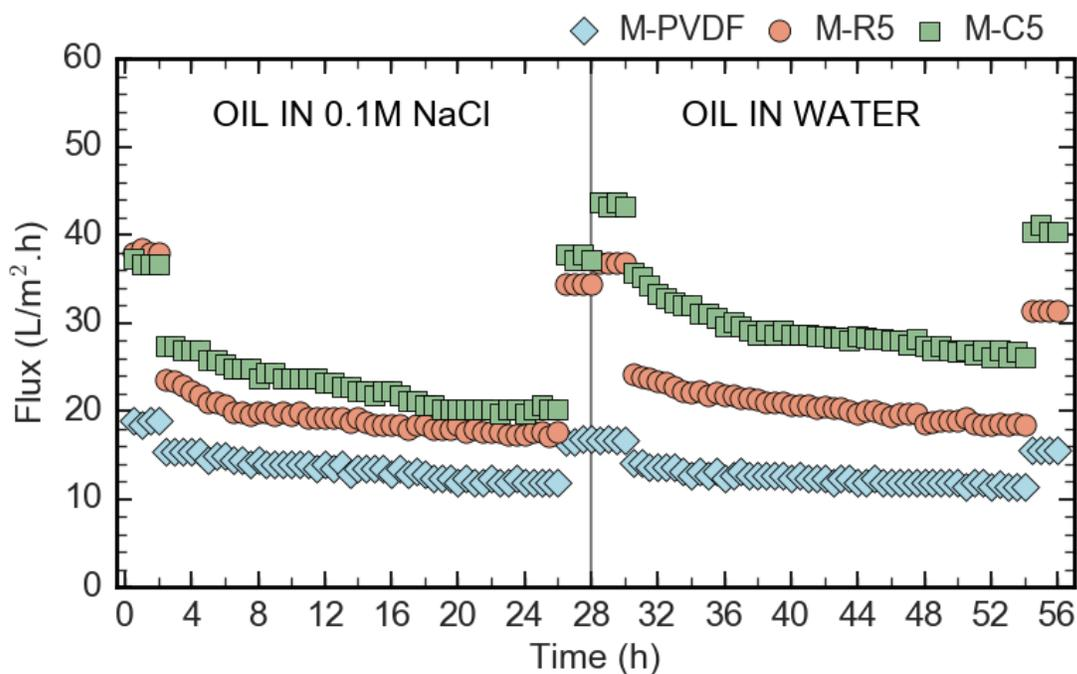
**Fig. S5** Long-term oil fouling resistance by filtration of M-PVDF (10 psi), M-R5 (5 psi), and M-C5 (10 psi) membranes. The fluxes are plotted without normalizing.
