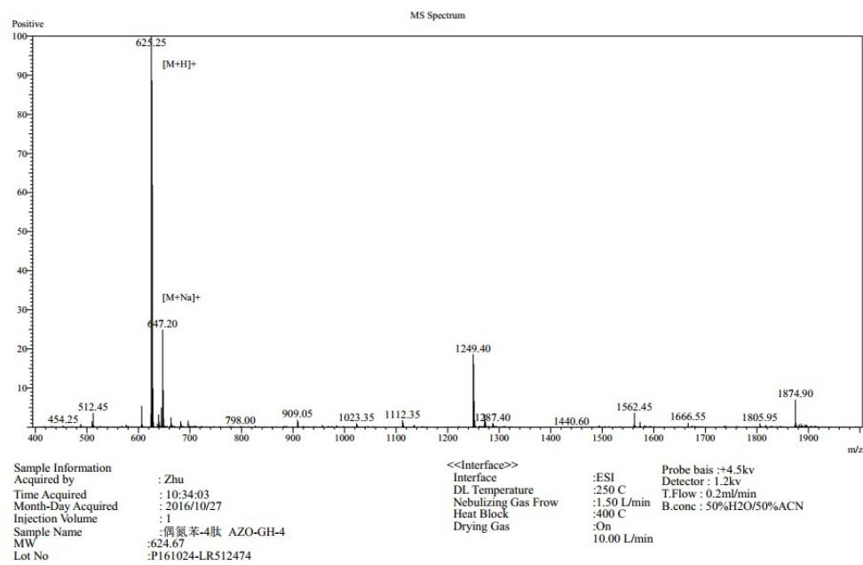
**Fig. S2** MS analysis of Azo-GFGH
