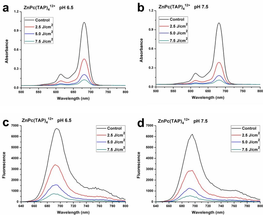
**Figure S2.** Photodegradation behaviors of  $\text{ZnPc(TAP)}_4^{12+}$ . The UV-Vis absorption spectra (500-800 nm) and fluorescence excitation spectra ( $\lambda_{\text{ex}}=610$  nm;  $\lambda_{\text{em}}=640, 800$  nm) of  $\text{ZnPc(TAP)}_4^{12+}$  at pH 6.5 (**a, c**) and pH 7.5 (**b, d**) after receiving different light dose (2.5, 5.0, 7.5  $\text{J/cm}^2$ , at 660 nm).
