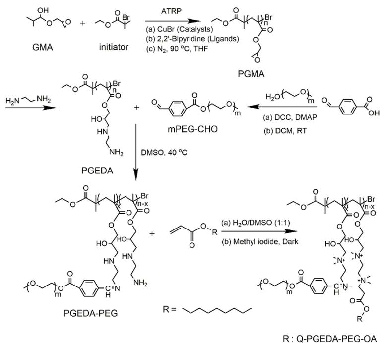
**Figure S1** Synthetic route of Q-PGEDA-PEG-OA.
