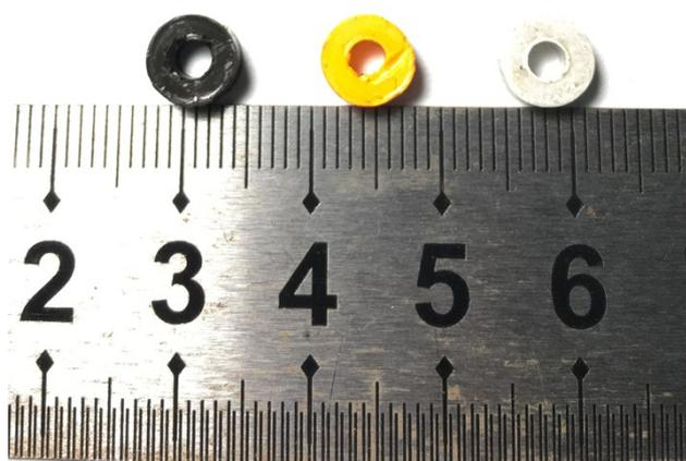
**Fig. S7** Photographs of MAPbI<sub>3</sub>, MAPbBr<sub>3</sub> and MAPbCl<sub>3</sub> crystal samples stored in N<sub>2</sub> for 180 days.
