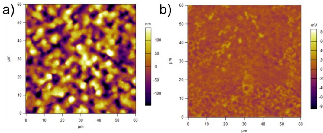
**Figure S1.** (a) Topography and KPFM image of the  $(\text{MA})_2(\text{PA})_2\text{Pb}_3\text{Br}_{10}$  film.
