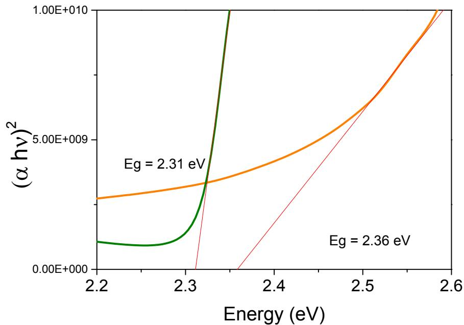
**Figure S2.** Tauc plots of  $(\text{PA})_2(\text{MA})_2\text{Pb}_3\text{Br}_{10}$  (orange line) and  $\text{MAPbBr}_3$  (green line) films.
