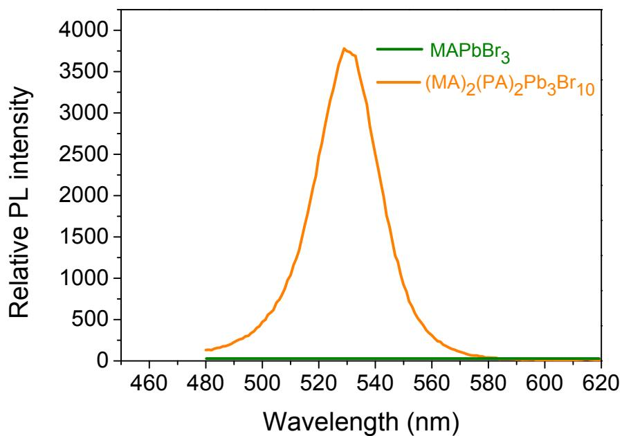
**Figure S3.** Room temperature PL spectrum of  $(\text{PA})_2(\text{MA})_2\text{Pb}_3\text{Br}_{10}$  and  $\text{MAPbBr}_3$  films excited at 470 nm.
