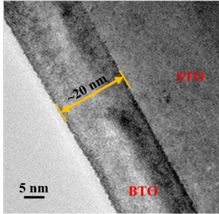
FIG. S1 Cross-section TEM image of BTO film grown on  $0^\circ$  miscut substrate.
