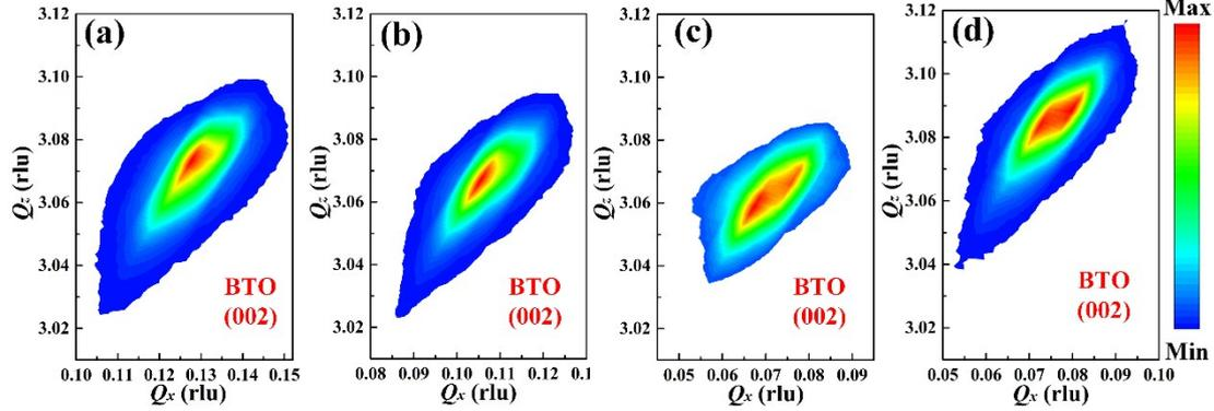
FIG. S3 RSM patterns of (002) reflections from BTO film grown on (a)  $0^\circ$ , (b)  $0.2^\circ$ , (c)  $1^\circ$  and (d)  $2^\circ$  miscut substrates.
