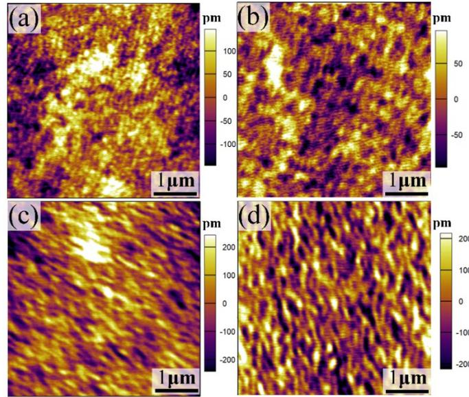
FIG. S4 Atomic force microscope images of BTO films grown on (a)  $0^\circ$ , (b)  $0.2^\circ$ , (c)  $1^\circ$  and (d)  $2^\circ$  miscut substrates.
