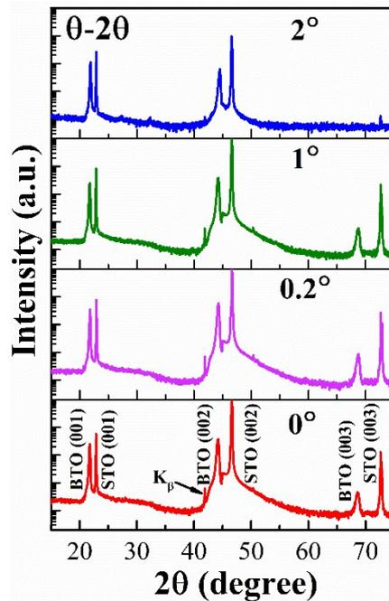
FIG. S2 Typical  $\theta$ - $2\theta$  XRD patterns of BTO films grown on various (001) STO miscut substrates.
