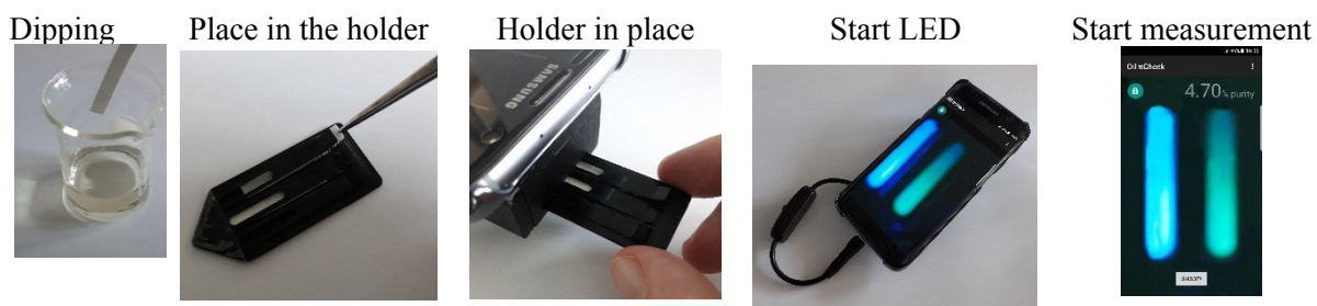
Fig. S6 Successive steps to analyze the purity of a gasoline fuel: dip in sample, place in the holder, start the LED, place the holder and press the shoot button to obtain directly the gasoline purity on screen.
