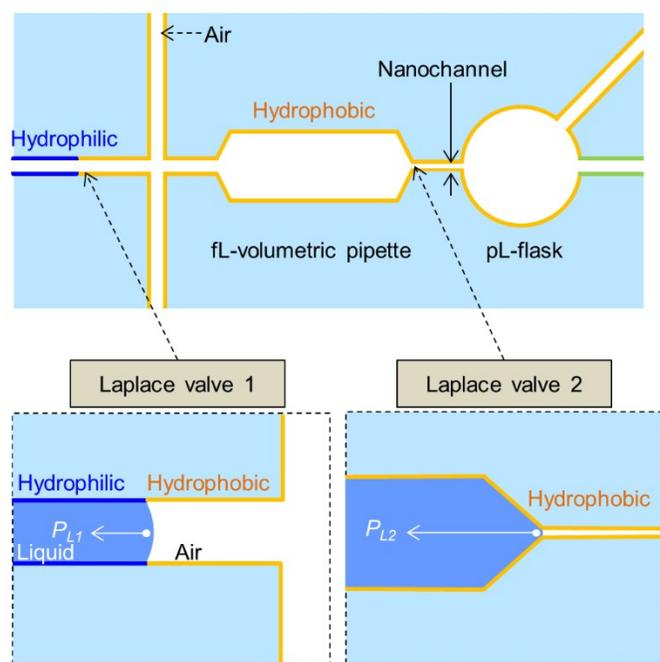
**Figure S3.** Structure of the fL-volumetric pipette and pL-flask.
