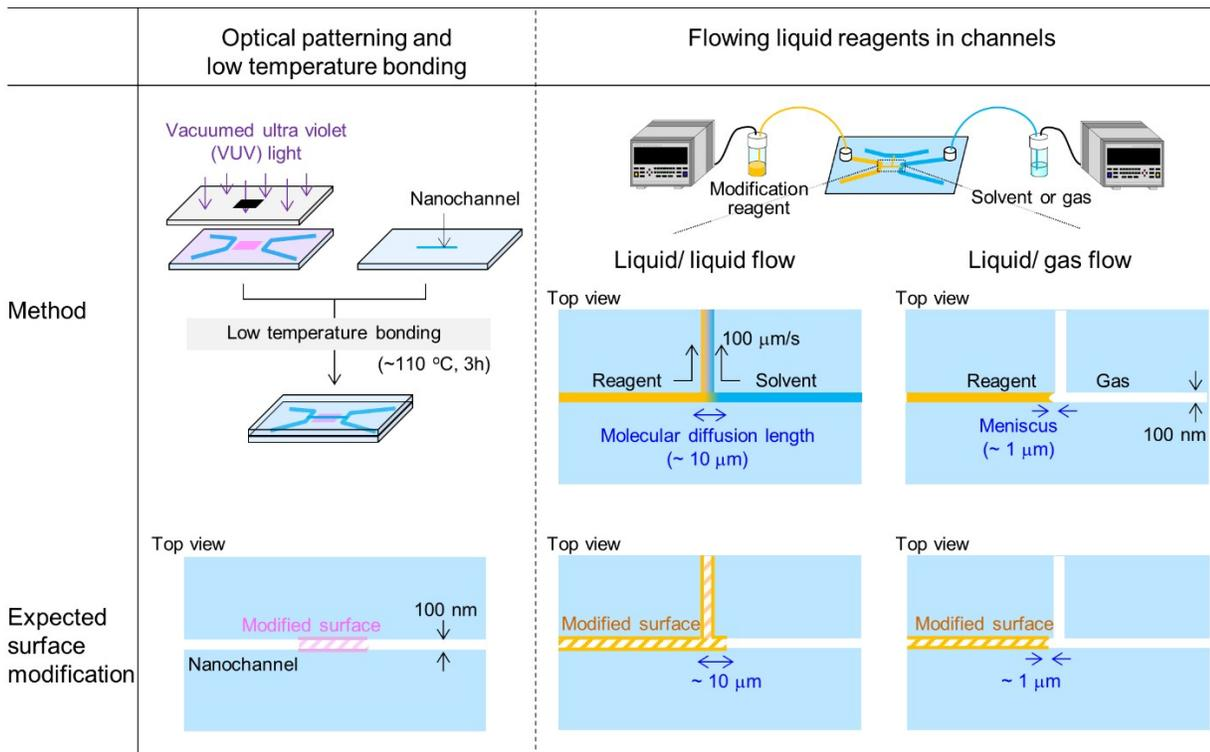
**Figure S4.** Principles of the partial surface modification methods.
