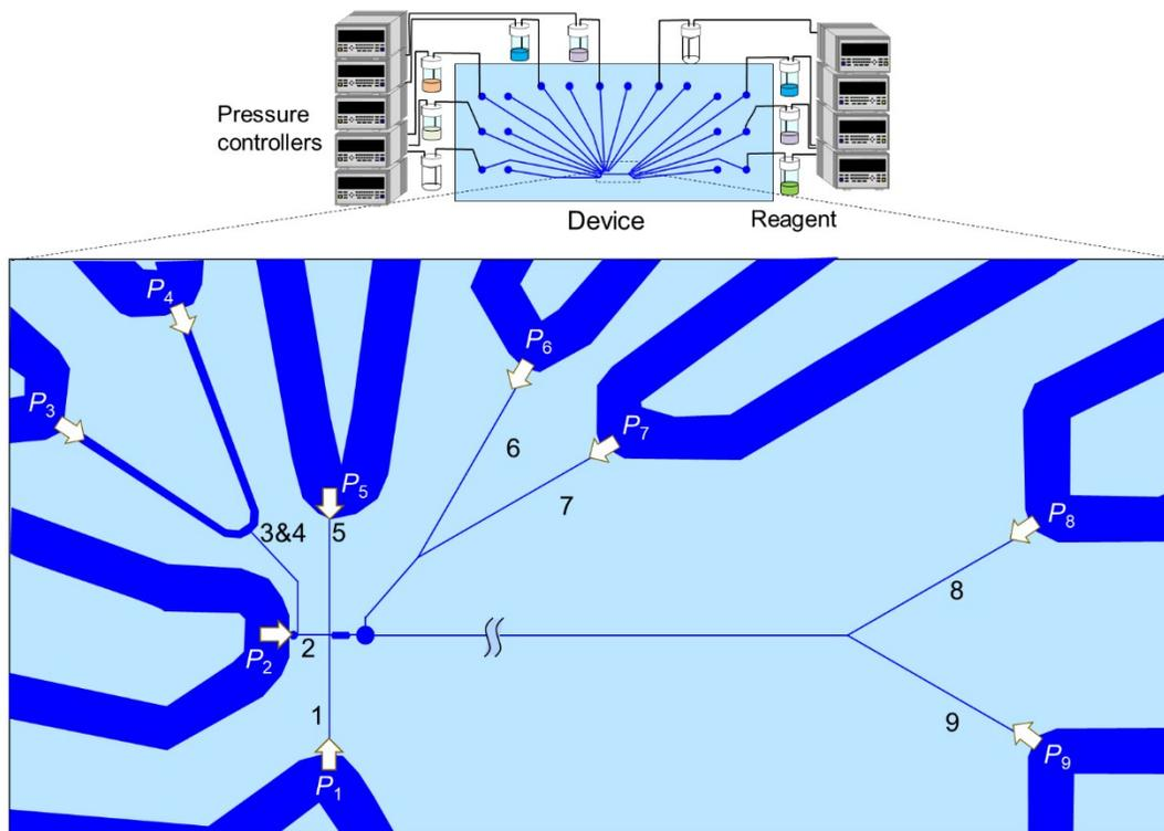
**Figure S2.** Layout of nanochannels and application of external pressure in the micro/nano-integrated fluidic device.
