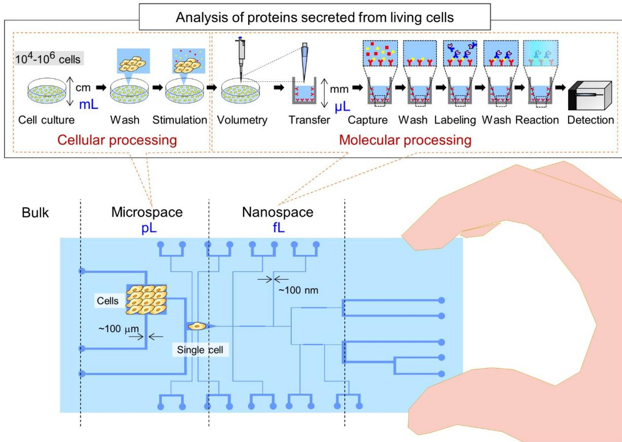
**Figure S1.** Schematic illustration of the concept of the micro/nano-integrated fluidic device for living single-cell protein analysis by comprehensive integration of cellular processing into microspaces (pL scale) and molecular processing into nanospaces (fL scale).
