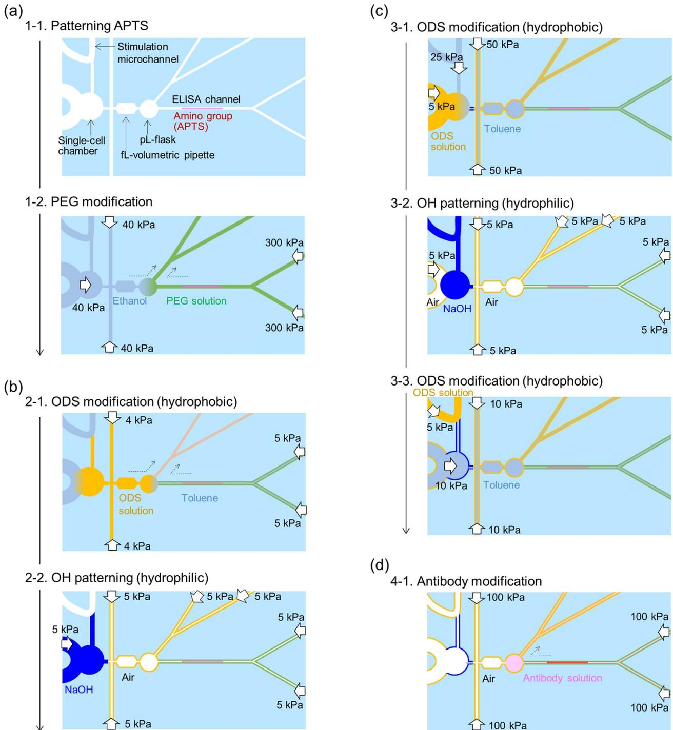
**Figure S5.** Procedure for surface modification of the micro/nano-integrated fluidic device: (a) Step 1. Pre-modification of the ELISA channel with scaffolding for antibody and blocking. (b) Step 2. Hydrophobic/hydrophilic-patterning of the fL-volumetric pipette. (c) Step 3. Hydrophobic/hydrophilic-patterning of the single-cell chamber. (d) Step 4. Modification of the ELISA channel with capture antibody.
