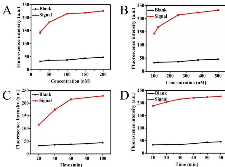
Fig. S1 Optimizations of experimental parameters: (A) concentrations of complex, (B) concentrations of S, (C) ESDRs interaction time, and (D) DNAzyme cleavage time.
