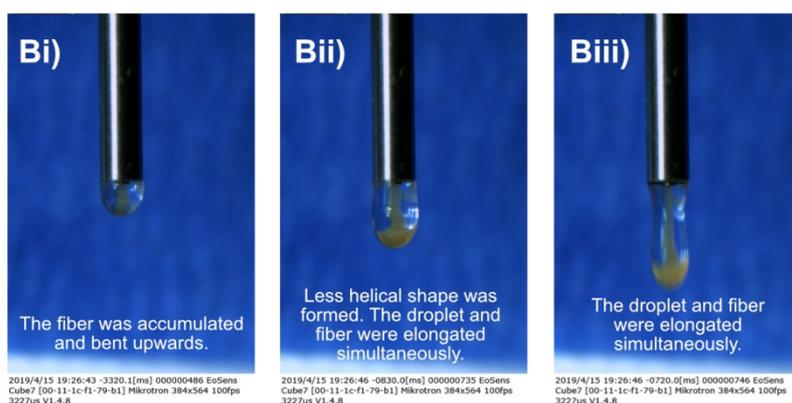
**Figure S2. The Images of Different Fabricating Stages.** The inner flowrate was 20  $\mu$ L/min. The out flowrate was 50  $\mu$ L/min. A) Without voltage. B) With high voltage (4.6kV).
