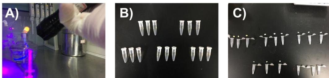
**Figure S4. The Testing of Degradation Profile of the Materials.** A) The fabrication of the tested samples. B) The samples immersed in the 1.5ml centrifugal tubes with 1ml DPBS containing 2U/ml collagenase II. C) The treated samples after freeze-dried process whose masses were weighed by the balance.
