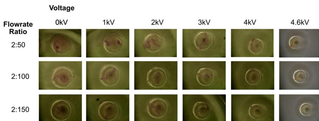
Figure S7. Images of the Structures Fabricated with Different Parameters.
