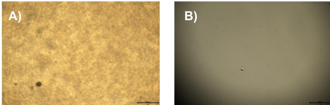
**Figure S3. Optical Morphology of the Materials.** A) The crosslinked 5% GelMA with 1% uncrosslinked sodium alginate. B) the pure crosslinked 5% GelMA.
