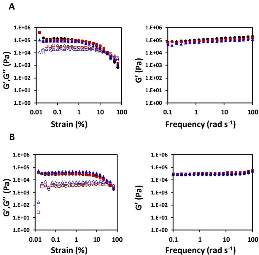
**Figure S13.** Amplitude (left column) and frequency sweeps (right column) recorded for bulk ALG/HA-SH:2<sub>1A</sub> click-hydrogels (2.5 wt%, 75:25 thiol:yne) prepared with the optimized alginate concentration and cross-linking parameters: A) as prepared and B) after being immersed in cell culture media at 37 °C for four days ( $n = 3$  samples for each system).
