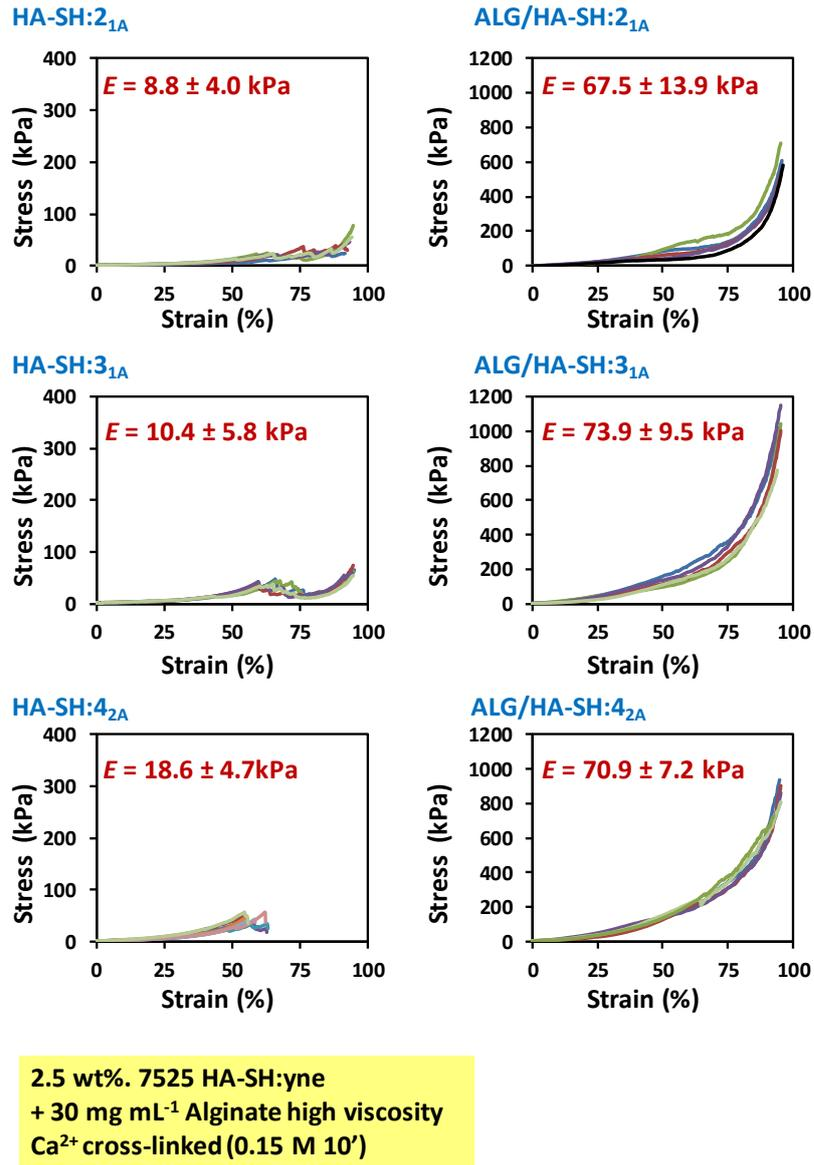
**Figure S9.** Representative compressive stress-strain curves recorded for HA-SH:yne (left column) and ALG/HA-SH:yne (right column) click-hydrogels prepared with the optimized alginate concentration and cross-linking parameters. Each graph displays the mean Young's moduli determined from the linear range of the curve (below 10% strain).
