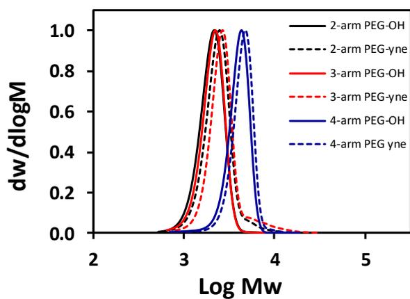
**Figure S5.** SEC chromatograms of alkyne-terminated PEG precursors (dashed lines) and starting PEG materials (solid lines). Molecular weight determined against poly(methyl methacrylate) using DMF (5 mM NH<sub>4</sub>BF<sub>4</sub>) as eluent.
