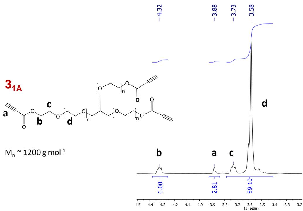
**Figure S3.**  $^1\text{H}$  NMR spectrum of yne-terminated 3-arm PEG ( $3_{1A}$ ,  $1 \text{ kg mol}^{-1}$ ) in  $d_6$ -acetone (300 MHz, 298 K).
