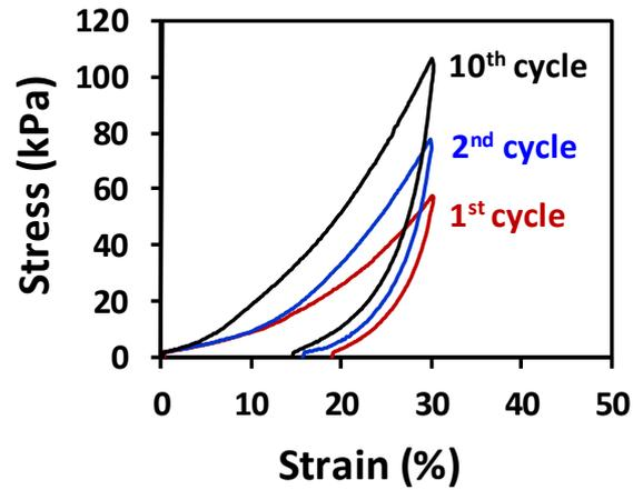
**Figure S12.** Representative compressive cyclic stress-strain curves of ALG/HA-SH:2<sub>1A</sub> click-hydrogels after being immersed in cell culture media for 4 days.
