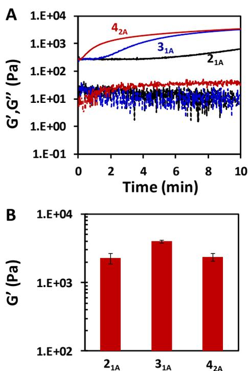
**Figure S10.** A) Representative gelling curves (time sweeps) as monitored by rheometry for HA-SH:yne hydrogels (2.5 wt%. 75:25 SH:yne). Gelation takes place very fast, being  $G' > G''$  since the beginning. B) Mean values of the final storage moduli ( $G'$ ) after 30 minutes.
