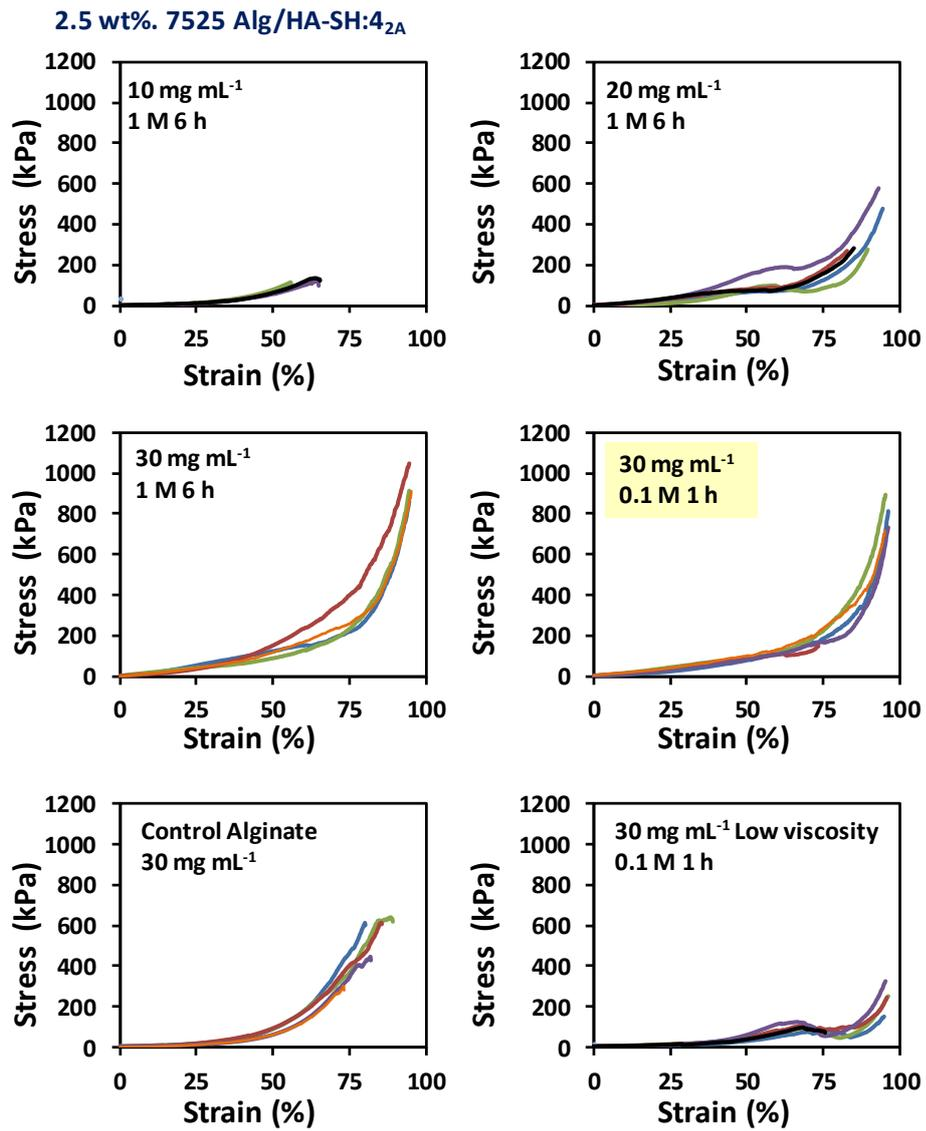
**Figure S8.** Representative compressive stress-strain curves recorded for ALG/HA-SH:4<sub>2A</sub> click-hydrogels prepared with varying amounts of alginate and crosslinking parameters.
