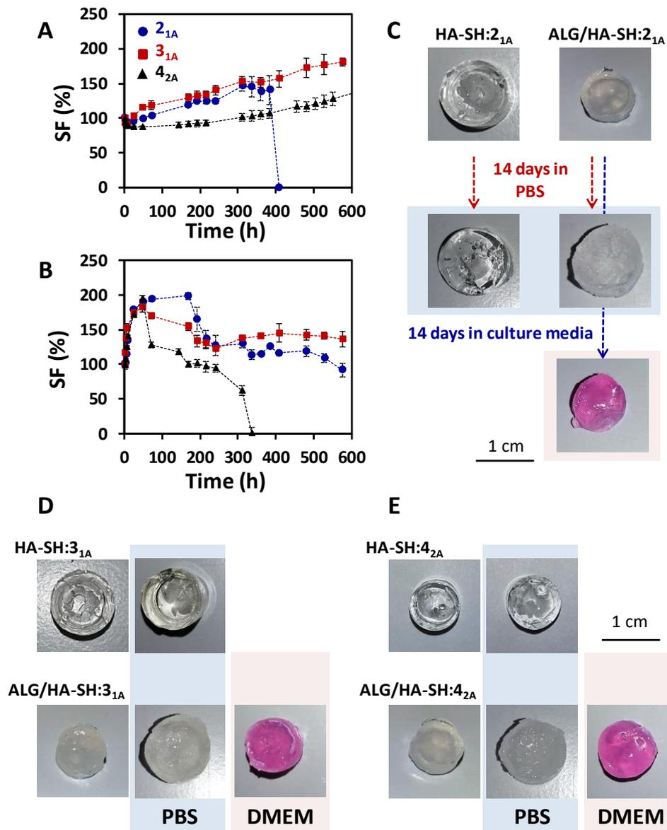
**Figure S7.** Swelling profiles for click-hydrogels immersed in PBS at 37 °C for A) HA-SH:yne (2.5 wt%. 75:25 SH:yne) and B) ALG/HA-SH:yne (2.5 wt%. 75:25 SH:yne). Images taken to show the volume change induced by swelling (14 days of immersion in PBS or cell culture media) for C) HA-SH:2<sub>1A</sub>, D) HA-SH:3<sub>1A</sub> and E) HA-SH:4<sub>2A</sub> with and without alginate.
