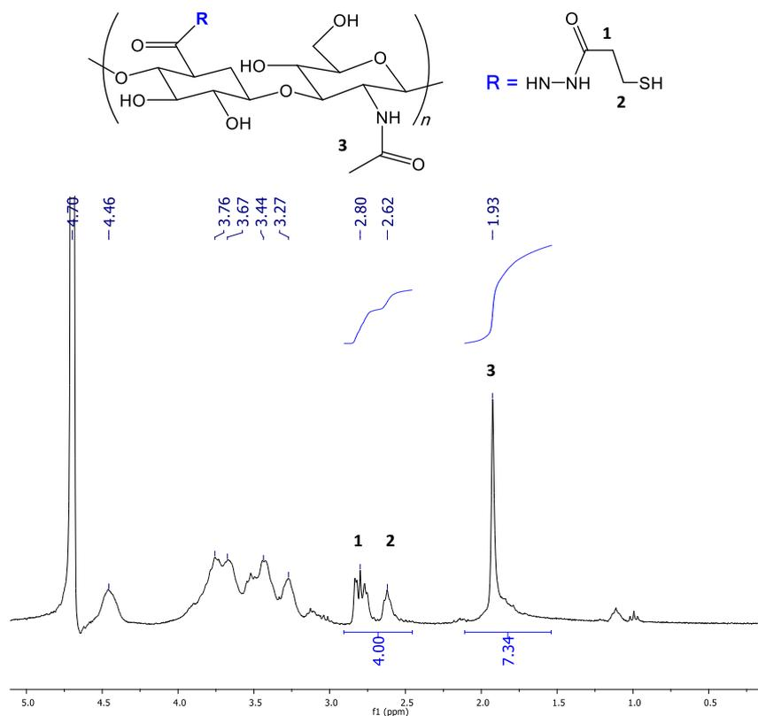
**Figure S1.** <sup>1</sup>H NMR spectrum of HA-SH in deuterated water (300 MHz, 298 K).
