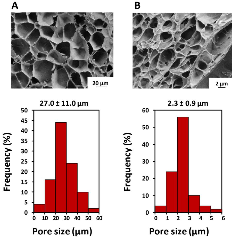
**Figure S14.** Cryo-SEM images taken for A) HA-SH:yne and B) ALG/HA-SH:yne click-hydrogels and pore size distribution determined from the images.
