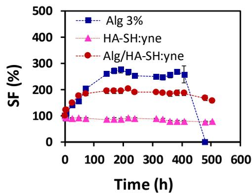
**Figure S15.** Swelling profiles monitored during the optimization stage for click-hydrogels immersed in PBS at 37 °C: HA-SH:2<sub>1A</sub> hydrogels (2.5 wt%) immersed in PBS + 0.1 M Ca<sup>2+</sup> to check the role played by the cross-linking cation.
