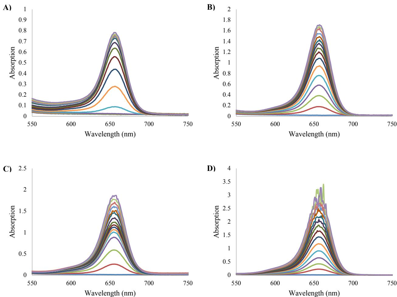
**Figure S1.** UV-Vis absorption spectra of titrations performed on a  $1.5 \times 10^{-3}$  M solution of **3b** in DMSO with **A)**  $\text{Rh}(\text{PPh}_3)_3\text{Cl}$ , **B)**  $\text{Pd}(\text{OAc})_2$ , **C)**  $[\text{Ir}(\text{cod})\text{Cl}]_2$ , and **D)**  $\text{Au}(\text{PPh}_3)\text{Cl}$ . Absorbance of regenerated squaraine **2b** measured at 656 nm.
