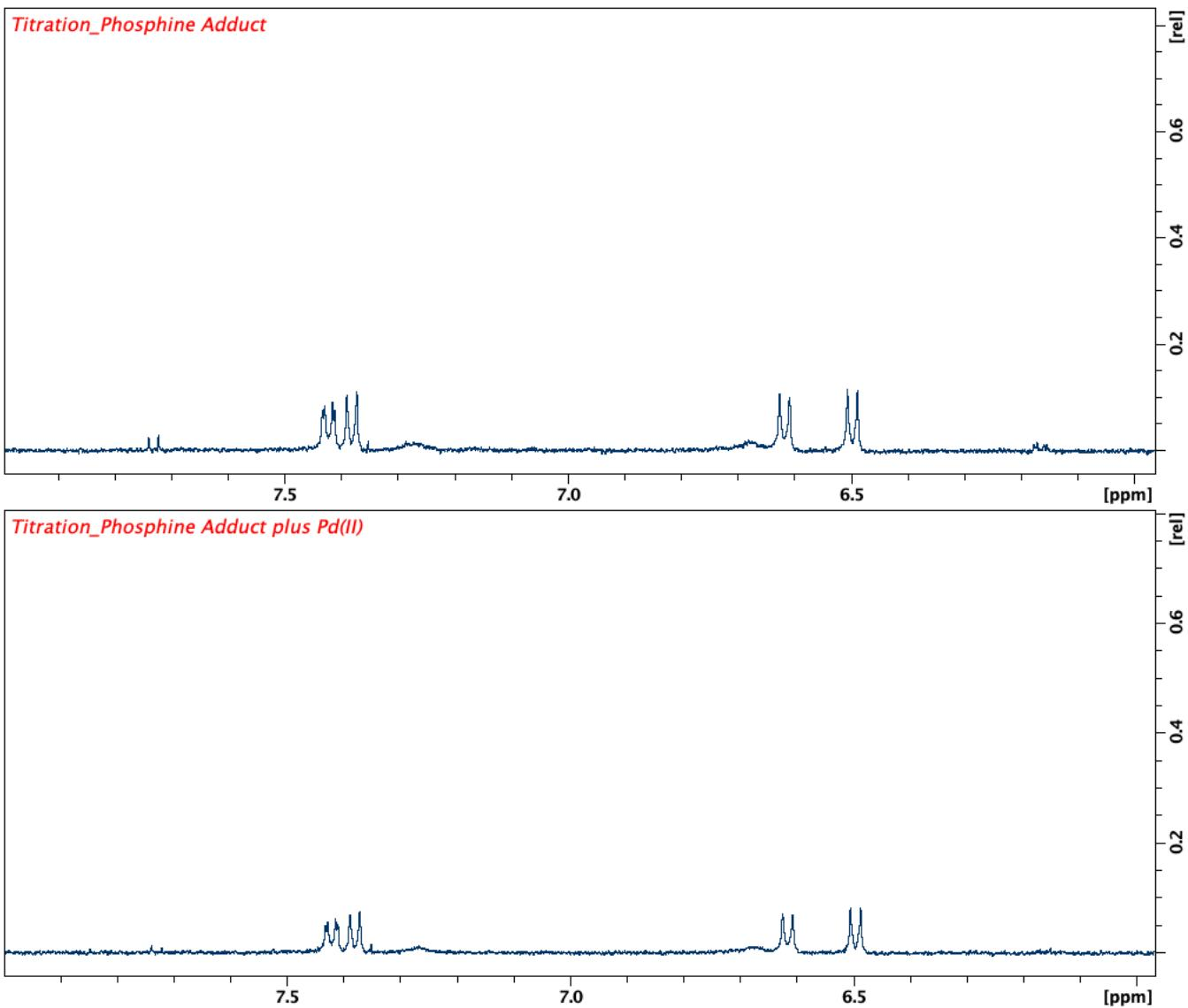
**Figure S2.** <sup>1</sup>H NMR spectra of a  $1.5 \times 10^{-3}$  M solution of **3b** in DMSO before (top) and after (bottom) addition of 1.5 molar equivalents of Pd(OAc)<sub>2</sub>.
