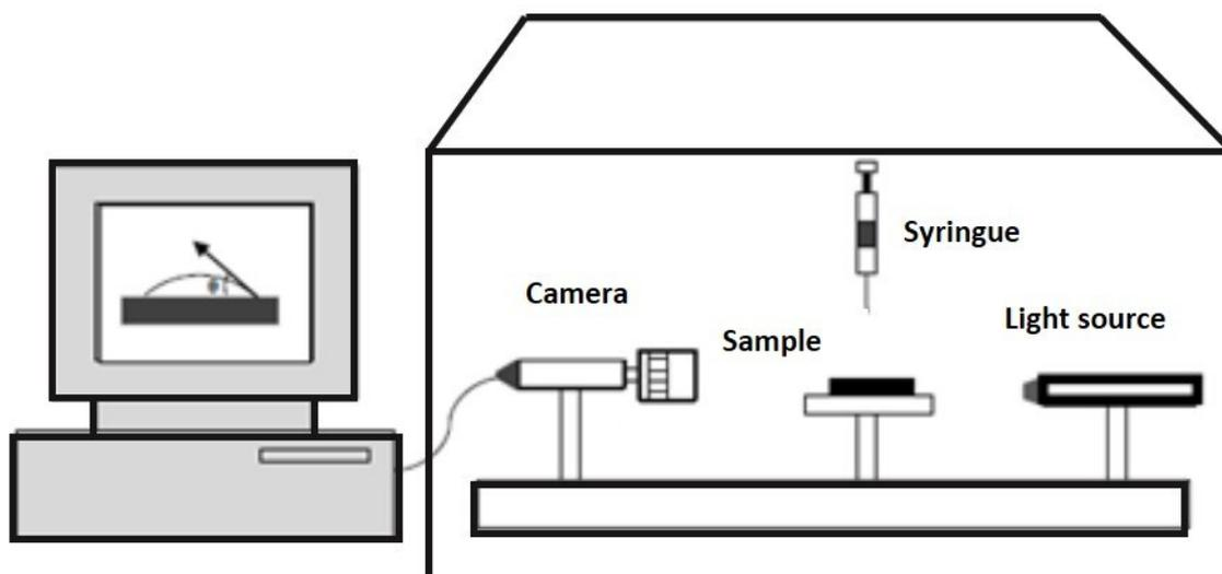
**Fig. S6:** Schematic illustration of the contact angle measuring device
