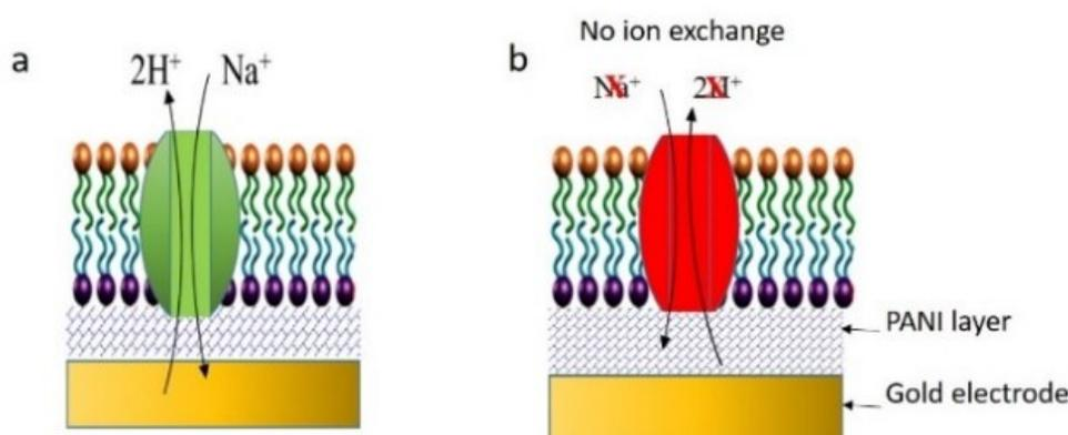
**Fig. S1.** Principle of Ion-co-transport for the NhaA membrane protein incorporated in the SLB. (a) For the **active** protein, there is an electrogenic ion current established across the lipid bilayer membrane due to the exchange of 2 H<sup>+</sup> ions for 1 Na<sup>+</sup> ion. (b) For the **inactive** mutated protein (see ESI), there is no ion transport.
