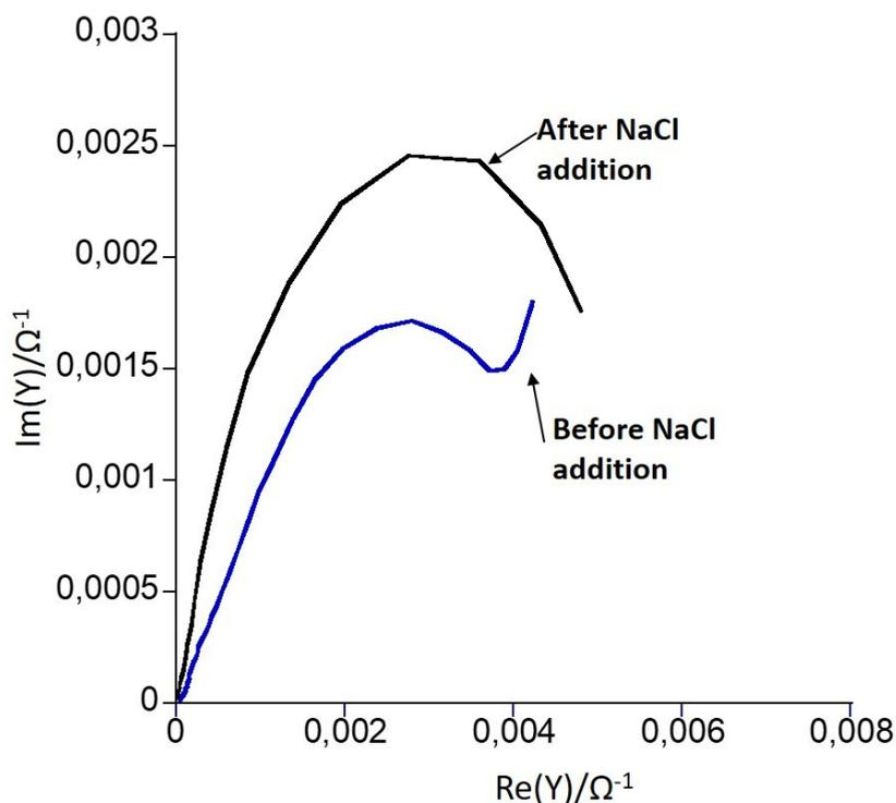
**Fig. S4.** The same data from Fig. 4 for the electrochemical impedance spectroscopy response (Cole-Cole diagram) of SLB-*inactive-NhaA*-PANI modified gold electrode before and the after the addition of NaCl 10 mM. The scale is reduced for better visibility of the differences before and after the addition of NaCl. Although the difference appears to be large at this scale, it is important to note that the inactive *NhaA* protein did not respond to addition of NaCl.
