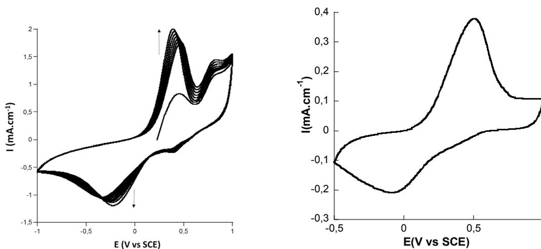
**Fig. S3.** *Left*, Consecutive cyclic voltammograms for electro polymerization of aniline obtained on gold electrode in PBS (pH 7) containing 2 mM of aniline, scan rate 10 mV/s. **Right**, cyclic voltammetry of PANI modified gold electrode in PBS (pH7), scan rate 10mV/s.
