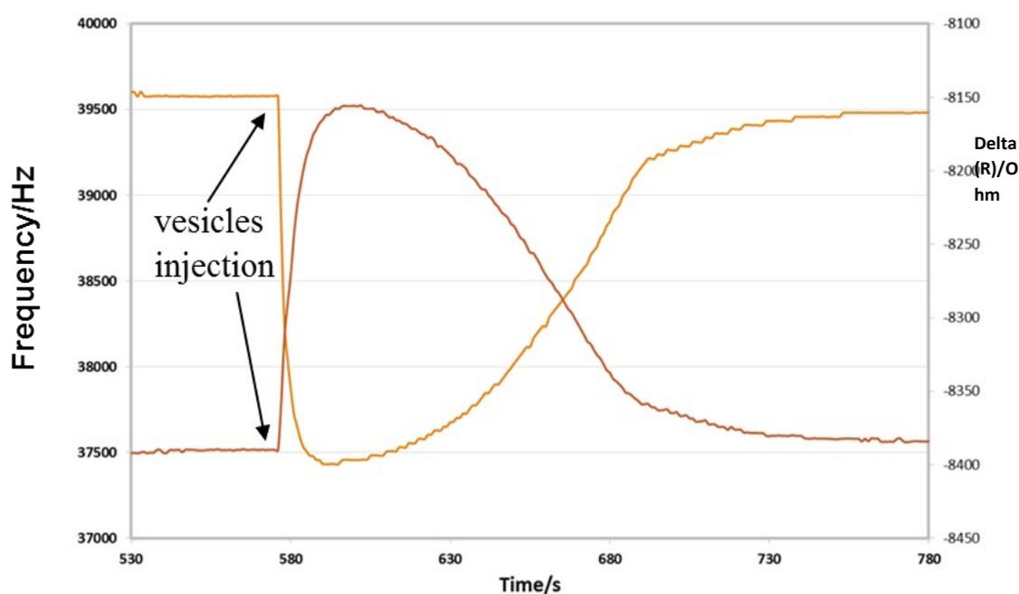
**Fig. S2.** QCM-D responses for PANI modified gold electrode before and after vesicle injection. The orange line shows the resonance frequency and the red line shows the change in dissipation. After the vesicles were injected (580 s) there was a diminution in the resonant frequency and a concomitant increase in the dissipation. After approximately 200 s both the resonant frequency and dissipation reached steady-state levels which were close to the initial values.
