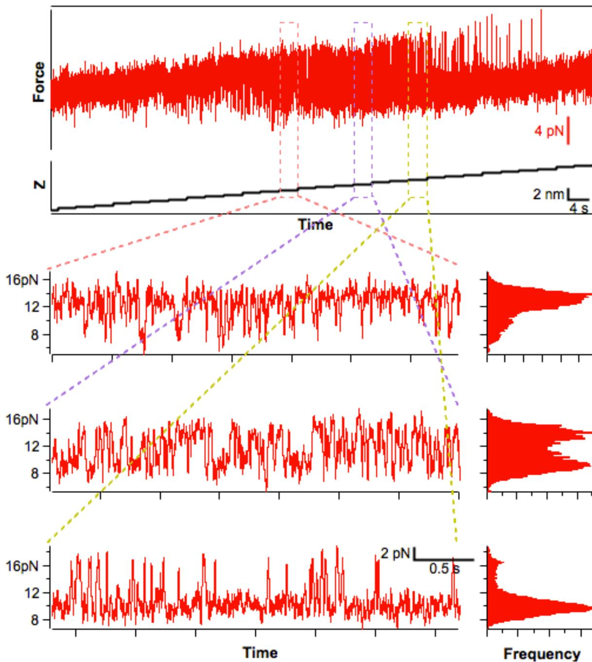
**Figure S3.** Constant separation trace from Fig 2. Insets show zoomed in regions of different fixed stage positions demonstrating the effect of stretching on GA folding/unfolding equilibrium. At low extensions, GA favours the folded state (top). As the extension increases, the unfolded state becomes increasingly populated (middle, bottom).
