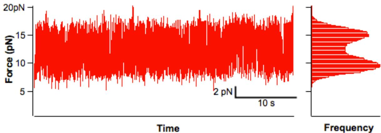
**Figure S2.** Constant separation experiment of GA demonstrating stability at a fixed stage position over ~40 seconds. Right: population distribution of folded (higher force) and unfolded (lower force) states.
