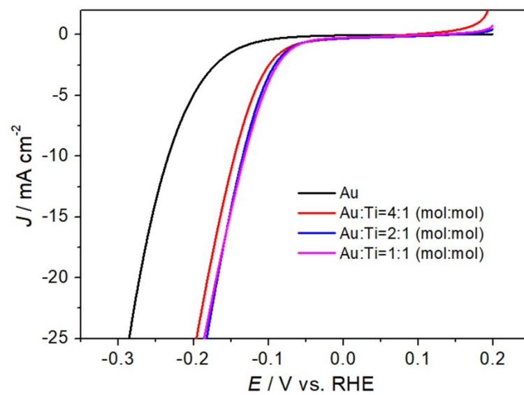
Figure S6 The HER activities of AuTiO<sub>2-x</sub> electrodes with different calcination temperatures and Au-Ti mole ratios.
