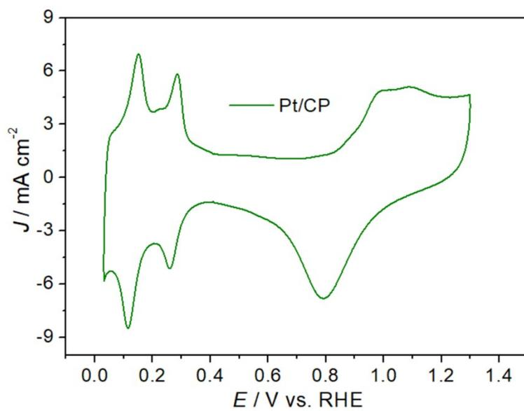
Figure S5 The cyclic voltammogram (CV) of the Pt electrode.
