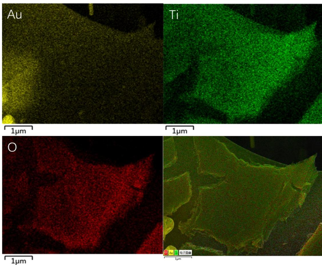
Figure S2 SEM-EDS elemental maps (Au, Ti and O) of AuTiO<sub>2-x</sub> nanoparticles.
