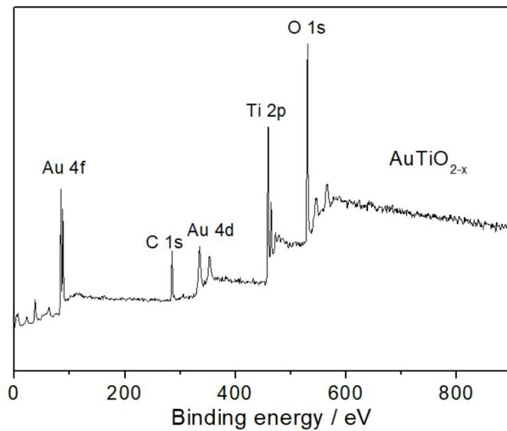
Figure S4 The XPS survey spectrum of AuTiO<sub>2-x</sub> electrodes.
