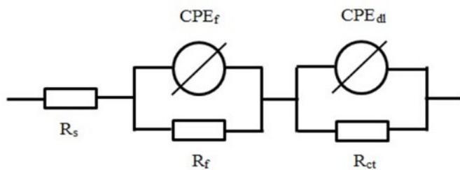
Figure S8 The equivalent circuit of the impedance of  $AuTiO_{2-x}$  and Au electrodes
