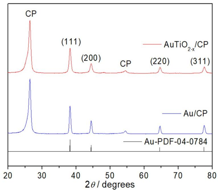
Figure S3 XRD images of Au and AuTiO<sub>2-x</sub> nanoparticles.
