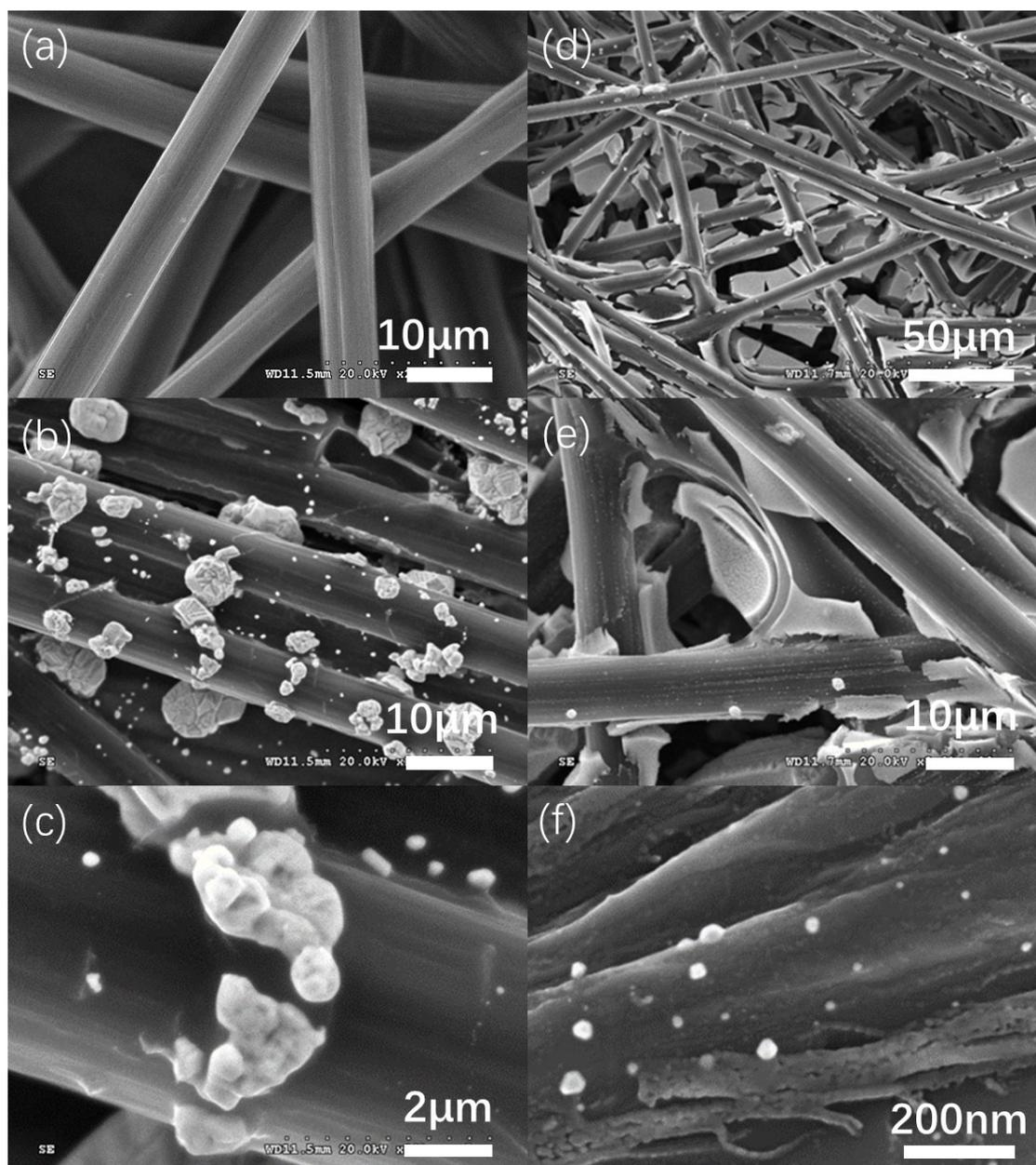
Figure S1 SEM images of CP (a), Au/CP (b, c) and AuTiO<sub>2-x</sub>/CP (d-f).
