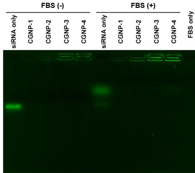
**Fig. S3** Agarose gel electrophoresis of siRNA and CGNP-siRNA with or without FBS treatment (37 °C, 4h). The siRNA-FAM was used to visualize its integrity by fluorescent imaging.
