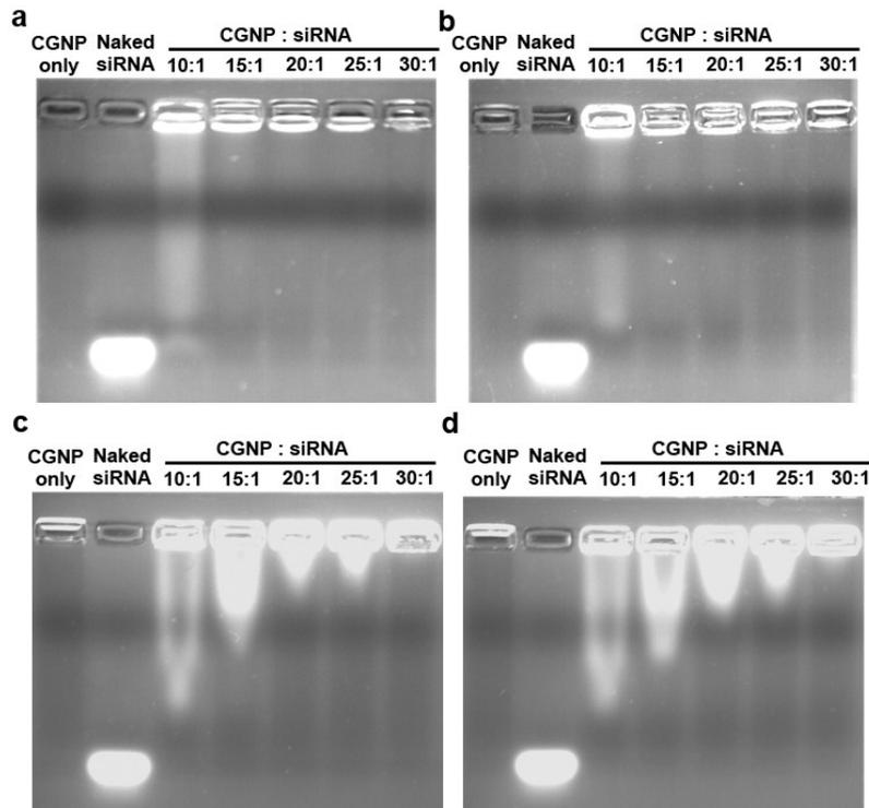
**Fig. S2** CGNP's binding with siRNA determined by agarose gel electrophoresis. (a) CGNP-1. (b) CGNP-2. (c) CGNP-3. (d) CGNP-4. CGNP:siRNA represents the weight ratio of CGNP to siRNA.
