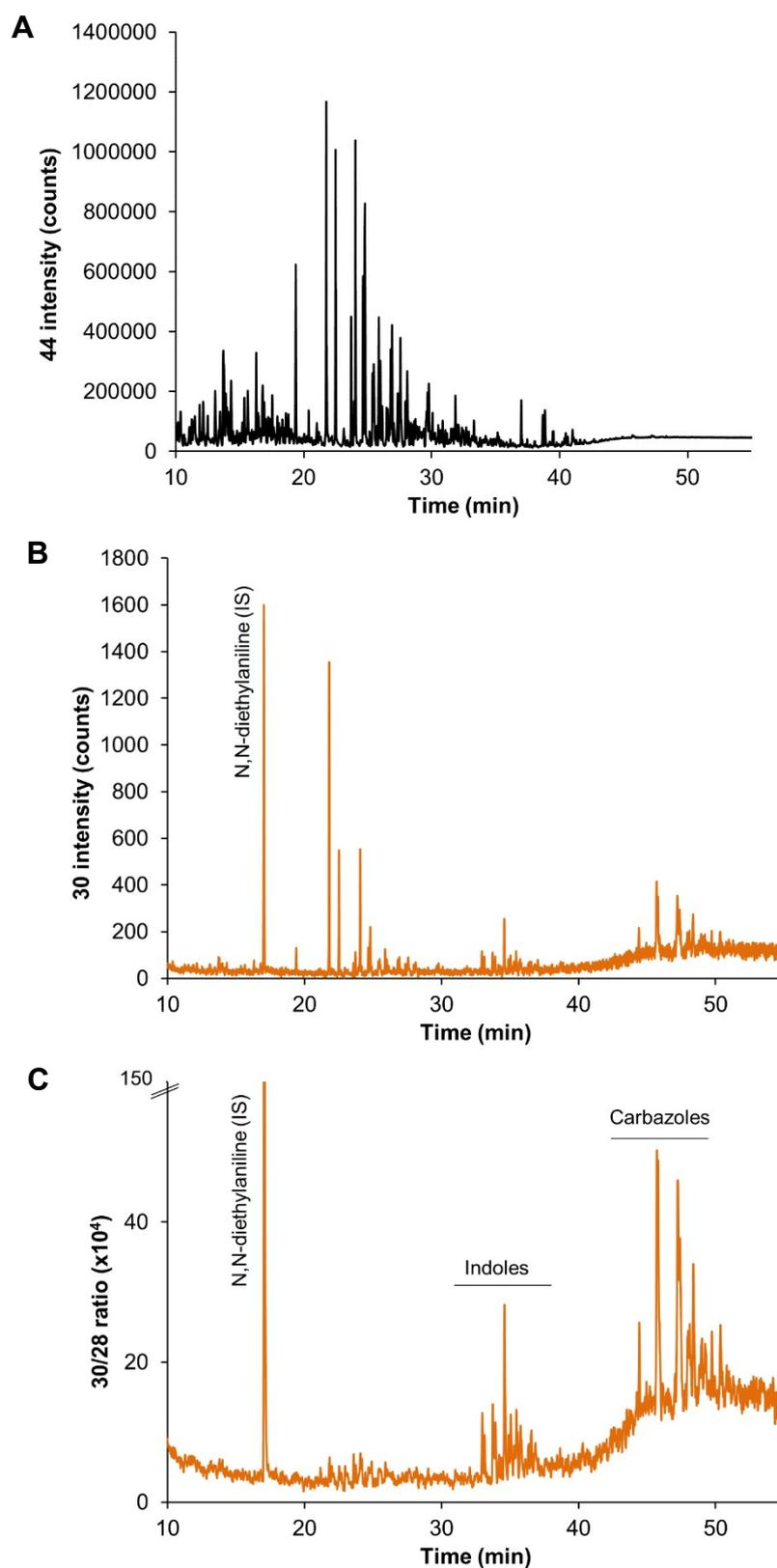
**Figure S18.** Chromatogram for the diesel sample (ca. 400  $\mu\text{g N g}^{-1}$ ) diluted 1:500 with the internal standard (N,N-diethylaniline, 0.25  $\mu\text{g N g}^{-1}$ ) A) m/z 44, B) m/z 30 (not corrected for  $^{12}\text{C}^{18}\text{O}$  contribution), C) complete N-selective 30/28 profile (corrected for the unspecific  $^{12}\text{C}^{18}\text{O}$  contribution, see Fig S13)
