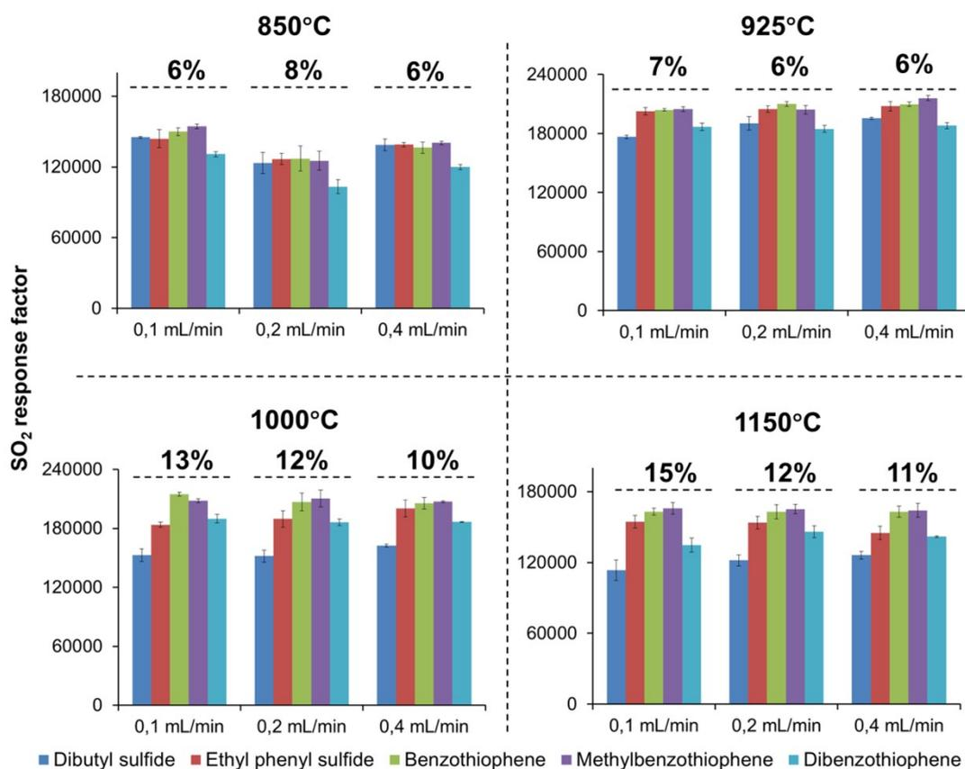
**Figure S15.** SO<sub>2</sub> response factors (peak area at m/z 64 divided by the S concentration in the corresponding compound) obtained for the mixture of S-containing compounds (2 μg S g<sup>-1</sup>) at different temperatures (ranging from 850 to 1150°C) and O<sub>2</sub>/He flows (0.1-0.4 mLmin<sup>-1</sup>). Error bars indicate 1 SD (n=3). RSD of the different response factors obtained for the mixture of compounds under the different conditions assayed are given.
