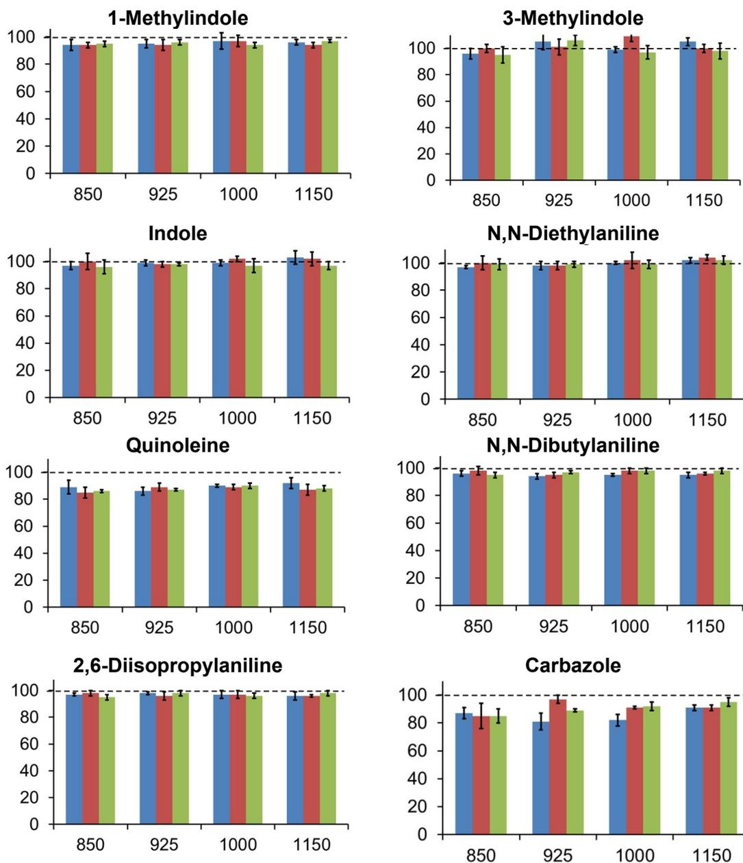
**Figure S9.** H<sub>2</sub>O recoveries (m/z 18) for N-containing compounds at different temperatures (850-1150°C) and 0.1, 0.2 and 0.4 mLmin<sup>-1</sup> O<sub>2</sub>/He (blue, red and green bars, respectively) using pentadecane as internal standard. Error bars indicate 1 SD (n=3).
