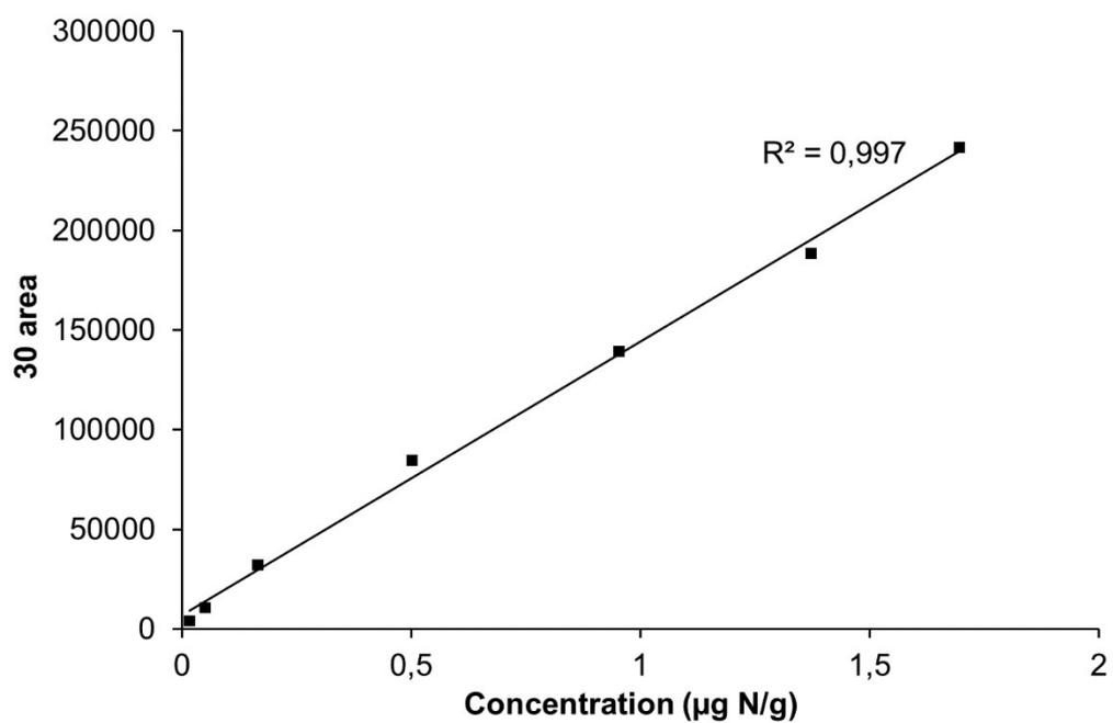
**Figure S13.** Linearity for indole from 0.016 to 1.7 µg N g<sup>-1</sup> using 1150°C and 0.4 mLmin<sup>-1</sup> O<sub>2</sub>/He.
