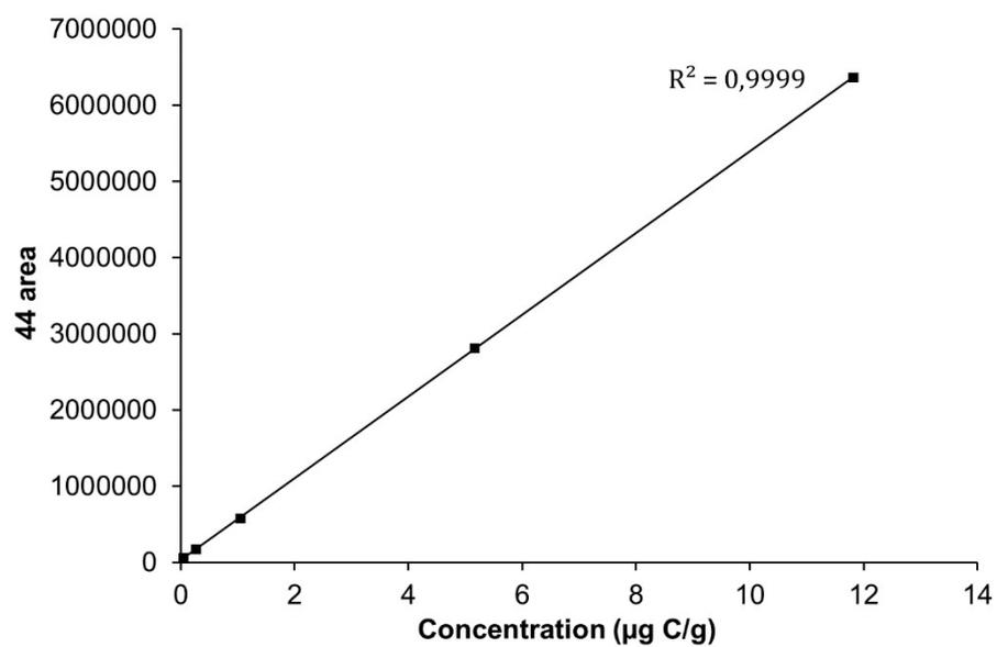
**Figure S7.** Linearity for acenaphthene from 0.050 to 12 µg C g<sup>-1</sup> using 925°C and 0.4 mLmin<sup>-1</sup> O<sub>2</sub>/He.
