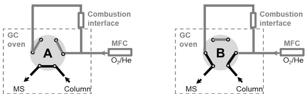
**Figure S2.** Diagram of the GC-combustion-MS setup with the two valve configurations: A) GC-MS conventional mode (structural elucidation) and B) GC-combustion-MS mode: C-, H-, N-, S-selective generic quantification.
