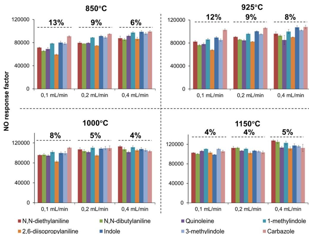
**Figure S16.** NO response factors (peak area at  $m/z$  30 divided by the N concentration in the corresponding compound) obtained for the mixture of N-containing compounds ( $1 \mu\text{g N g}^{-1}$ ) at different temperatures (ranging from 850 to 1150°C) and  $\text{O}_2/\text{He}$  flows (0.1-0.4  $\text{mL min}^{-1}$ ). Error bars indicate 1 SD (n=3). RSD of the different response factors obtained for the mixture of compounds under the different conditions assayed are given.
