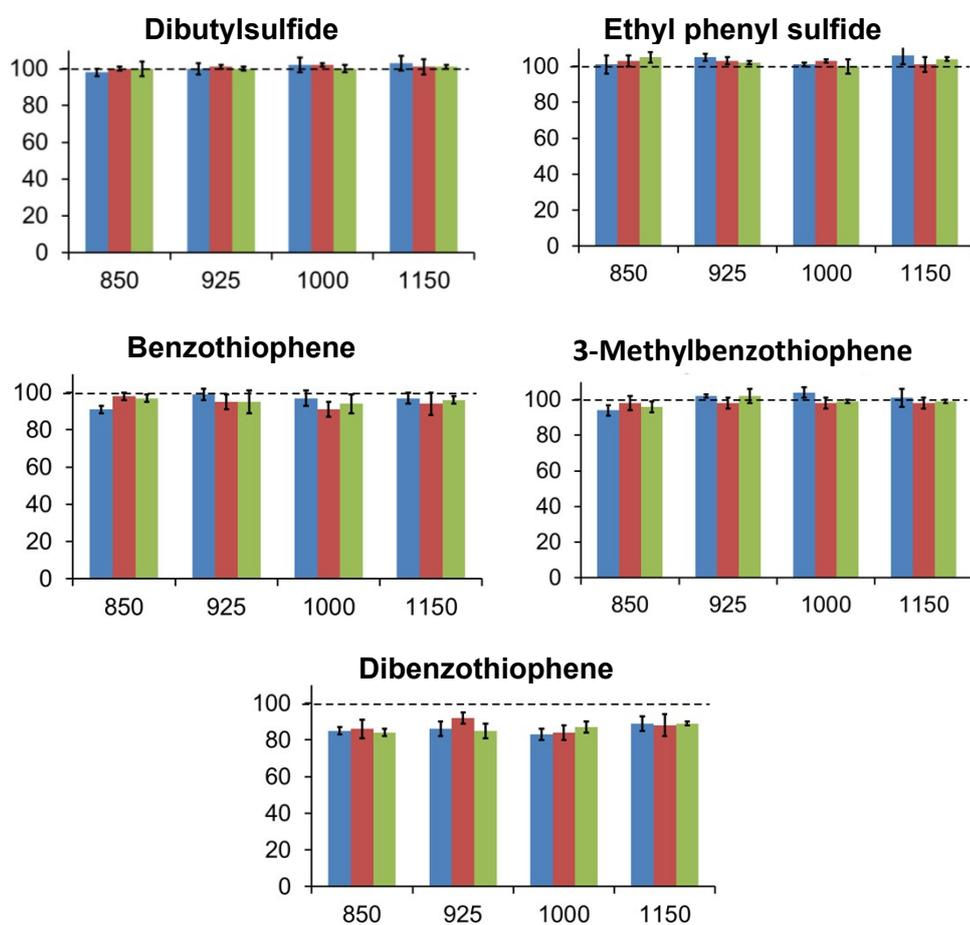
**Figure S8.** H<sub>2</sub>O recoveries (*m/z* 18) for S-containing compounds at different temperatures (850-1150°C) and 0.1, 0.2 and 0.4 mLmin<sup>-1</sup> O<sub>2</sub>/He (blue, red and green bars, respectively) using tetradecane as internal standard. Error bars indicate 1 SD (n=3).
