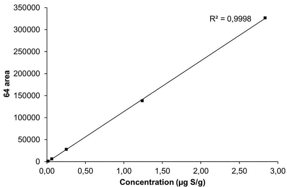
**Figure S12.** Linearity for 3-Methylbenzothiophene from 0.013 to 2.8 µg S g<sup>-1</sup> using 925°C and 0.4 mLmin<sup>-1</sup> O<sub>2</sub>/He.
