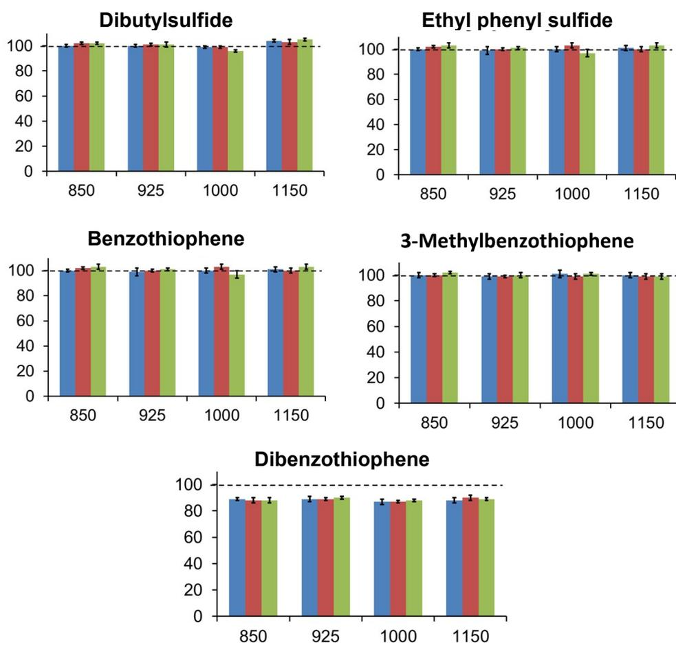
**Figure S5.** CO<sub>2</sub> recoveries (m/z 44) for S-containing compounds at different temperatures (850-1150°C) and 0.1, 0.2 and 0.4 mLmin<sup>-1</sup> O<sub>2</sub>/He (blue, red and green bars, respectively) using tetradecane as internal standard. Error bars indicate 1 SD (n=3).
