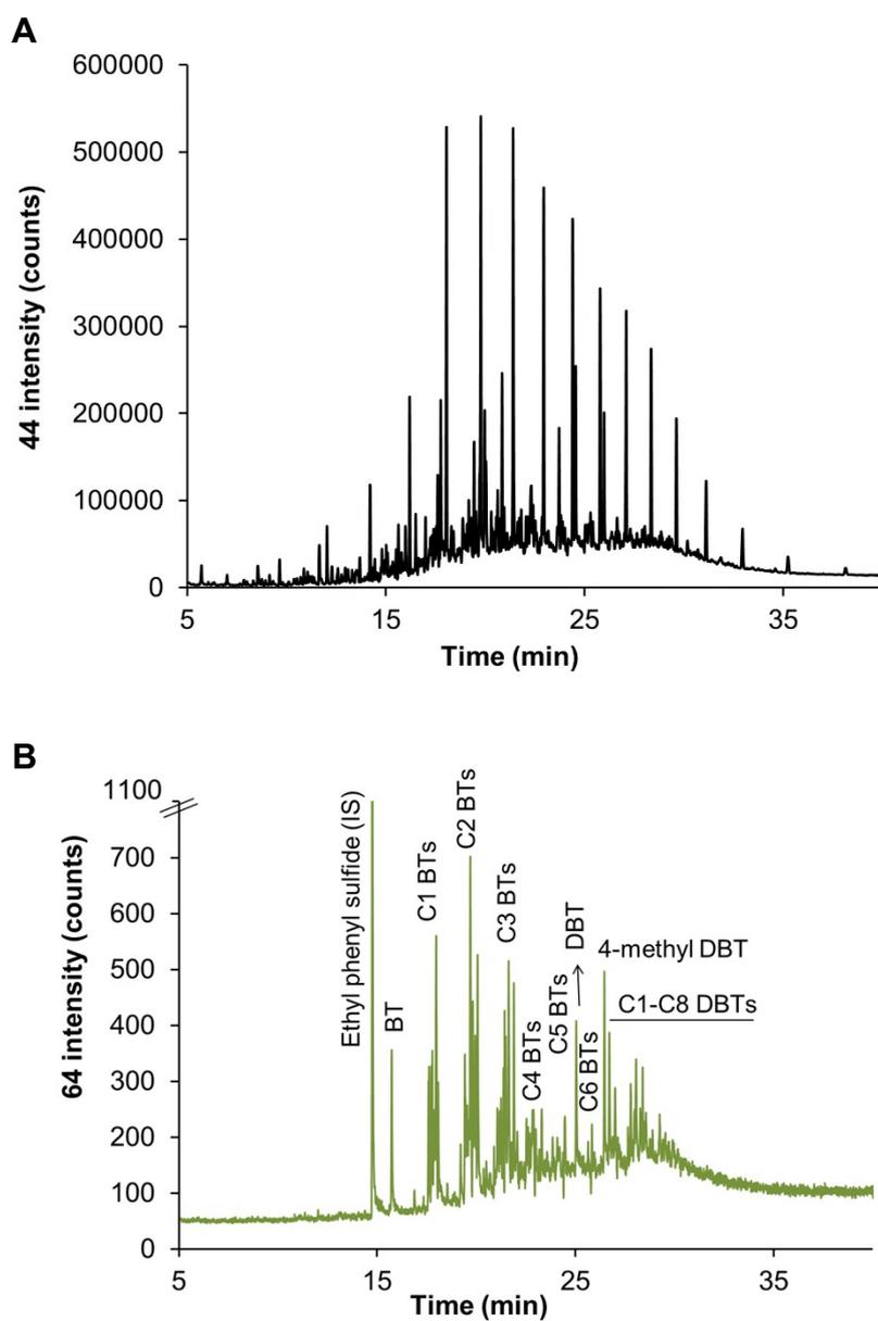
**Figure S17.** Chromatogram for the diesel sample (ca. 4000  $\mu\text{g S g}^{-1}$ ) diluted 1:800 and spiked with ethyl phenyl sulfide as internal standard; A) m/z 44 and B) m/z 64.
