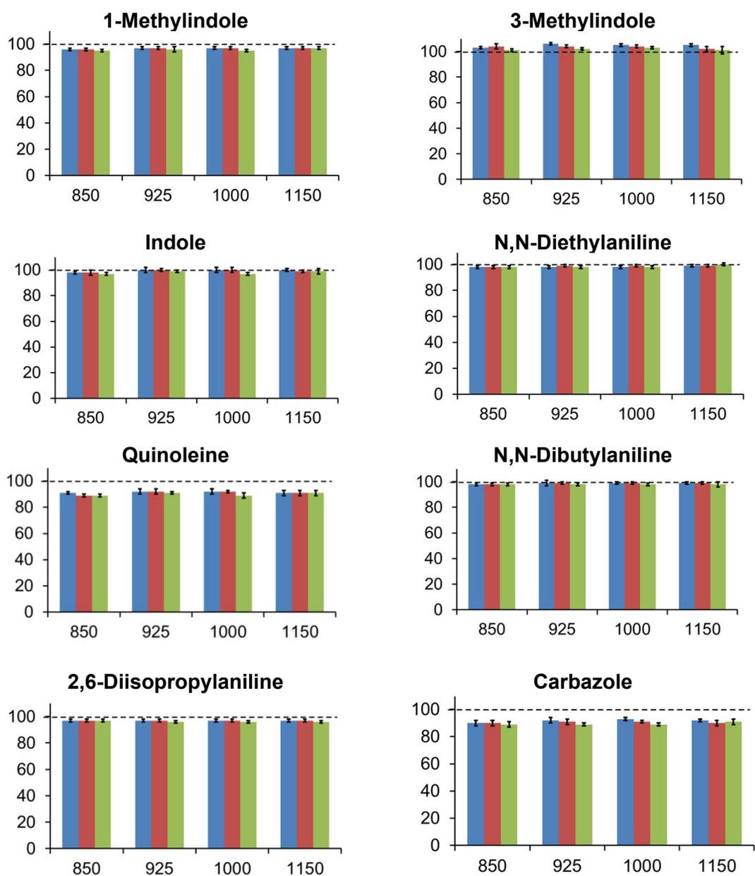
**Figure S6.** CO<sub>2</sub> recoveries (m/z 44) for N-containing compounds at different temperatures (850-1150°C) and 0.1, 0.2 and 0.4 mLmin<sup>-1</sup> O<sub>2</sub>/He (blue, red and green bars, respectively) using pentadecane as internal standard. Error bars indicate 1 SD (n=3).
