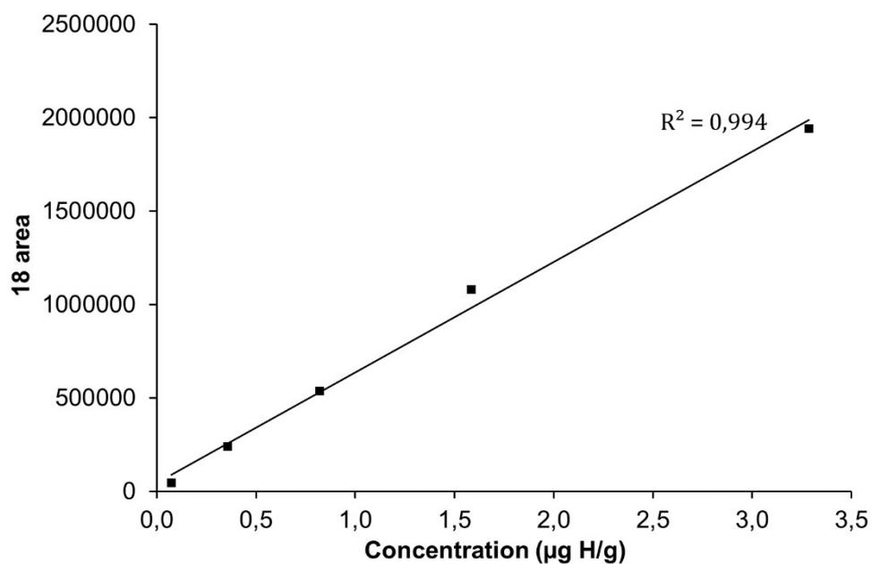
**Figure S10.** Linearity for acenaphthene from 0.020 to 3 µg H g<sup>-1</sup> using 925°C and 0.4 mLmin<sup>-1</sup> O<sub>2</sub>/He.
