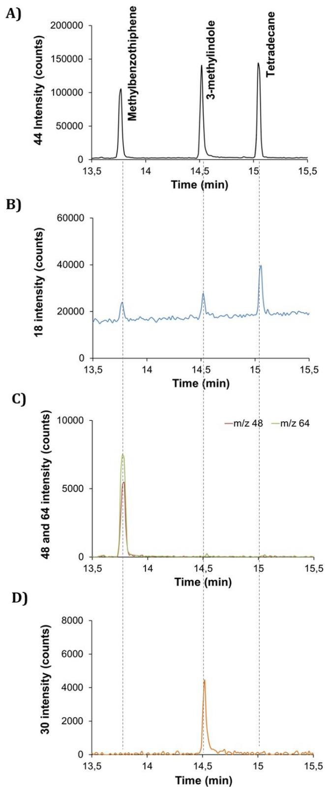
**Figure S3.** GC-combustion-MS chromatogram for A) m/z 44 (CO<sub>2</sub>), B) m/z 18 (H<sub>2</sub>O), C) m/z 48 y 64 (SO and SO<sub>2</sub>) and D) m/z 30 (NO) obtained at 925°C and 0.4 mLmin<sup>-1</sup> O<sub>2</sub>/He for the mixture of 3-Methylbenzothiophene, 3-Methylindole and tetradeceane. Signal to noise ratio is low because the chromatogram was acquired in scan mode (12-300 u) in order to monitor the species combustion and the formation of the corresponding volatile species.
