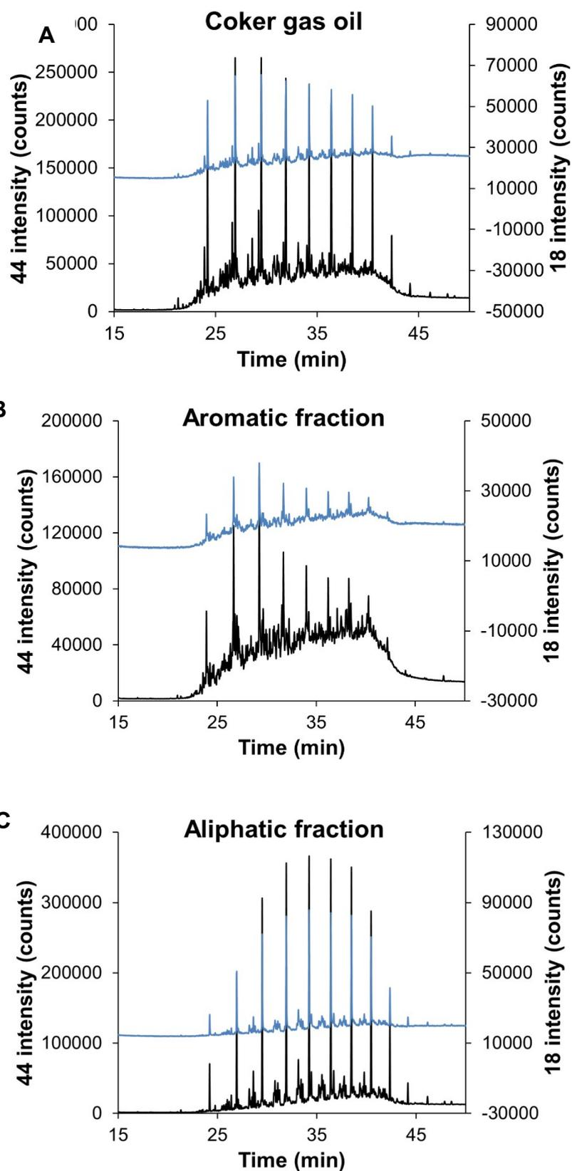
**Figure S19.** Chromatogram for  $m/z$  44 (C, black line) and  $m/z$  18 (H, blue line) for the original coker gas oil sample (A) and its aromatic (B) and aliphatic (C) fractions.
