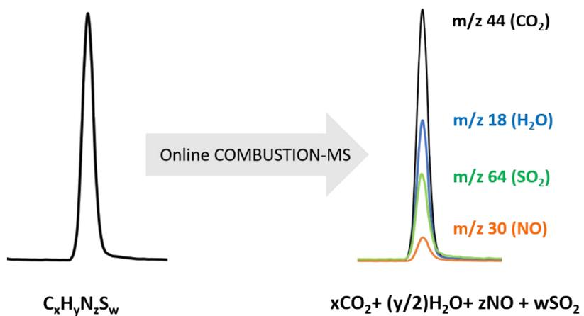
**Figure S1.** Schematic of the process and reactions occurring in the combustion mode to every organic species eluting from the column (left panel). Multiplexed element specific detection and quantification is carried out through the volatile species formed as indicated (right panel).
