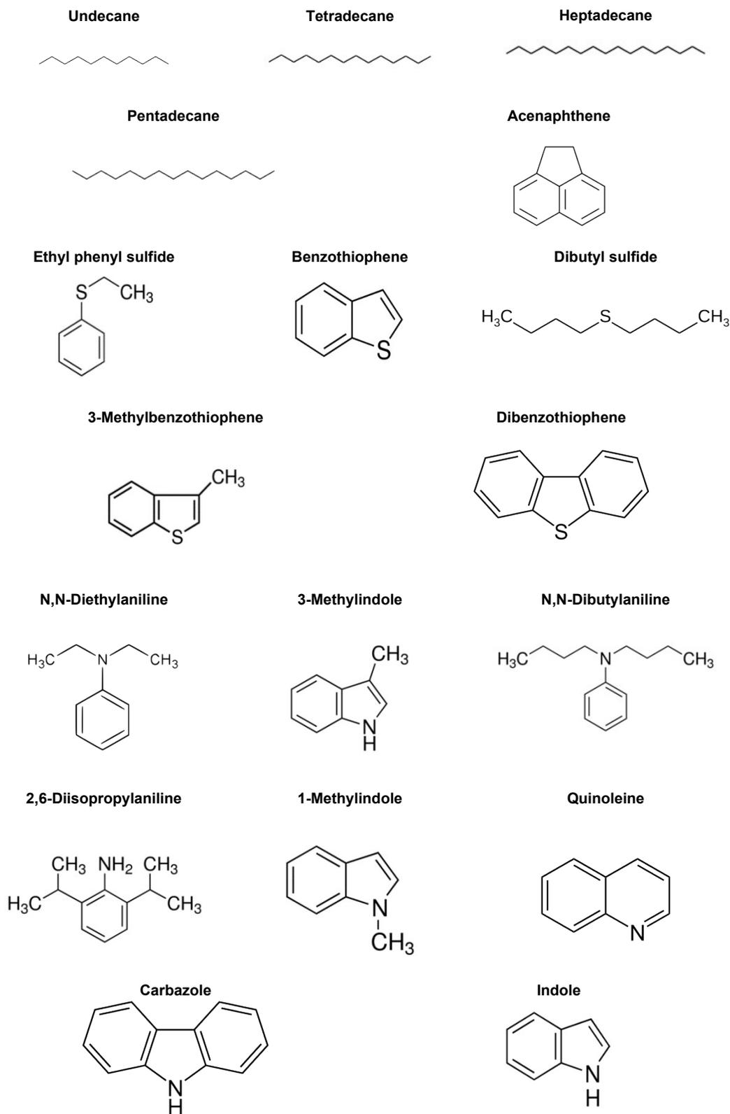
**Figure S4.** Structures of S-, N-containing and organic compounds present in the model mixtures.
