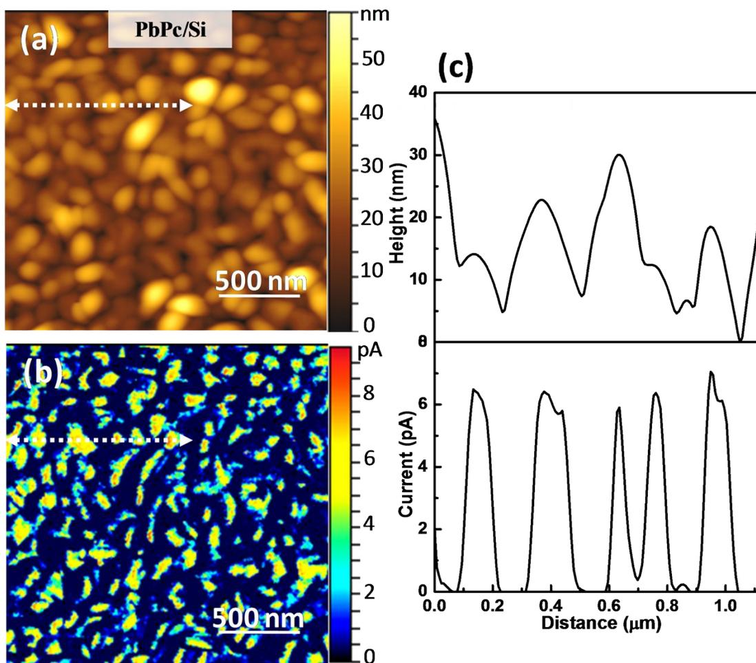
**Figure S9:** (a)  $2\ \mu\text{m} \times 2\ \mu\text{m}$  topography and (b) corresponding current map of pristine PbPc film on Si substrate obtained at 1 V (c) profile sections of (a) and (b) showing the height and current variations across pristine PbPc film on Si substrate.
