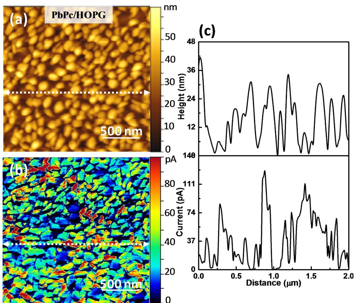
**Figure S10:** (a)  $2\ \mu\text{m} \times 2\ \mu\text{m}$  topography (b) corresponding current map obtained at 1 V for pristine PbPc film on HOPG substrate; (c) profile sections of (a) and (b) showing the height and current variations across pristine PbPc film on HOPG substrate.
