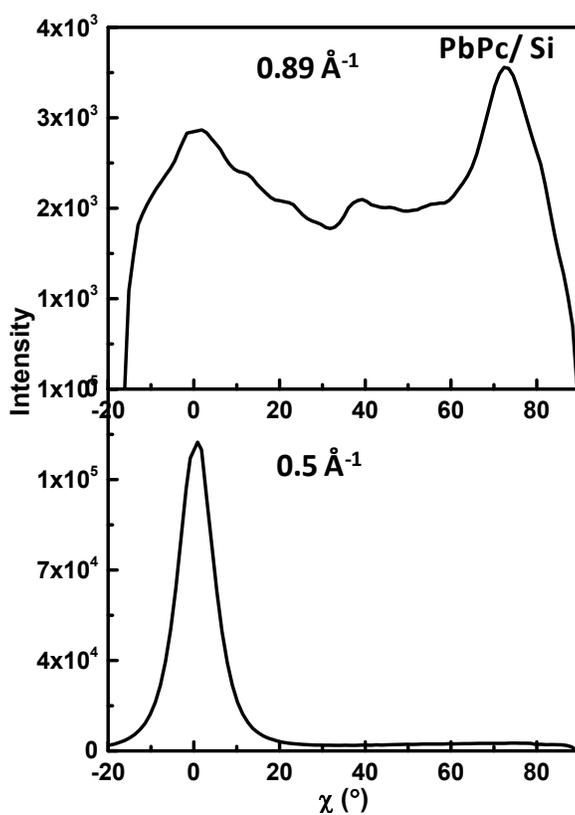
**Figure S1:** Plot of intensity versus azimuthal angles for pristine PbPc film on Si substrate.
