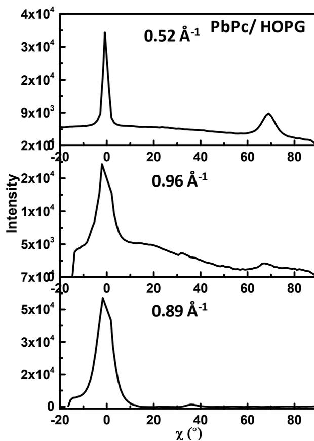
**Figure S2:** Plot of intensity vs. azimuthal angles for pristine PbPc film on HOPG substrate.
