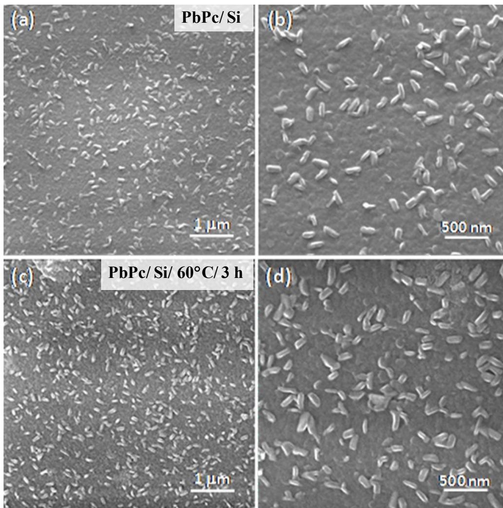
**Figure S7.** (a), (b) FESEM images of as deposited pristine PbPc film on Si substrate and (c), (d) FESEM images of pristine PbPc film on Si substrate after annealing at 60 °C for 3 hours.
