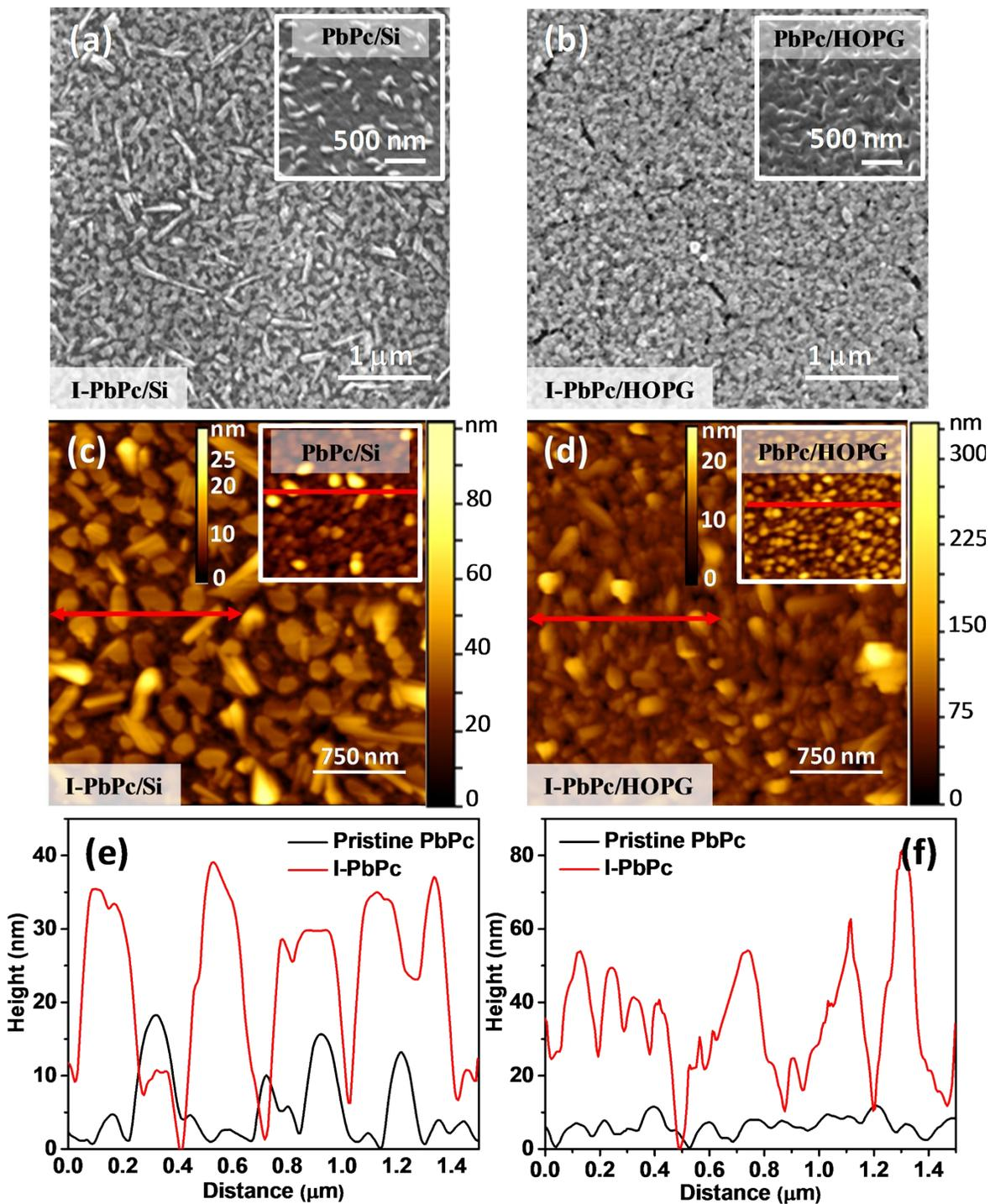
**Figure S6:** (a), (b) FESEM and (c), (d)  $3 \mu\text{m} \times 3 \mu\text{m}$  AFM images of I-PbPc films on Si and HOPG substrates. Insets in (a), (b) are FESEM and (c), (d) are  $1.5 \mu\text{m} \times 1.5 \mu\text{m}$  AFM images of pristine PbPc films on Si and HOPG substrates; (e) and (f) are the profile sections taken across the marked lines in (c) and (d).
