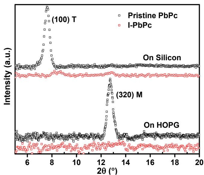
**Figure S3:** XRD patterns of 50 nm pristine PbPc and I-PbPc films deposited on Si and HOPG substrates.
