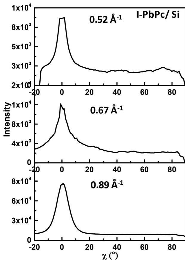
**Figure S4:** Plot of intensity vs. azimuthal angles for pristine I-PbPc film on Si substrate.
