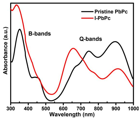
**Figure S5:** UV-Vis absorption spectra of 50 nm pristine PbPc and I-PbPc films obtained on quartz substrates.
