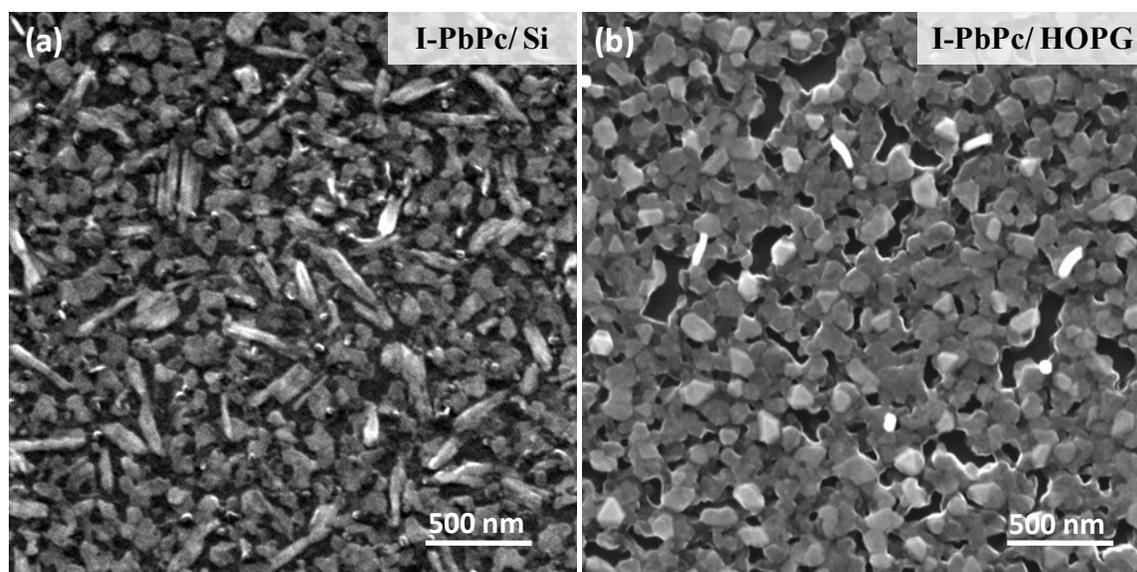
**Figure S8:** FESEM images for I-PbPc films annealed at 100 °C for 1 h in an argon atmosphere on (a) Si and (b) HOPG substrates.
