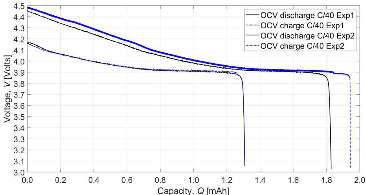
**Fig. S2** Cycling between the voltage limits of 4.2 V - 3.0 V (blue curve: discharge at C/40; red curve: charge at C/40) and 4.5 V - 3.0 V (black curve: discharge at C/40; blue curve: charge at C/40). The offset between the discharge and charge curves is the rest period between the discharge and charge sequence.
