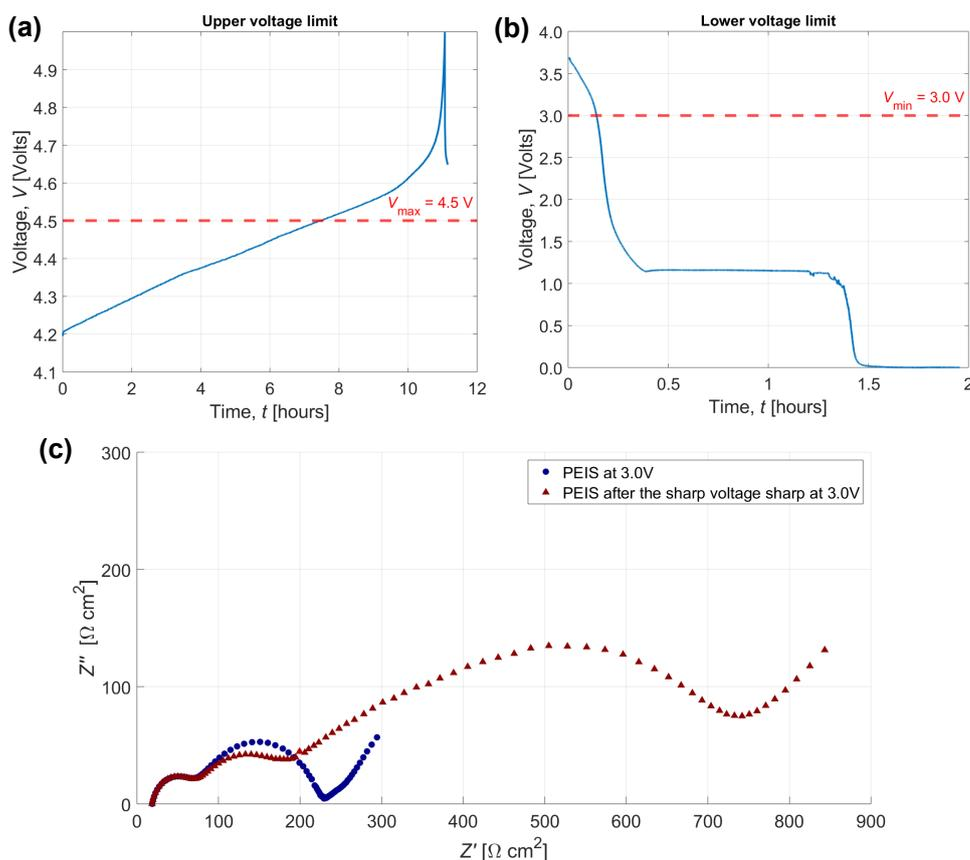
**Fig. S1** Initial overcharge (a) and overdischarge characterisation experiment (b) to estimate the upper and lower voltage limits of the cell, which are used as a basis to estimate the maximum and minimum lithium content in the cell. (c) PEIS impedance measurement at the OCV of 3.0 V and 1.5 V.
