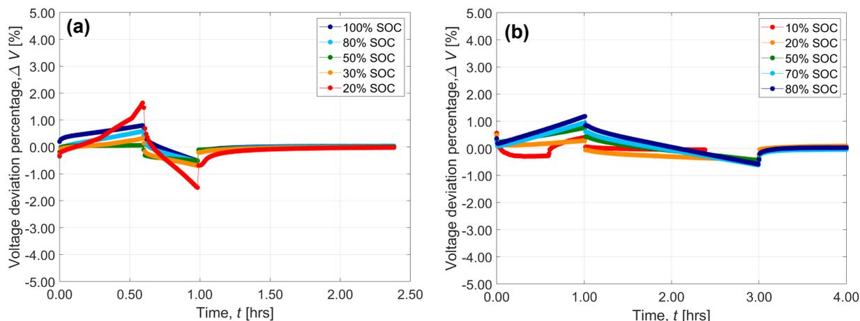
**Fig. S3** The voltage deviations in percentage for the pulse discharge and charge profiles. Both experimental and simulated profiles have a maximum deviation percentage of  $\approx 2\%$ .
