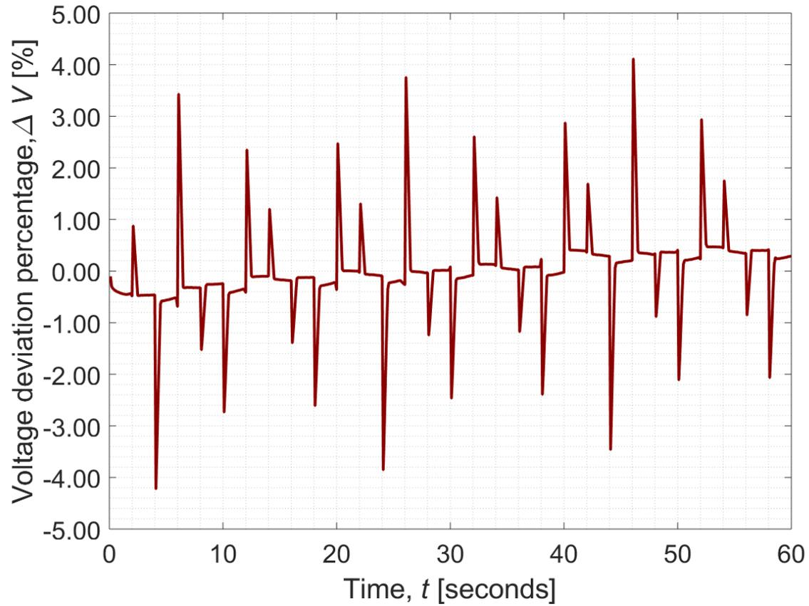
**Fig. S4** The voltage deviations in percentage for the dynamic pulse profiles, which has a maximum deviation in percentage of approximately 4%. The sharp peak in the deviations is caused by the immediate voltage jump when the current profile changes.
