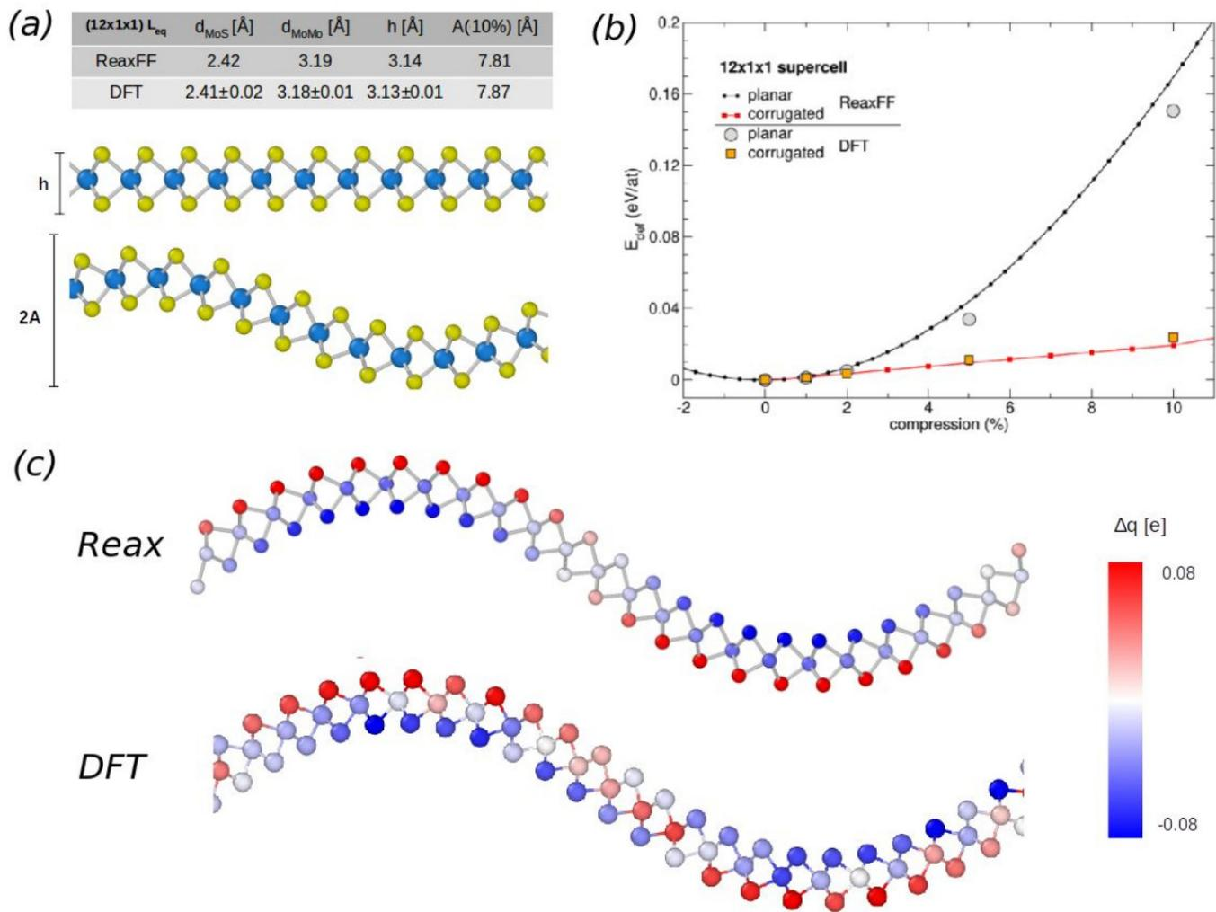
**Fig. 3** Comparison between the REAX classical potential and the DFT predictions for the the structural (a), energetics (b) and charge (c) properties of MoS<sub>2</sub> monolayers. In (b), we show the energy per atom in eV for keeping the system planar and allowing it to wrinkle. In (c), blue/red colors mean loss/gain of electrons.
