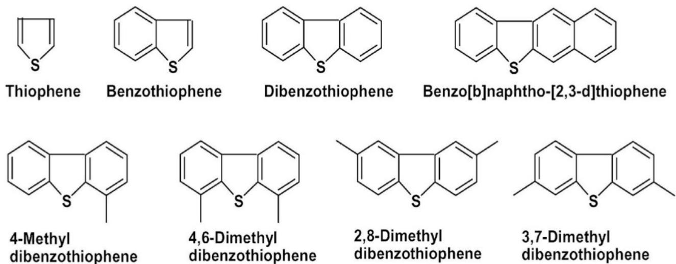
Fig. 1 Structures of the refractory sulphur compounds.
