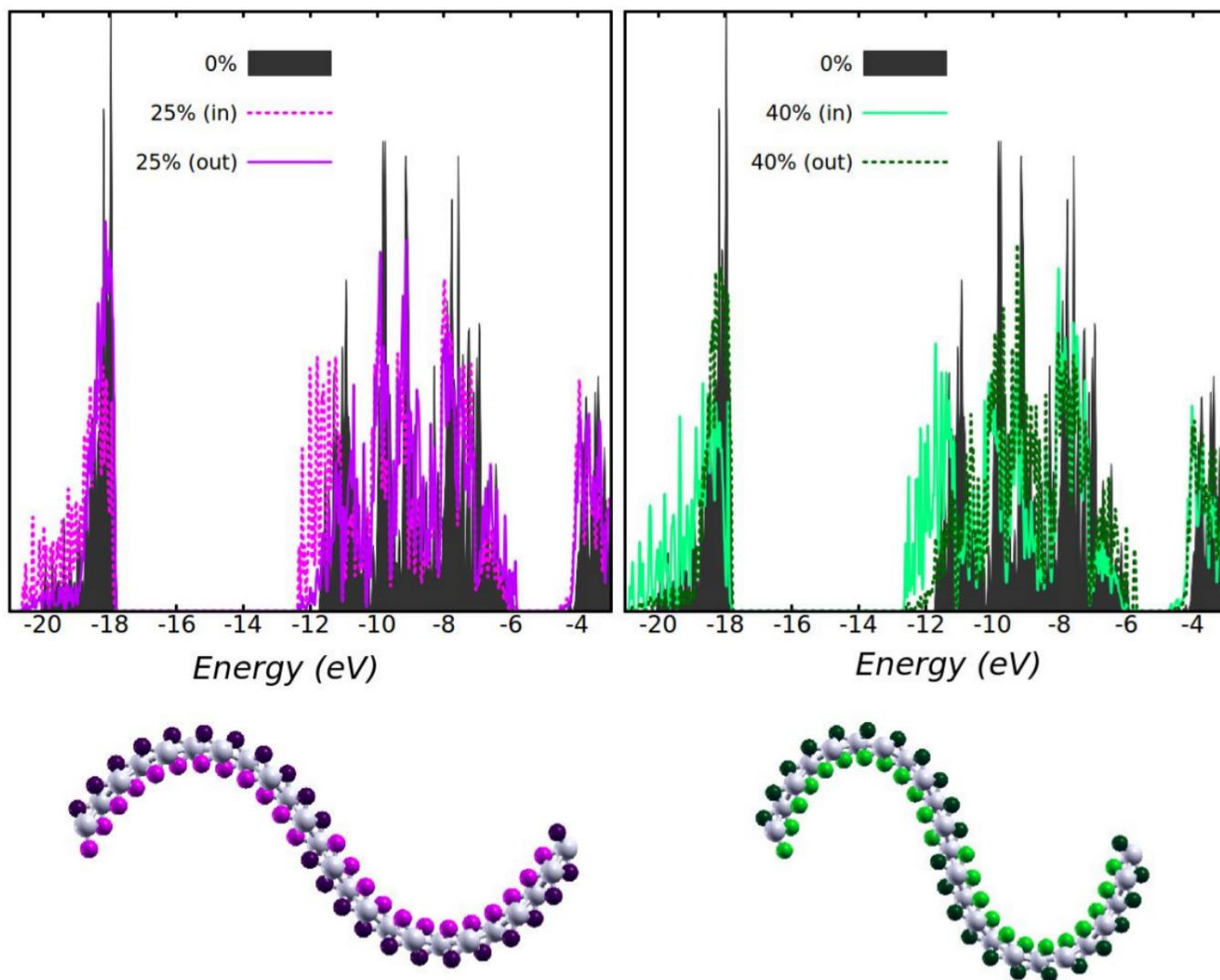
**Fig. 4** Complete Projected Density of States (PDOS) for the 1H MoS2 structure with C=0% (dark gray in both figures), with C=25% (left) and 40% (right). The contributions of the internal/ external S atoms is separated with a dashed/continuous line, respectively.
