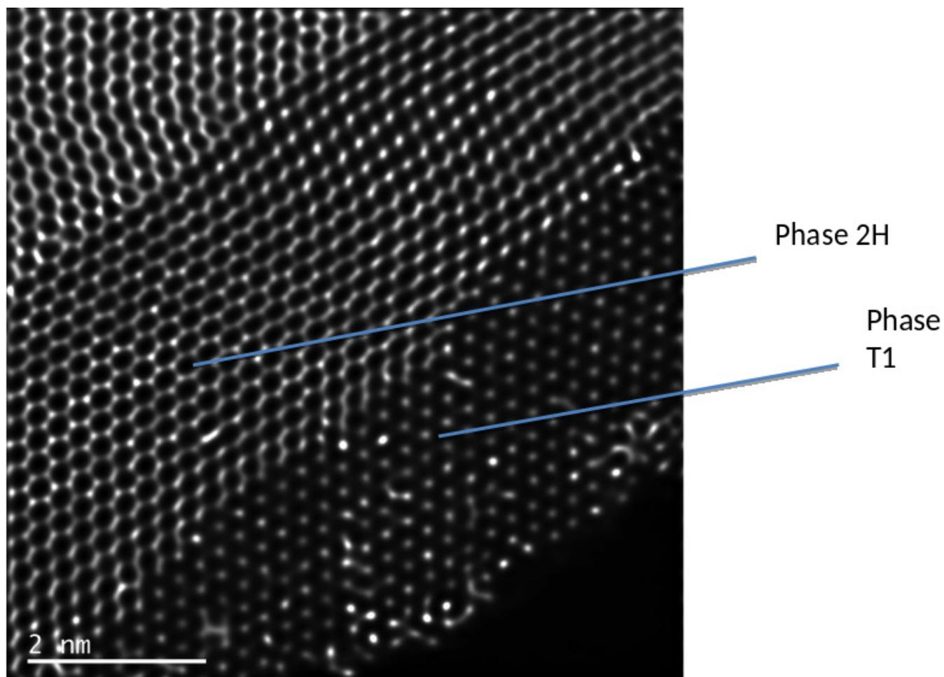
Fig. 2 Image showing the coexistence of the hexagonal and trigonal phases.
