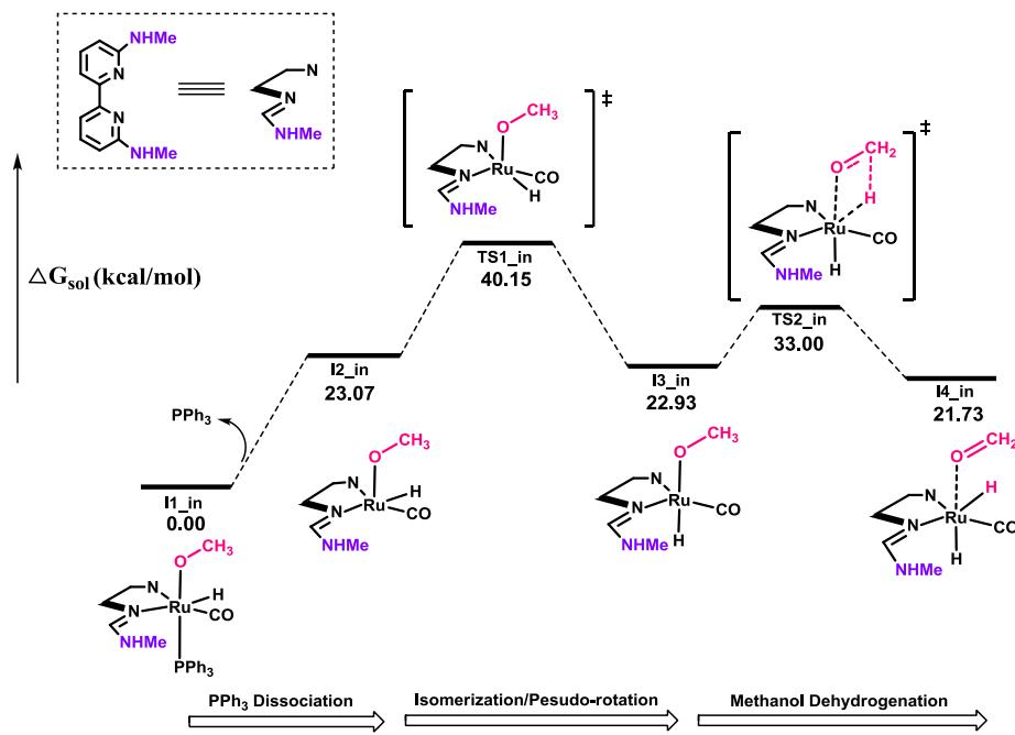
**Fig. S2:** Calculated Gibbs free energies (kcal/mol) for the methanol dehydrogenation following *inner-sphere* pathway (hybrid functional, M06-2X was used with the LANL2DZ basis set for Ru and the 6-31G\*\* basis set for non-metal elements).
