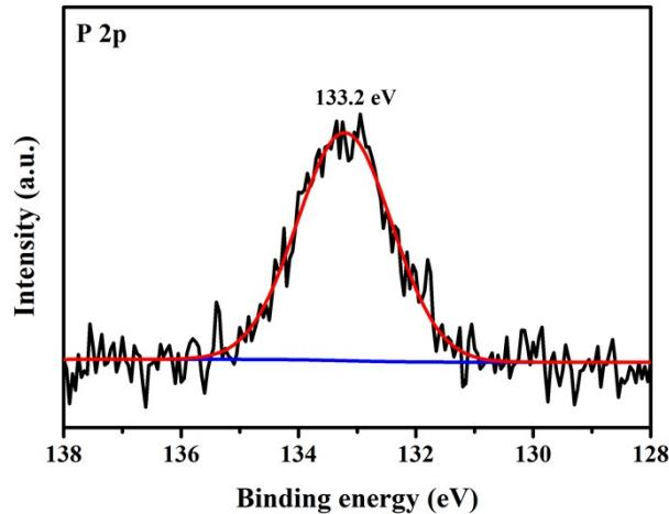
**Figure 14** XPS spectrum of P 2p for etched 0FeP/Ti- $\text{Fe}_2\text{O}_3$  using argon sputtering.
