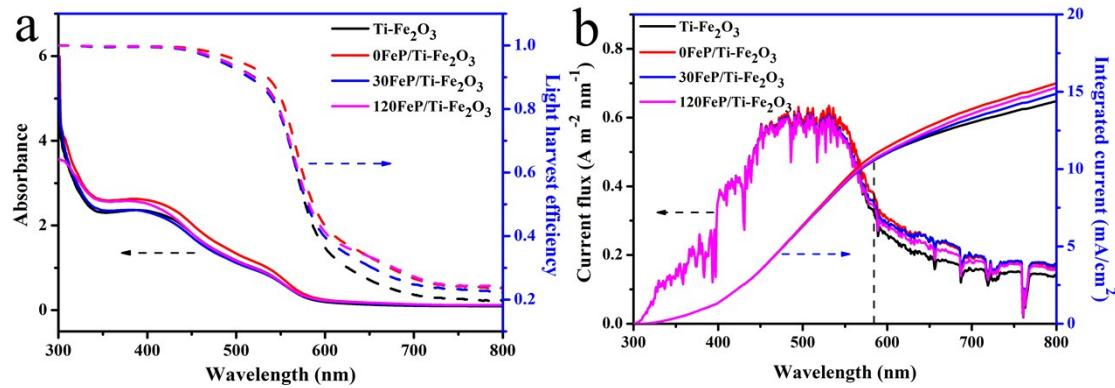
**Figure 13** (a) The absorption (solid line) and light harvest efficiency (dash line) of  $\text{Ti}-\text{Fe}_2\text{O}_3$  and  $\text{FeP}/\text{Ti}-\text{Fe}_2\text{O}_3$ . (b) The calculated current density flux and integrated current density ( $J_{\text{abs}}$ ) of  $\text{Ti}-\text{Fe}_2\text{O}_3$  and  $\text{FeP}/\text{Ti}-\text{Fe}_2\text{O}_3$ .
