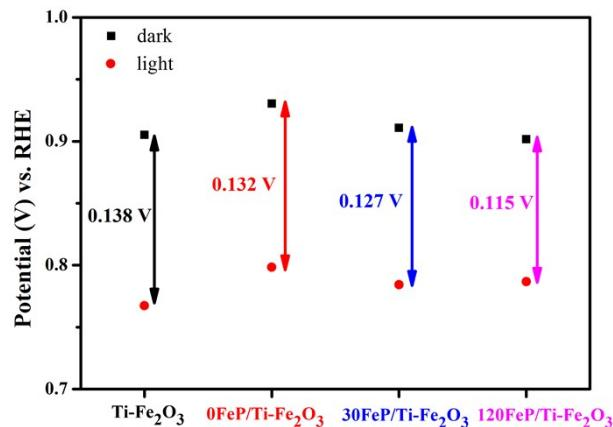
**Figure S11** Open-circuit potentials of Ti- $\text{Fe}_2\text{O}_3$  and FeP/Ti- $\text{Fe}_2\text{O}_3$  in dark and under AM 1.5 G illumination.
