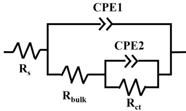
**Figure S15** The equivalent circuit model for fitting Nyquist plots of photoanodes.
