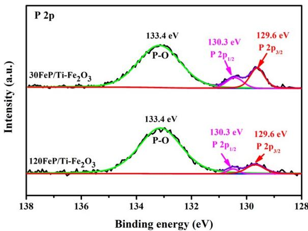
**Figure S5** XPS spectra of P 2p for 30FeP/Ti-Fe<sub>2</sub>O<sub>3</sub> and 120FeP/Ti-Fe<sub>2</sub>O<sub>3</sub>.
