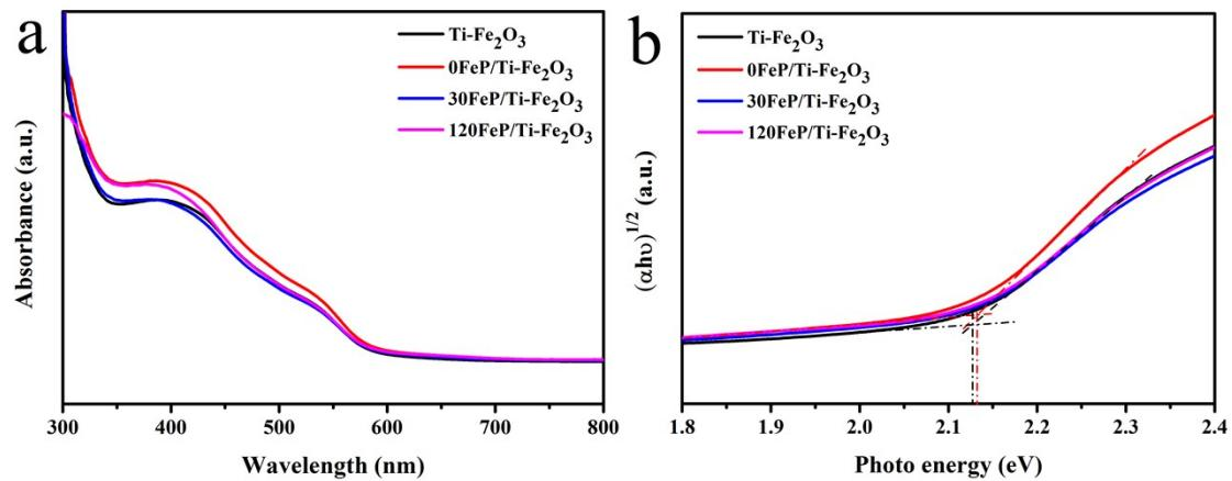
**Figure S10** UV-vis absorption spectra (a) and the corresponding Tauc's plots (b) of Ti- $\text{Fe}_2\text{O}_3$  and FeP/Ti- $\text{Fe}_2\text{O}_3$ .
