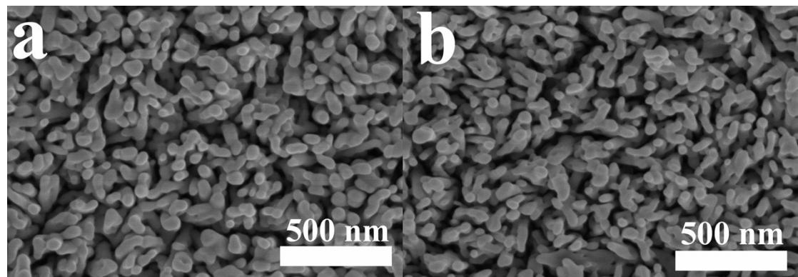
**Figure S2** Top-view FE-SEM images of Ti-Fe<sub>2</sub>O<sub>3</sub> (a) and 0FeP/Ti-Fe<sub>2</sub>O<sub>3</sub> (b).
