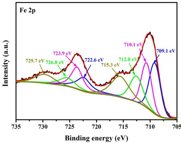
**Figure S4** XPS spectrum of Fe 2p for 0FeP/Ti-Fe<sub>2</sub>O<sub>3</sub>.
