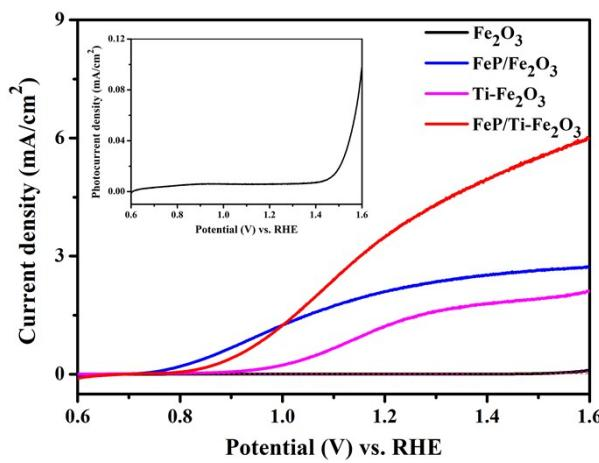
**Figure S6** Current-potential curves of Fe<sub>2</sub>O<sub>3</sub>, 0FeP/Fe<sub>2</sub>O<sub>3</sub>, Ti-Fe<sub>2</sub>O<sub>3</sub> and 0FeP/Ti-Fe<sub>2</sub>O<sub>3</sub> in dark and under AM 1.5 G illumination in 1 M KOH electrolyte solution. The inset shows the photocurrent density-potential curve of Fe<sub>2</sub>O<sub>3</sub>.
