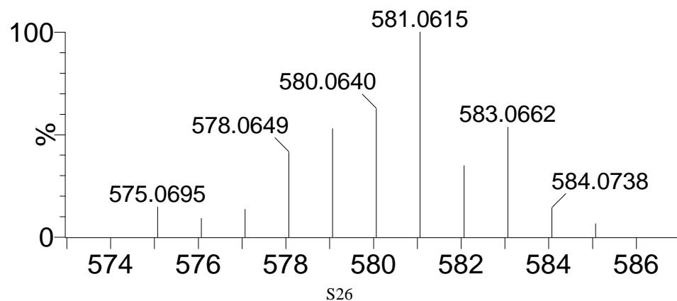
**Figure S16.** ESI-MS of the reaction of **2[PF<sub>6</sub>]** with thiophenol in THF
