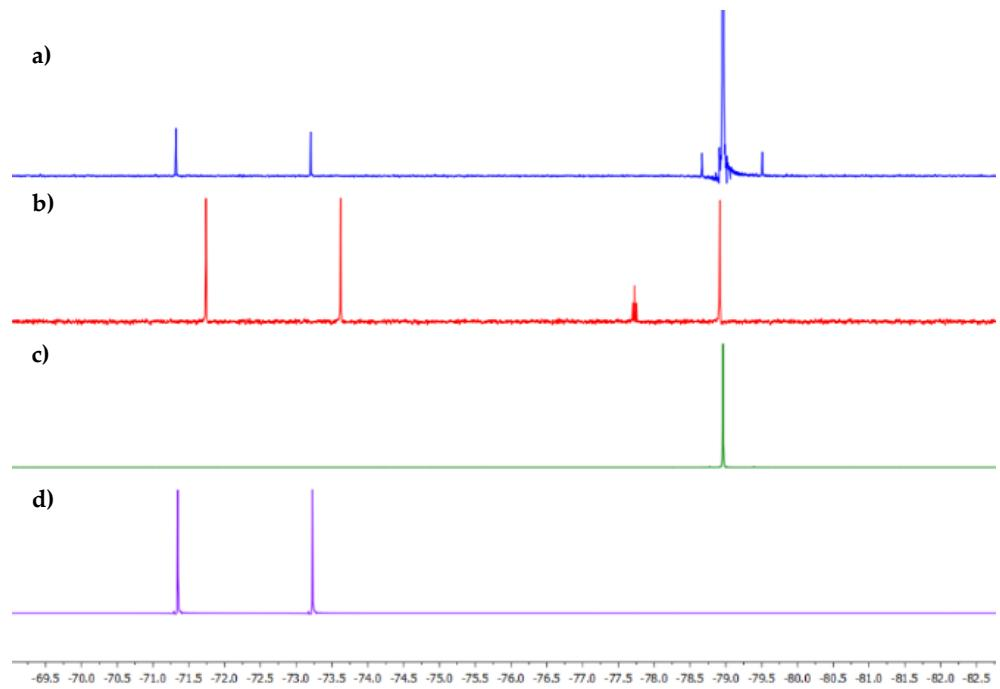
Figure S4: <sup>19</sup>F NMR comparisons between; a) *in*-[3-OH<sub>2</sub>]<sup>3+</sup> in D<sub>2</sub>O b) *in*-[3-OCOCF<sub>3</sub>]<sup>2+</sup> in acetone-d<sub>6</sub>. The <sup>19</sup>F NMR of free trifluoroacetate in D<sub>2</sub>O (c) and free potassium hexafluorophosphate in D<sub>2</sub>O (d) are shown for comparison
