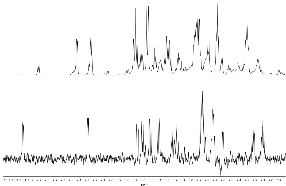
Figure S2: Stacked  $^1\text{H}$ -NMR spectra of impure **out-[3-Cl] $^{2+}$**  before light irradiation (above) and after light irradiation (below) performed in  $\text{MeOD}$ . Apodization for bottom spectra: Exponential: 1.60 Hz, Integral-to-noise effect : 5.129 s.
