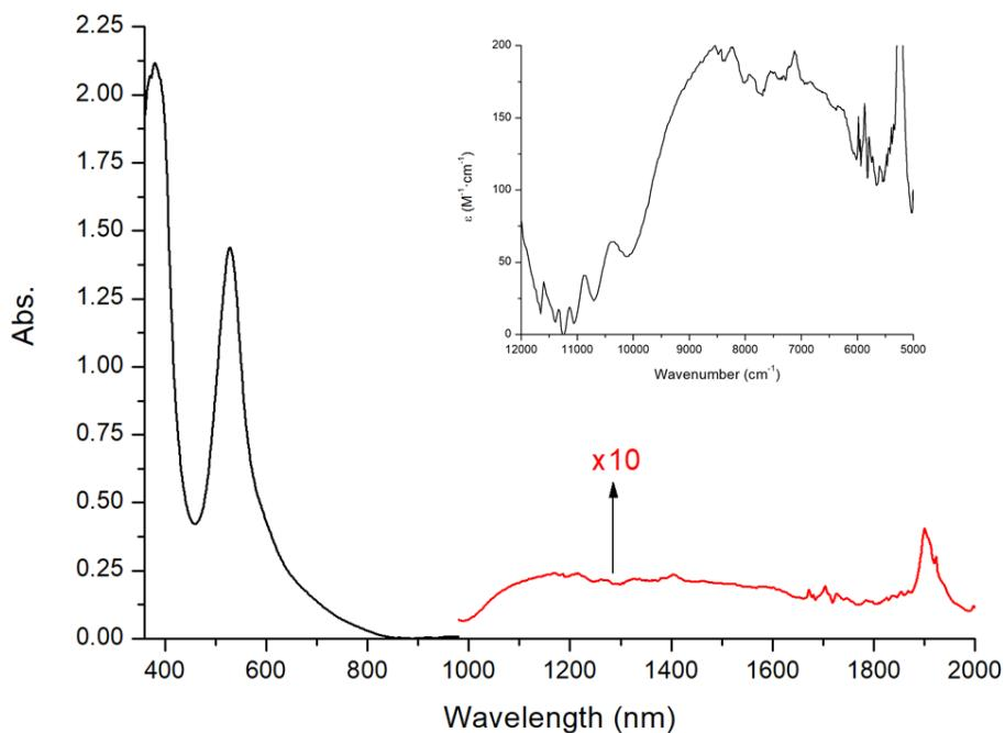
Figure S7: Vis-NIR spectra of *in*-[3-OH<sub>2</sub>]3<sup>+</sup> in CF<sub>3</sub>SO<sub>3</sub>H (pH = 1). Values between 1000-2000 nm multiplied by 10 for visibility. Inset: Vis-NIR spectra of *in*-[3-OH<sub>2</sub>]3<sup>+</sup> in CF<sub>3</sub>SO<sub>3</sub>H (pH = 1) at a concentration of 2.0 mM.  $\nu_{\text{max}}$  (cm<sup>-1</sup>) = 8422.
