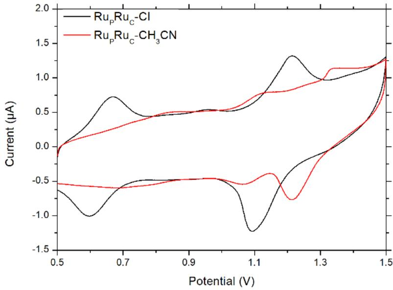
Figure S8: Cyclic voltammograms of *in-[3-Cl]<sup>2+</sup>* and *in-[3-CH<sub>3</sub>CN]<sup>3+</sup>* in a deoxygenated solution of CH<sub>2</sub>Cl<sub>2</sub> with supporting electrolyte TBAF (0.1 M) scan rate of 0.01 Vs<sup>-1</sup>.
