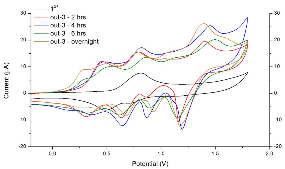
Figure S1: Cyclic voltammograms of **out-[3-Cl] $^{2+}$**  showing degradation under ambient light over time periods of 2 hours in  $\text{CH}_2\text{Cl}_2$ , scan rate 0.1 V/s.  $\text{out-}[1]^{2+}$  shown for comparison.
