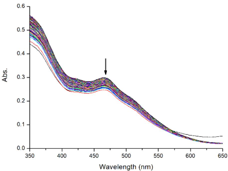
Figure S6: UV-Vis absorbance spectra over time for an aqueous solution of *in*-[3-OH]3<sup>+</sup> at pH = 12 under air. The arrow indicates the decrease in absorption at the MLCT as a result of precipitation of the complex.
