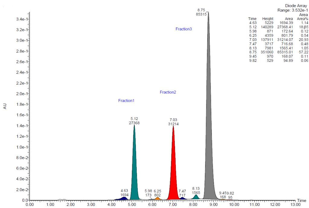
Figure S19: Full HPLC chromatogram of dyad mixture after reaction (iv). Fractions assigned by mass spec. Fraction 1 - Ru(tpy)<sub>2</sub> derivative, Fraction 2 - **2<sup>2+</sup>**, Fraction 3 - *in-[3-OOCF<sub>3</sub>]<sup>2+</sup>*.
