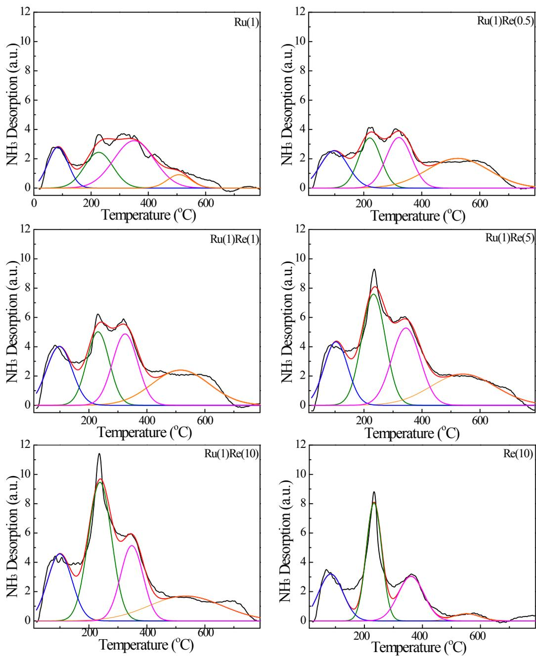
**Fig. S5** NH<sub>3</sub>-TPD profiles of TiO<sub>2</sub>-supported catalysts. Each TPD desorption profile is divided into four regions depending on desorption temperatures.
