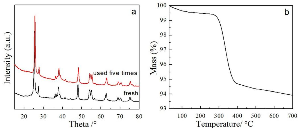
**Fig. S1** (a) XRD patterns of fresh and used catalysts and (b) TGA of Ru(1)Re(10)/TiO<sub>2</sub> used five times.
