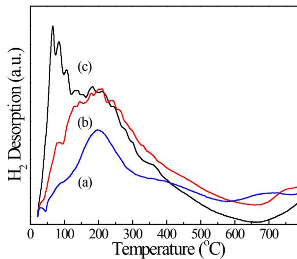
**Fig. S4** H<sub>2</sub>-TPD results of (a) Ru(1)/TiO<sub>2</sub>, (b) Re(10)/TiO<sub>2</sub> and (c) Ru(1)Re(10)/TiO<sub>2</sub> catalysts.
