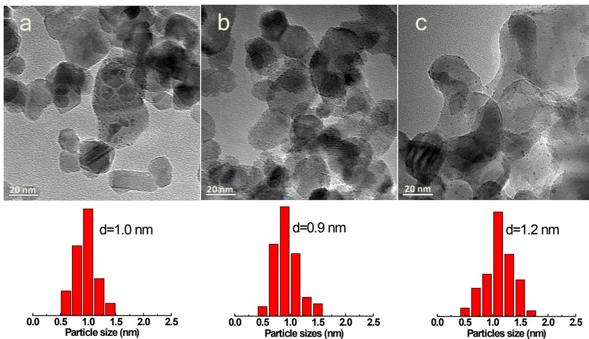
**Fig. S2** TEM images and histograms of metal particle size distribution of (a) Ru(1)/TiO<sub>2</sub>, (b) Re(10)/TiO<sub>2</sub> and (c) Ru(1)Re(10)/TiO<sub>2</sub> catalysts reduced at 300 °C.
