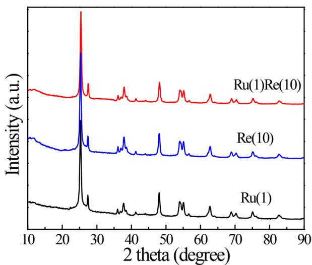
**Fig. S3** XRD patterns of Ru(1)/TiO<sub>2</sub>, Re(10)/TiO<sub>2</sub> and Ru(1)Re(10)/TiO<sub>2</sub> catalysts reduced at 300 °C.
