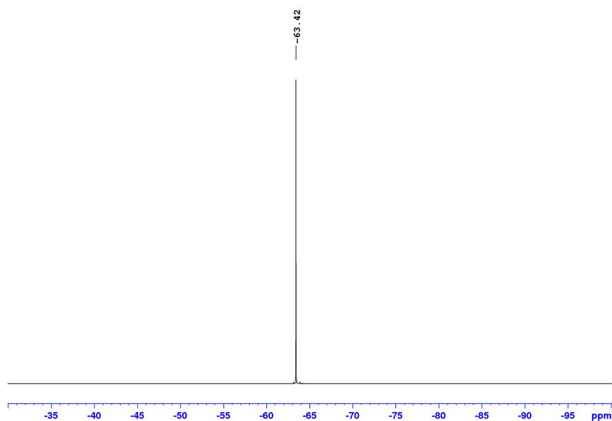
**Figure S9:**  $^{19}\text{F}\{^1\text{H}\}$  NMR (376.5 MHz,  $\text{THF-}d_8$ , 298 K) spectrum of anhydrous  $\text{Na}[\text{BAr}^{\text{F}}_4]$  (**2**) as a representative example of anhydrous alkali metal  $\text{BAr}^{\text{F}}_4$  salt (anhydrous  $\text{Li}[\text{BAr}^{\text{F}}_4]$  and anhydrous  $\text{K}[\text{BAr}^{\text{F}}_4]$  gave identical spectra).
