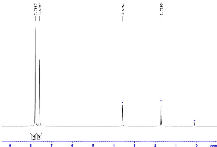
**Figure S6:**  $^1\text{H}$  NMR (400.2 MHz,  $\text{THF-}d_8$ , 298 K) spectrum of anhydrous  $\text{Na}[\text{BAr}^{\text{F}}_4]$  (**2**). Residual protio solvent resonances and traces of silicone grease from  $\text{THF-}d_8$  are marked with \* and + respectively.
