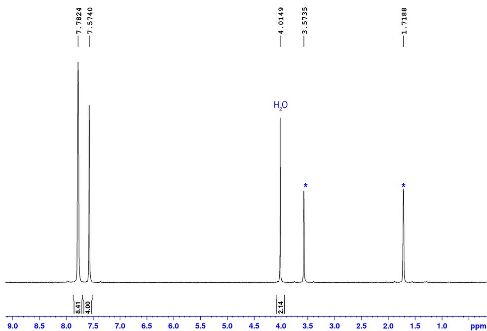
**Figure S4:**  $^1\text{H}$  NMR (400.2 MHz,  $\text{THF-}d_8$ , 298 K) spectrum of isolated crystals of  $[\text{Li}(\text{H}_2\text{O})][\text{BAr}^{\text{F}}_4]$  (4).
