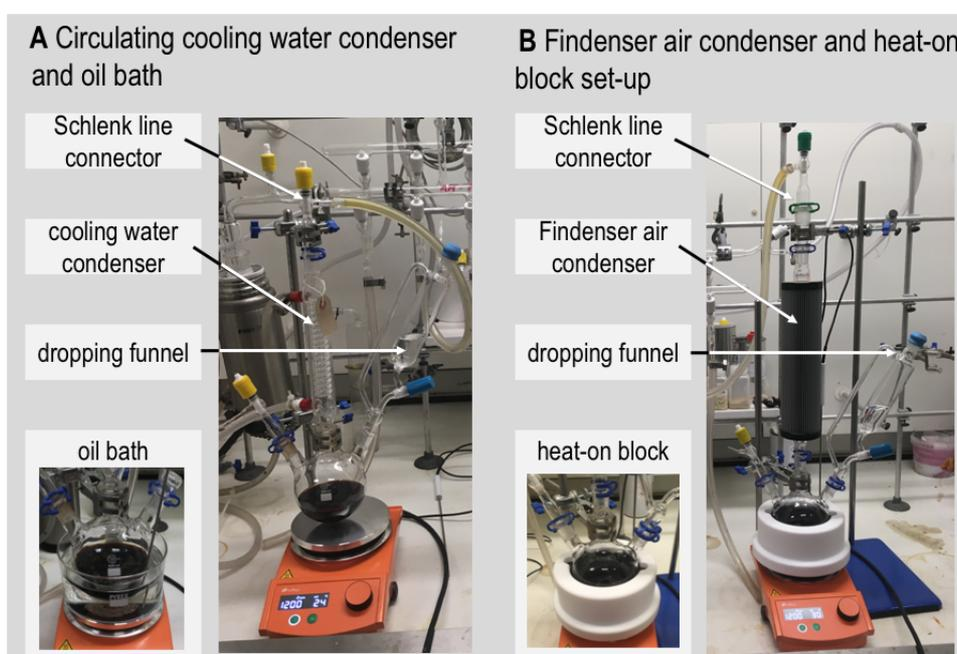
**Figure S1:** Comparing the two systems: (A) Silicone oil bath and circulating water cooling condenser set-up and (B) heat-on block and Findenser air condenser set-up.
