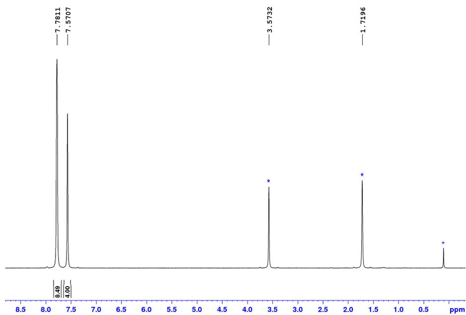
**Figure S10:**  $^1\text{H}$  NMR (400.2 MHz,  $\text{THF-}d_8$ , 298 K) spectrum of anhydrous  $\text{K}[\text{BAr}^{\text{F}}_4]$  (**3**). Residual protio solvent resonances and traces of silicone grease from  $\text{THF-}d_8$  are marked with \* and + respectively.
