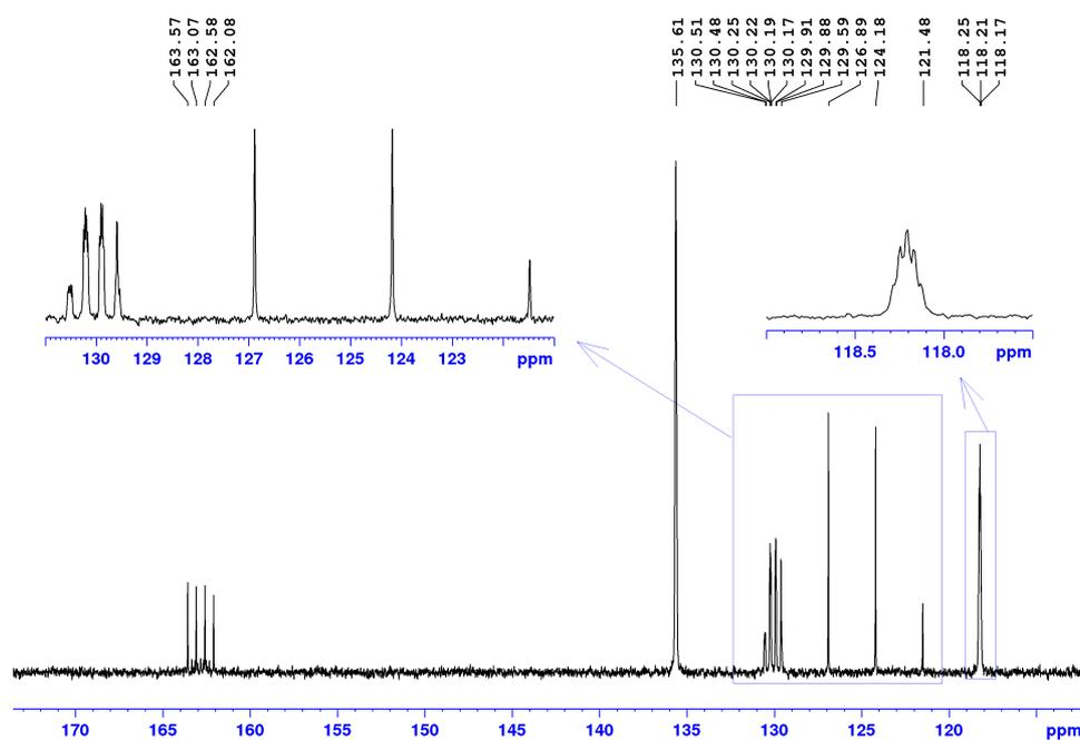
**Figure S8:**  $^{13}\text{C}\{^1\text{H}\}$  NMR (100.6 MHz,  $\text{THF-}d_8$ , 298 K) spectrum of anhydrous  $\text{Na}[\text{BAr}^{\text{F}}_4]$  (**2**) as a representative example of anhydrous alkali metal  $\text{BAr}^{\text{F}}_4$  salt (anhydrous  $\text{Li}[\text{BAr}^{\text{F}}_4]$  and anhydrous  $\text{K}[\text{BAr}^{\text{F}}_4]$  gave identical spectra).
