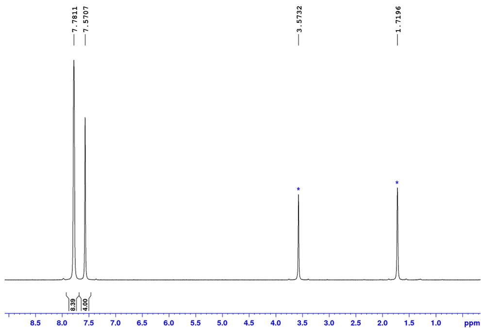
**Figure S2:** <sup>1</sup>H NMR (400.2 MHz, THF-*d*<sub>8</sub>, 298 K) spectrum of anhydrous Li[BAr<sup>F</sup><sub>4</sub>] (**1**). Residual protio solvent resonances are marked with \*.
