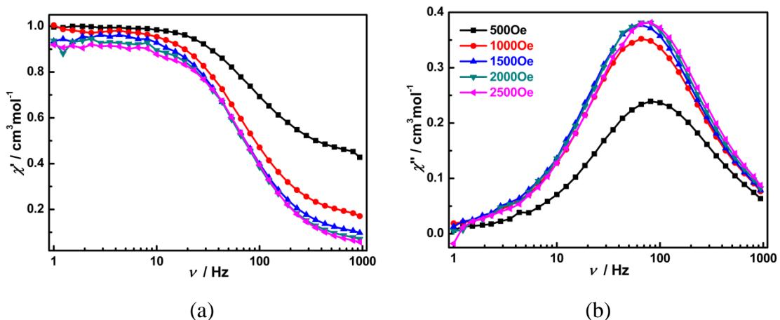
**Fig. S7** Frequency dependence of in-phase (a) and out-of-phase (b) ac susceptibility data under different dc fields at 2 K for **2**.
