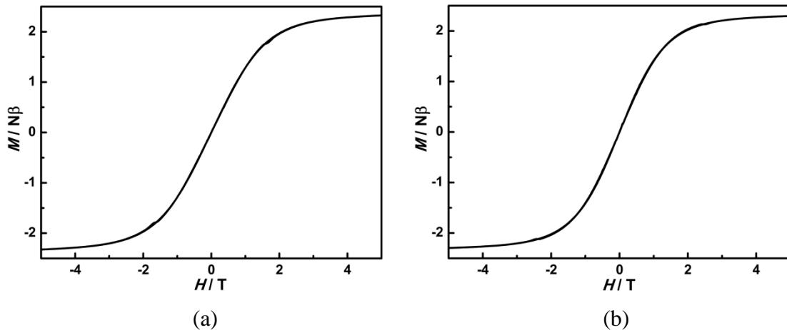
**Fig. S8** Field dependence of the magnetization at 2 K for **1** (a) and **2** (b).
