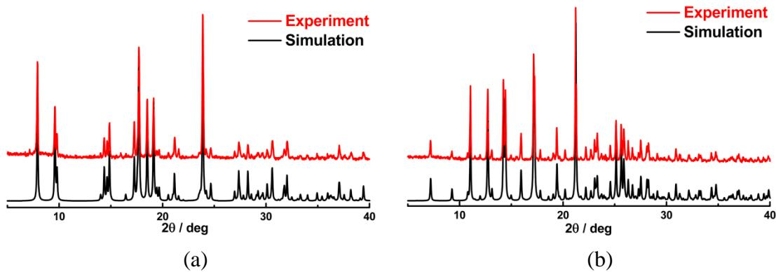
**Fig. S2** Experimental and simulated PXRD patterns for complexes **1** (a) and **2** (b).
