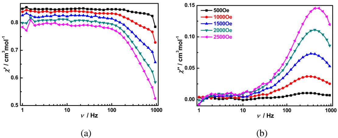
**Fig. S6** Frequency dependence of in-phase (a) and out-of-phase (b) ac susceptibility data under different dc fields at 2 K for **1**.
