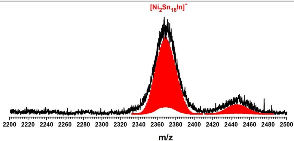
**Figure S14.** Measured (top) and simulated (bottom) spectrum of the fragment  $[\text{Ni}_2\text{Sn}_{18}\text{In}]^-$  and  $[\text{K}_2\text{Ni}_2\text{Sn}_{18}\text{In}]^-$ .
