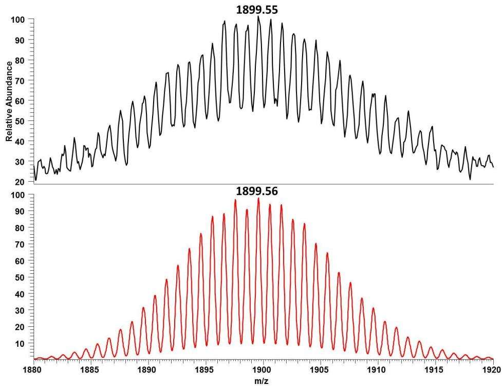
**Figure S13.** Measured (top) and simulated (bottom) spectrum of the fragment  $[\text{K}(2,2,2\text{-crypt})\text{Sn}_9]^-$ .
