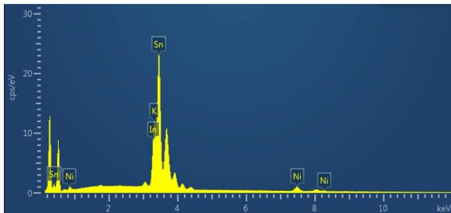
Figure S20. EDX analysis of  $[\text{K}(2,2,2\text{-crypt})]_5[\text{Ni}@\text{Sn}_9]\text{In}[\text{Ni}@\text{Sn}_9]$ .
