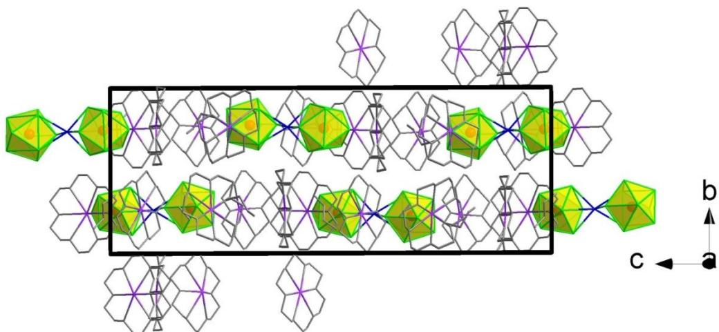
**Figure S5.** Packing of cations and anions in  $[K(18\text{-crown-6})]_5[Ni@Sn_9]In[Ni@Sn_9]$  viewed down the  $a$  axes. Solvent molecules and hydrogen atoms are omitted for clarity.
