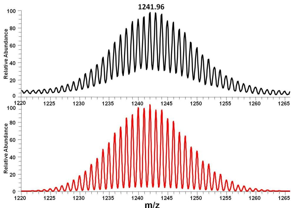
**Figure S11.** Measured (top) and simulated (bottom) spectrum of the fragment  $[\text{NiSn}_9\text{In}]^-$ .
