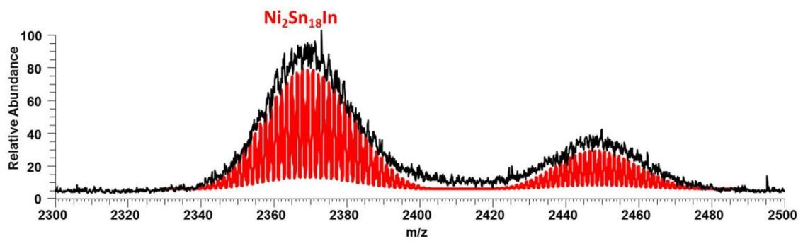
**Figure S19.** Measured (top) and simulated (bottom) spectrum of the fragment  $[\text{Ni}_2\text{Sn}_{18}\text{In}]^-$  and  $[\text{K}_2\text{Ni}_2\text{Sn}_{18}\text{In}]^-$ .
