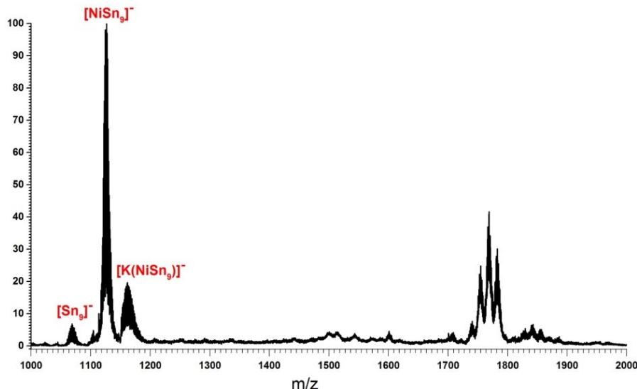
**Figure S1.** The full electrospray mass spectrum ( $m/z$ : 1000–2000) in negative ion mode of the DMF solution of the phase “ $K_4Ni_3Sn_9$ ”
