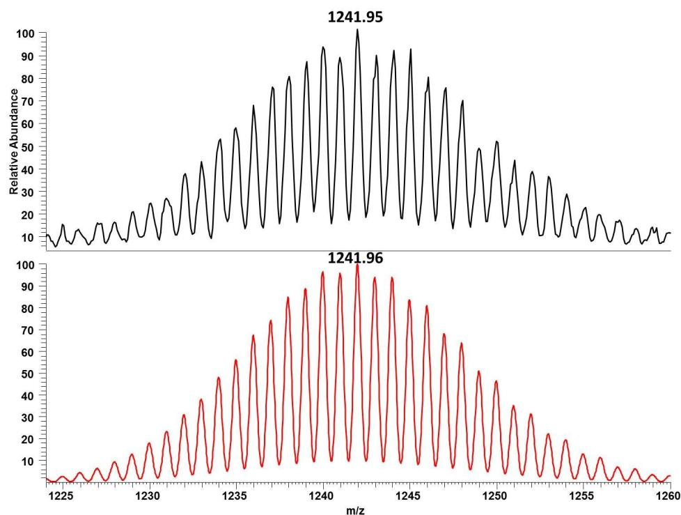
**Figure S16.** Measured (top) and simulated (bottom) spectrum of the fragment  $[\text{NiSn}_9\text{In}]^-$ .
