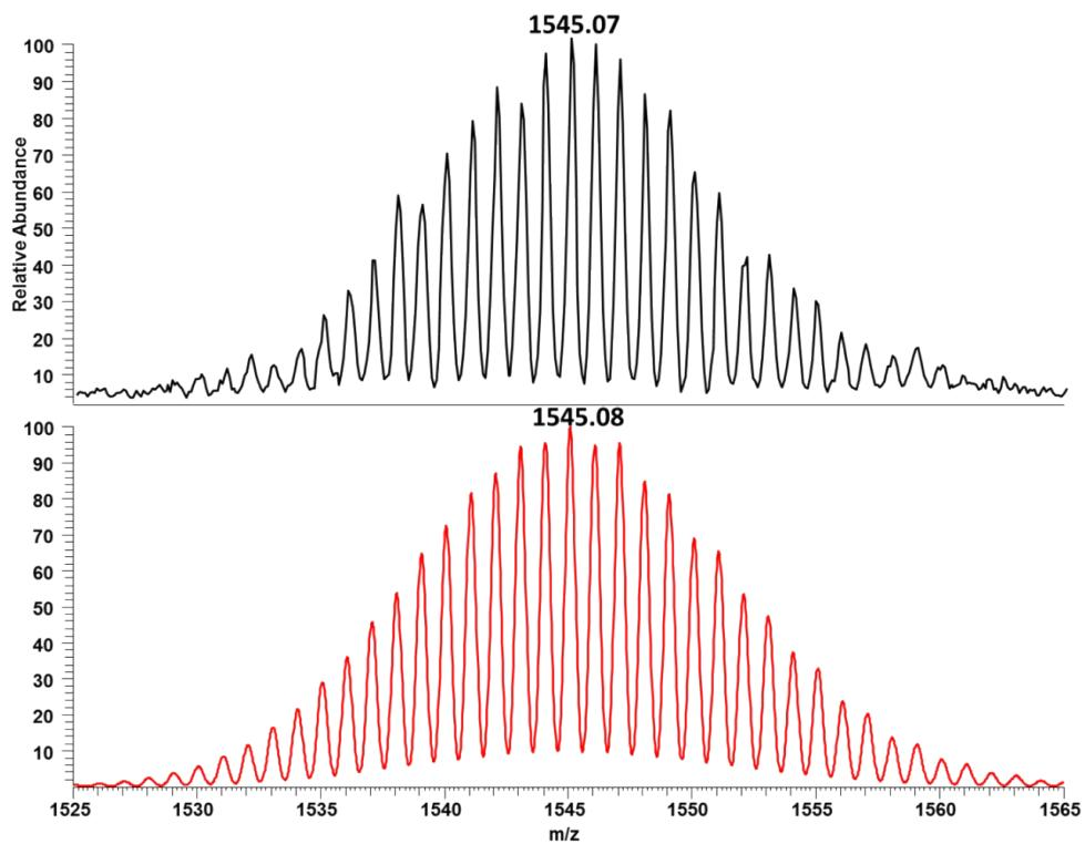
**Figure S18.** Measured (top) and simulated (bottom) spectrum of the fragment  $[\text{K}(18\text{-C-6})\text{NiSn}_9\text{In}]^-$ .
