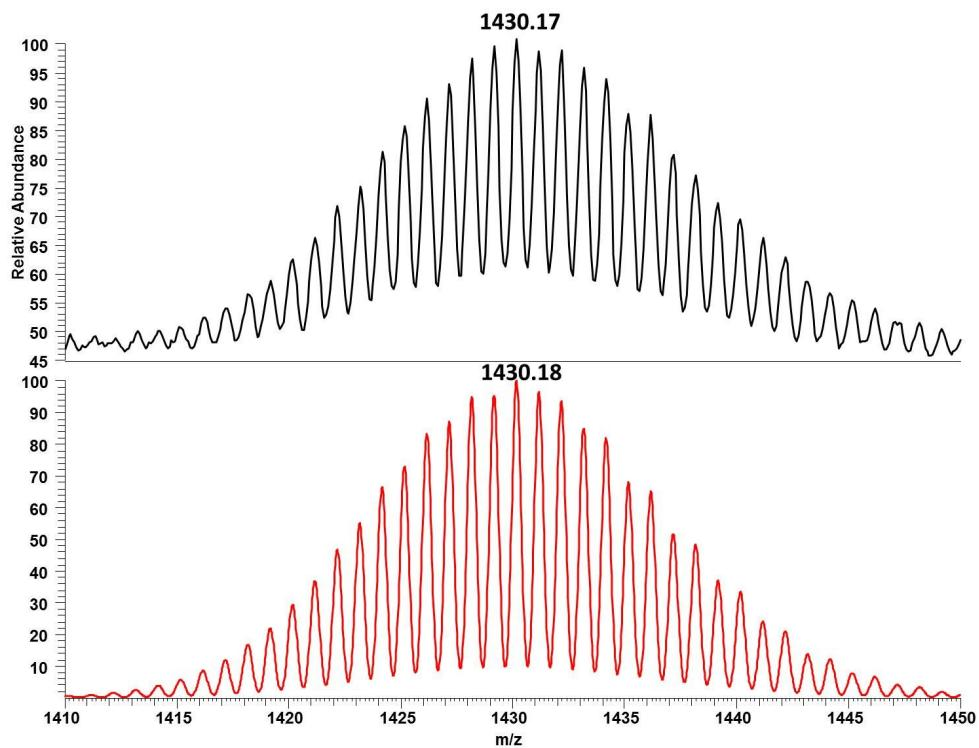
**Figure S17.** Measured (top) and simulated (bottom) spectrum of the fragment  $[\text{K}(18\text{-C-6})\text{NiSn}_9]^-$ .
