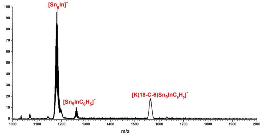
**Figure S2.** The full electrospray mass spectrum ( $m/z$ : 1000-2000) in negative ion mode of the en solution of the mixture of “ $K_4Sn_9$ ” and  $In(C_6H_5)_3$ .
