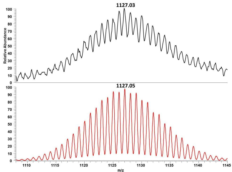
**Figure S9.** Measured (top) and simulated (bottom) spectrum of the fragment  $[NiSn_9]^-$ .
