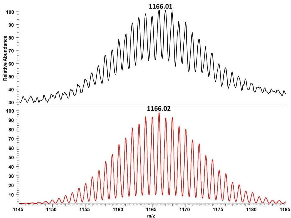
**Figure S10.** Measured (top) and simulated (bottom) spectrum of the fragment  $[\text{KNiSn}_9]^-$ .
