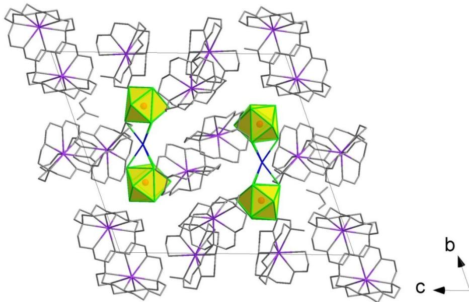
**Figure S4.** Packing of cations and anions in  $[K(2,2,2\text{-crypt})]_5[Ni@Sn_9]In[Ni@Sn_9]$  viewed down the  $a$  axes. Solvent molecules and hydrogen atoms are omitted for clarity.
