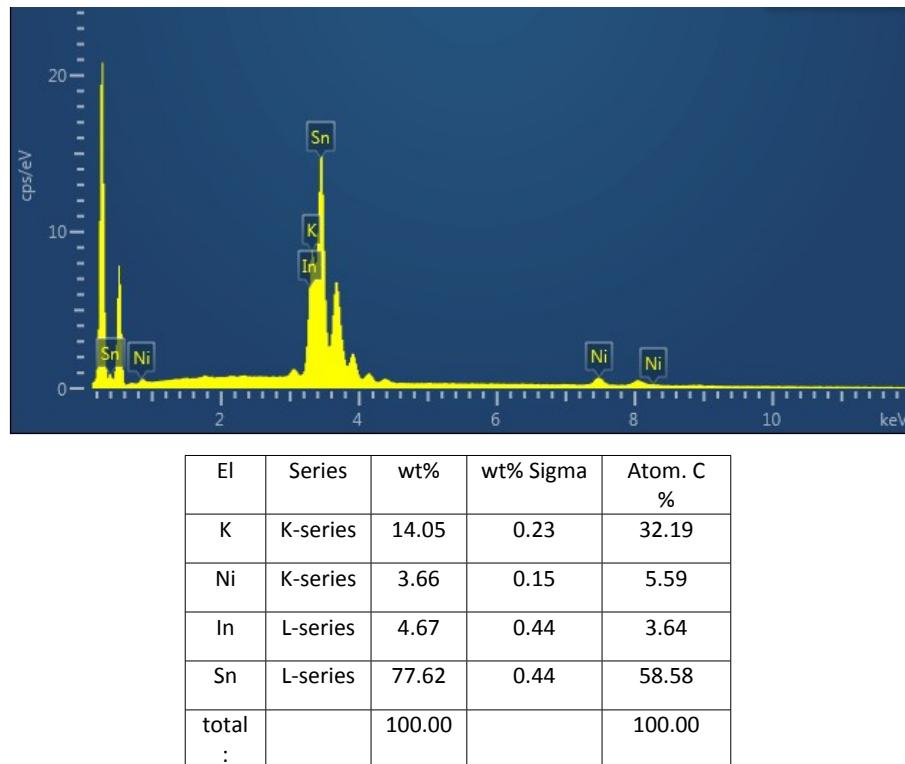
Figure S21. EDX analysis of  $[\text{K}(18\text{-crown-6})]_5[\text{Ni}@\text{Sn}_9]\text{In}[\text{Ni}@\text{Sn}_9]$ .
