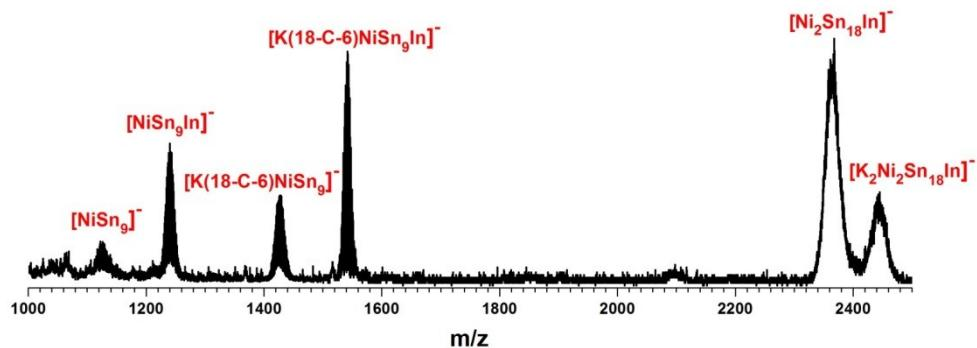
**Figure S15.** Overview ESI mass spectrum in negative ion mode of a freshly dissolved crystalline sample of  $[\text{K}(18\text{-crown-6})]_5[\text{Ni}@\text{Sn}_9]\text{In}[\text{Ni}@\text{Sn}_9]$  in en.
