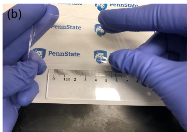
Fig. S4. (a) Cross-sectional SEM image of XL-VK-2 film with a thickness of 10.8 \mu\text{m} . Photographs of XL-VL-2 films (b) before and (c) after soaking in a high-temperature insulation fluid at 150^\circ\text{C} for 24 h. The crosslinked films maintain the flatness, transparency and flexibility, exhibiting excellent thermal stability.
