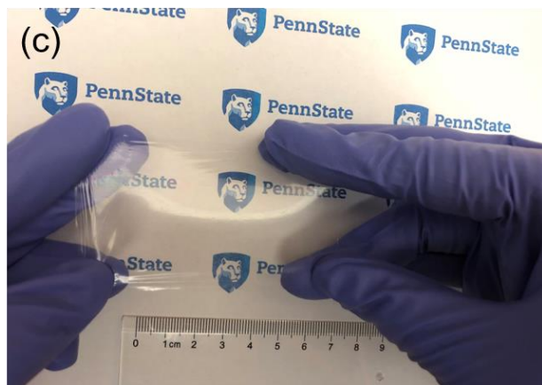
Fig. S4. (a) Cross-sectional SEM image of XL-VK-2 film with a thickness of 10.8 \mu\text{m} . Photographs of XL-VL-2 films (b) before and (c) after soaking in a high-temperature insulation fluid at 150^\circ\text{C} for 24 h. The crosslinked films maintain the flatness, transparency and flexibility, exhibiting excellent thermal stability.
