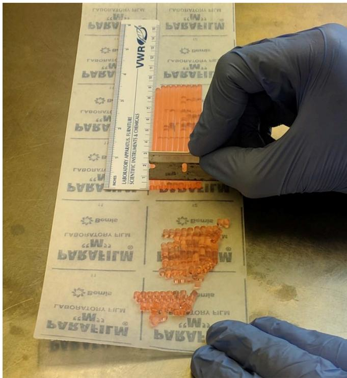
Figure S5. Manual cutting of gellan gum strands into 2mm right cylinders for experimental use. For better visualization GG pre-gel solution was dyed orange.
