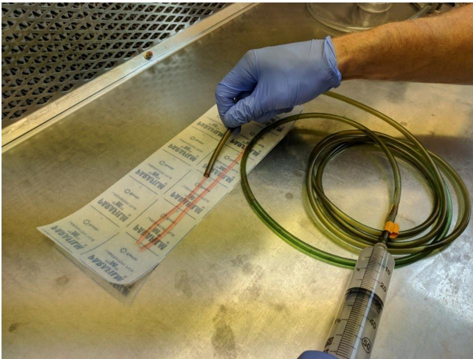
Figure S4. Extrusion of solidified gellan gum cylindrical sections from rubber tubing onto Parafilm. For better visualization GG pre-gel solution was dyed orange.
