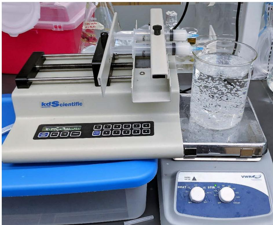
Figure S1. Calcium-alginate macrobead formation by extrusion into crosslinking solution.
