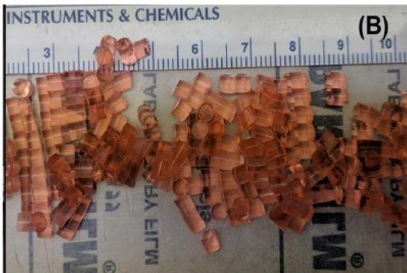
Figure S6. Gellan gum beads with ATCC 21198 and TBOS co-encapsulated 2 mm in diameter by 2 to 3 mm in length.
