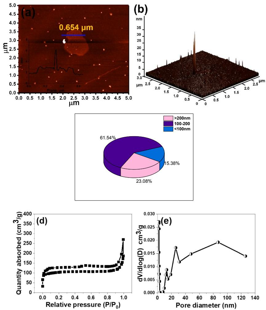
Figure S1 (a) AFM images of MGA (insets show the height profiles), (b) AFM 3D surface images of the MGA, (c) particle size distribution in the MGA, (d) N<sub>2</sub> adsorption and desorption isotherms of MGA, (e) pore size distribution of MGA.
