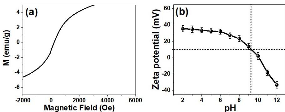
Figure S2 (a) Low field region of magnetization curves, (b) Zeta potential of MGA.
