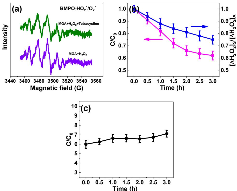
Figure S3 (a) BMPO spin-trapping EPR spectra for HO<sub>2</sub>•/O<sub>2</sub>• of MGA, (b) The decomposition and utilization efficiency of H<sub>2</sub>O<sub>2</sub> during tetracycline degradation by MGA, (c) pH changes of the solution during tetracycline degradation by MGA.
